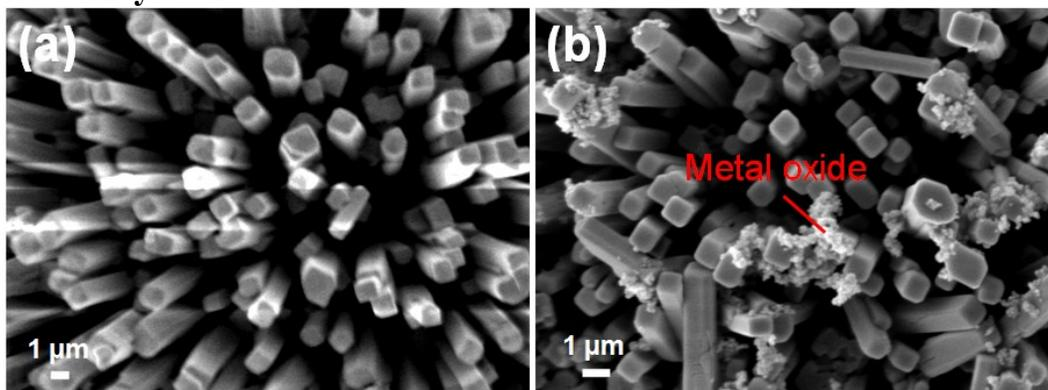
**Fig. S1:** The FESEM micrographs of (a)  $\text{CuBi}_2\text{O}_4$  and (b)  $\text{CuBi}_2\text{O}_4$  composite with auxiliary Co but without EG. The metal oxide could be visibly seen anchored on the surface of the  $\text{CuBi}_2\text{O}_4$  nanorods.
