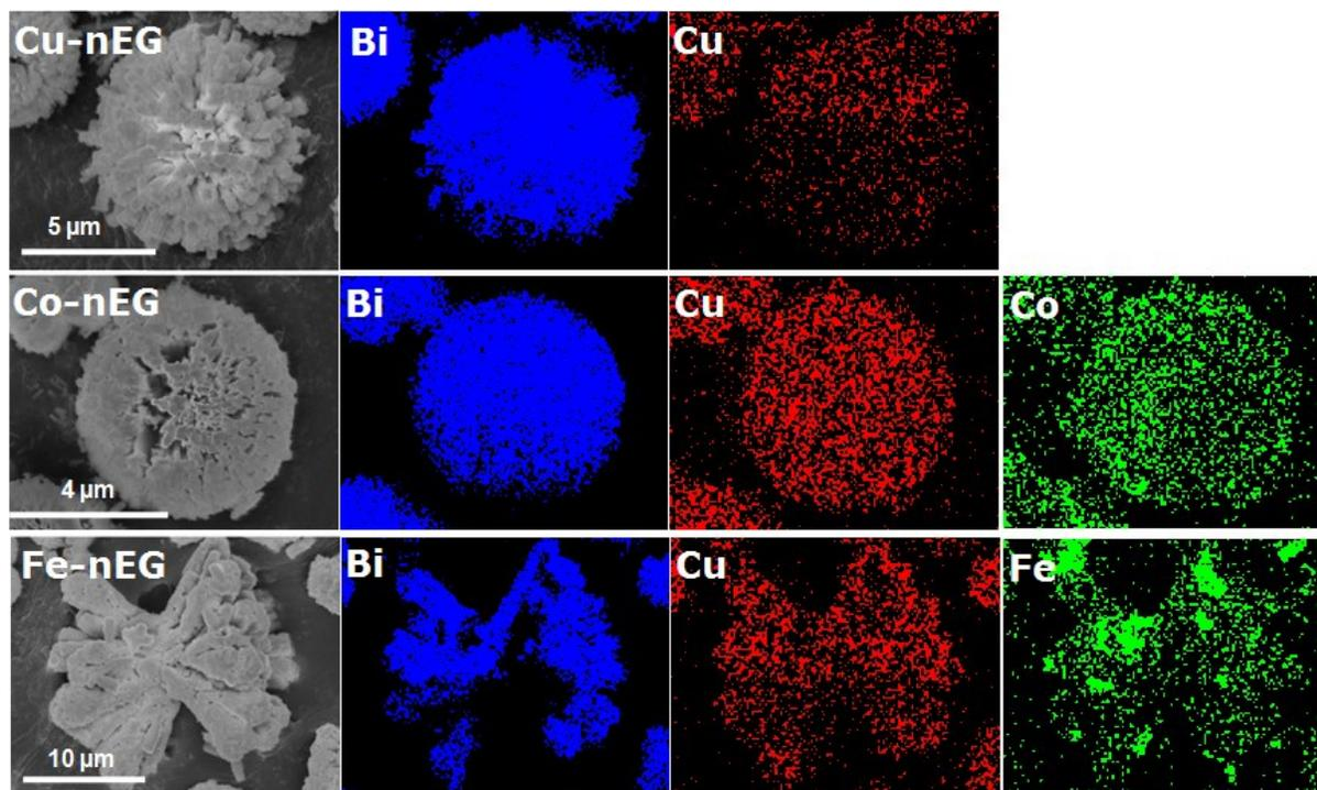
**Fig. S3:** Elemental mapping of CuO-CuB, CoO-CuB and FeO-CuB indicating relatively homogeneous distribution of the elements. This also provides clear evidence that the Co and Fe are present in the crystal system.
