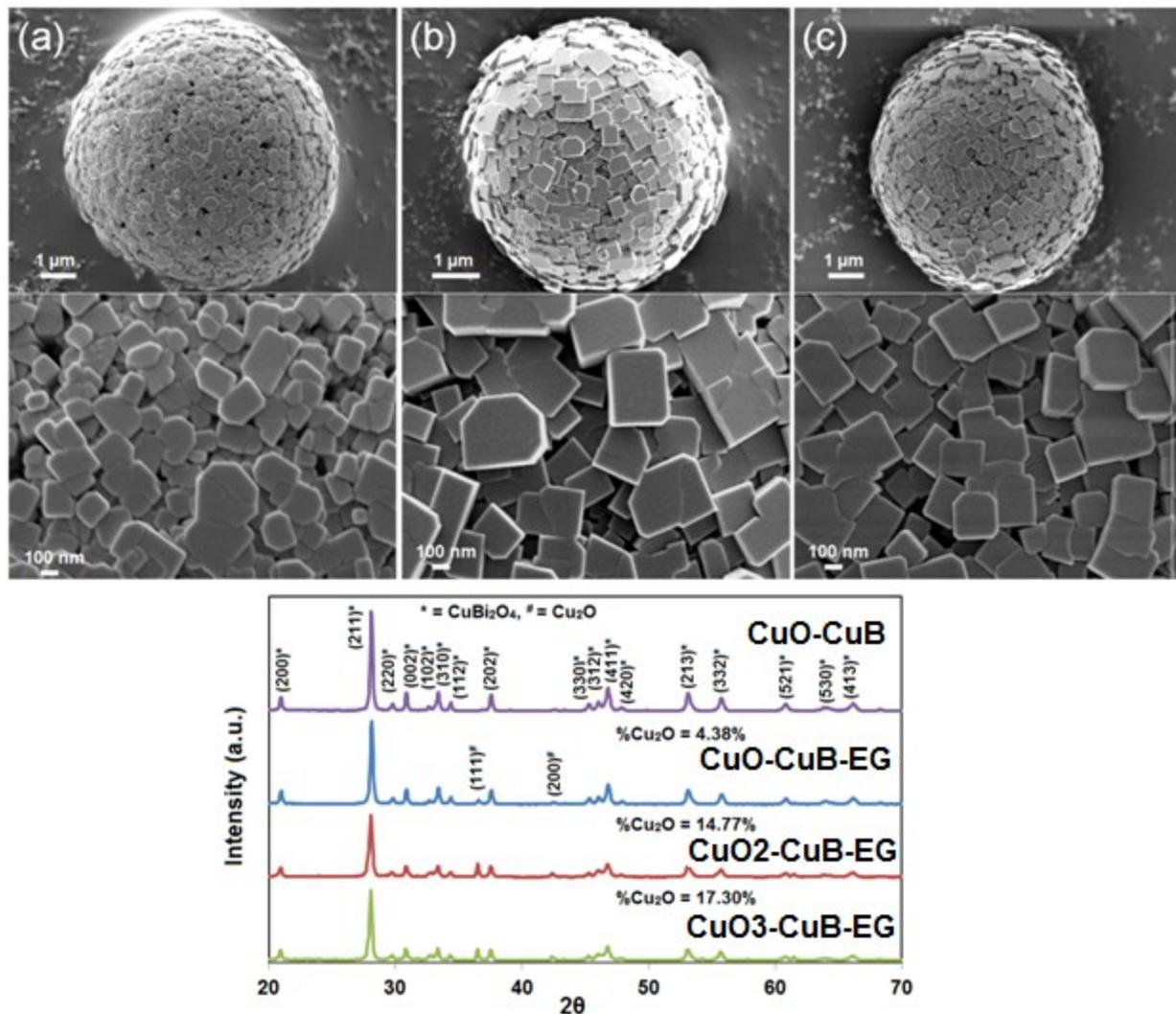
**Fig. S4:** The FESEM micrographs (single microsphere and surface) and % Cu<sub>2</sub>O content determined using the rietveld refinement method. (a) CuO-CuB-EG, (b) CuO<sub>2</sub>-CuB-EG, and (c) CuO<sub>3</sub>-CuB-EG. The morphologies of the CuBi<sub>2</sub>O<sub>4</sub> composites are similar. The close-up micrograph of the surface reveals Cu<sub>2</sub>O cubic surface.
