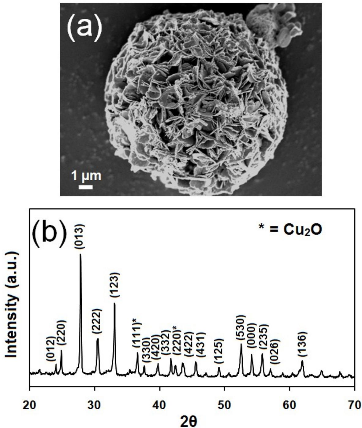
**Fig. S5:** The FESEM micrograph (a) and XRD pattern (b) of FeO-CuB-EG. The FESEM micrograph indicates that the FeO-CuB-EG has a pollen-grain-like morphology. The XRD pattern can be indexed to and Cu<sub>2</sub>O.
