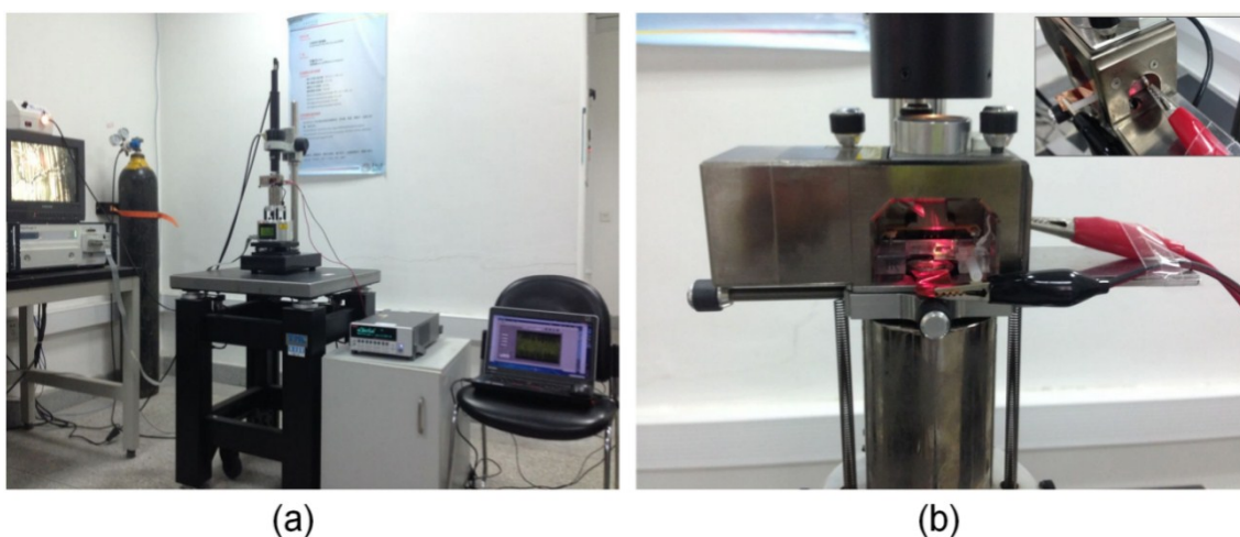
Figure S8: (a) Enhanced setup used for measuring the I-t curves. (b) Detail of the connections between the sourcemeter and the AFM tip and sample plate.
