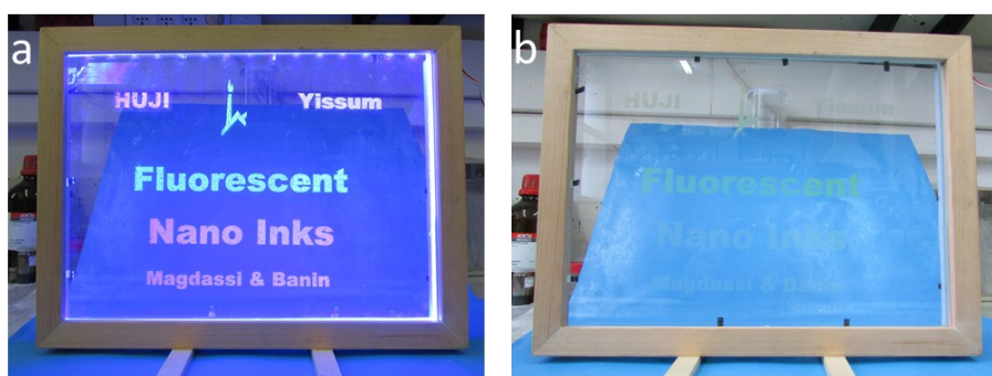
Figure S2: Green and red emitting CdSe/CdS seeded NRs inks printed on Perspex with (a) and without (b) exposure to blue LED.
