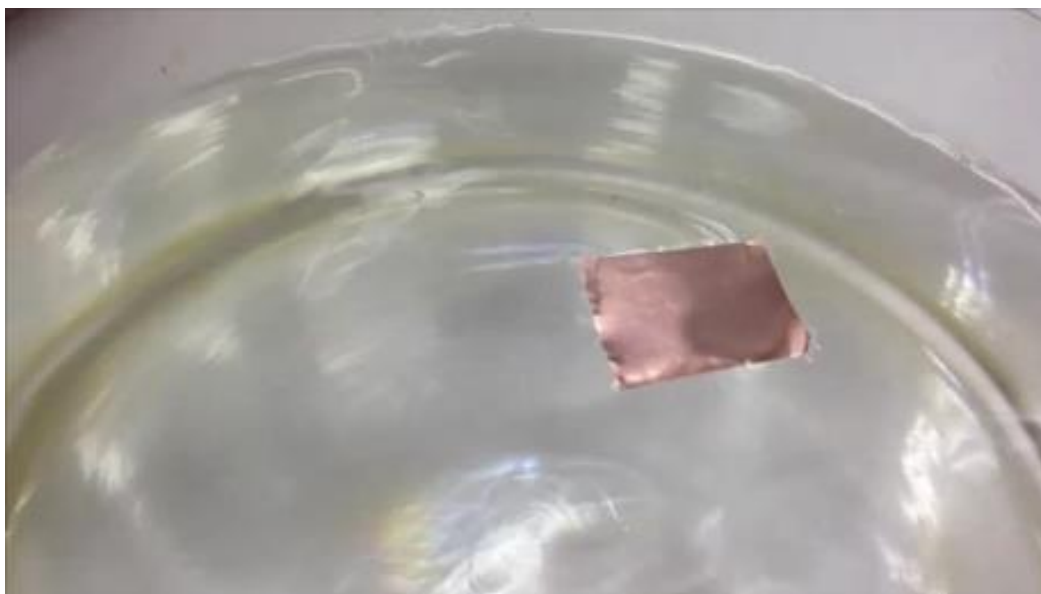
Video V1: Video of the lifting of the graphene film from the Cu foil catalyst.
