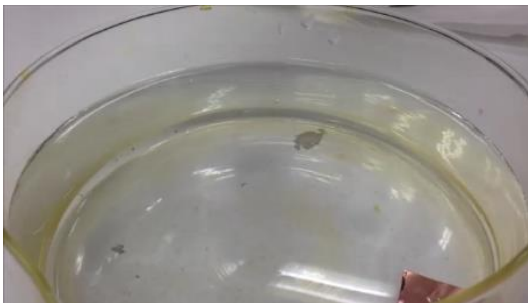
Video V2: Video of the transfer of the GF lifted off the Cu foil onto a piece of plastic.
