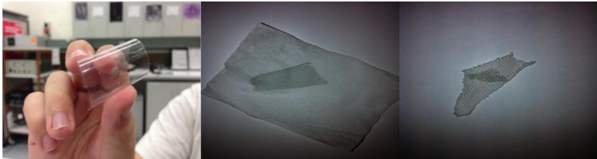
Figure S6: Graphene transferred to a) plastic, b) paper and c) cotton.
