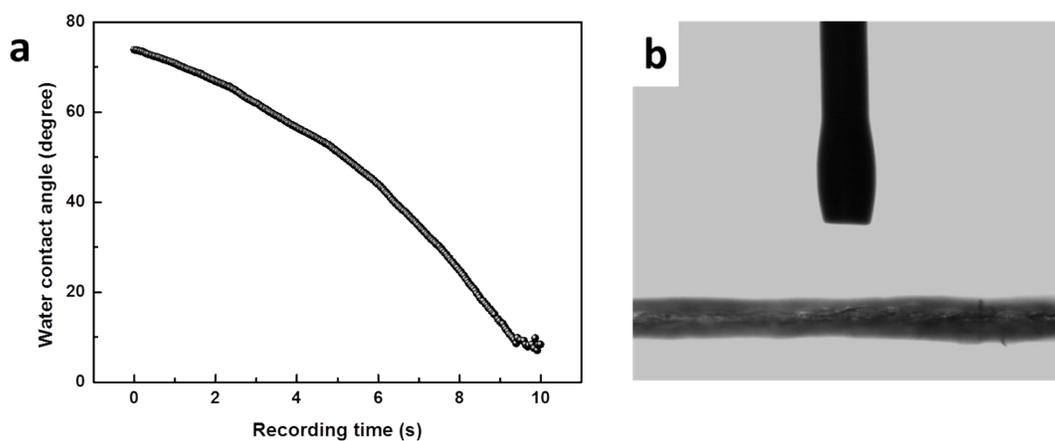
**Figure S3.** (a) Water CA recordings of pristine fabric. (b) Oil CA image on pristine fabric. Water droplet spread out on the pristine fabric in 10 s. The final water CA is less than 10°, demonstrating the superhydrophilicity of pristine fabric. Cyclohexane droplet spread out on the pristine fabric immediately, showing the superoleophilicity of pristine fabric.
