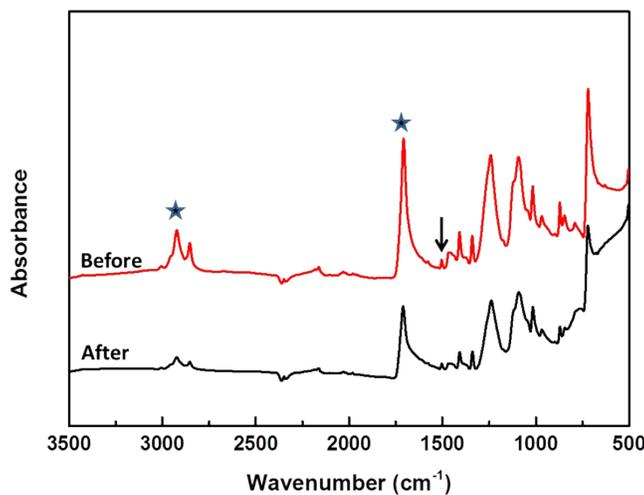
**Figure S6.** FTIR spectra of OA/PBZT10 before and after heating.
