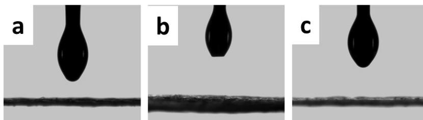
**Figure S5.** Oil CA images of (a) OA/PBZT10, exposed OA/PBZT10 (b) before and (c) after heat treatment at 140 °C for 1h. The surfaces are all superoleophilic with an oil droplet spreading out on the surfaces.
