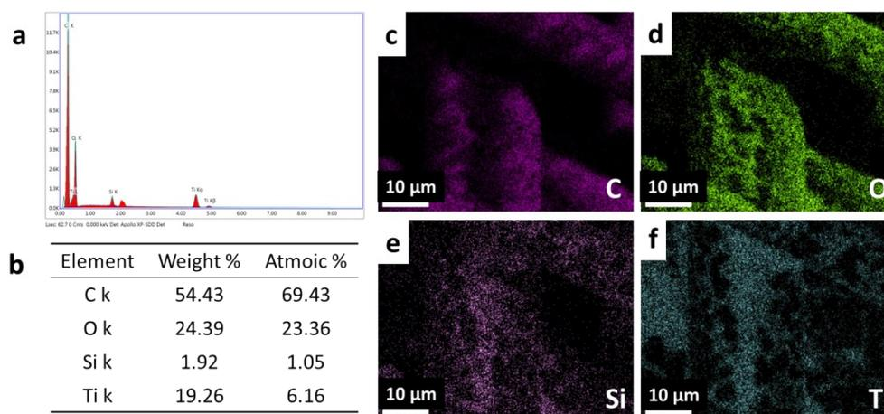
**Figure S1.** (a) EDS spectrum and (b) element distribution on PBZT10. Mapping images of (c) C, (d) O, (e) Si and (f) Ti of PBZT10 surface.
