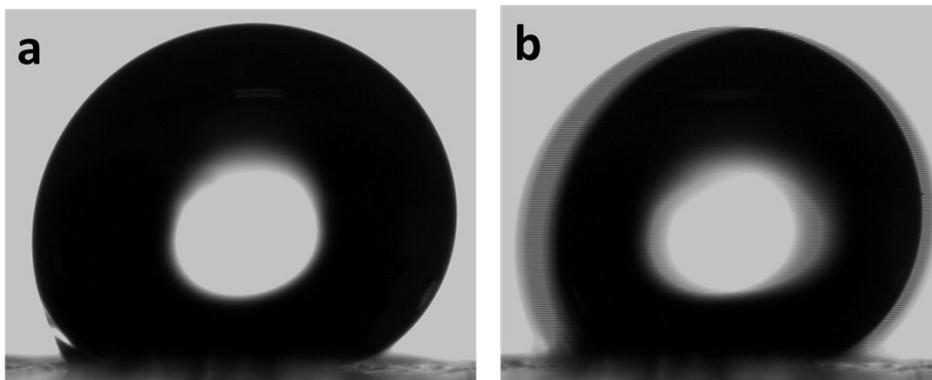
**Figure S7.** Images of water droplet on PBZT10 before and during rolling when the base was tilted for 25°. (water droplet, 10  $\mu\text{L}$ )
