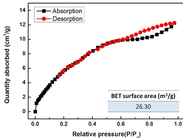
**Figure S4.** N<sub>2</sub> adsorption-desorption isotherm and BET surface area of PBZT10.
