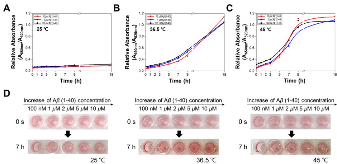
**Fig. S4.** Plots for colorimetric responses showing the different protein aggregation kinetics according to the incubation temperature. (A) 25 °C, (B) 36.5 °C, (C) 45 °C, and (D) Corresponding color changes observed after 7 hours.
