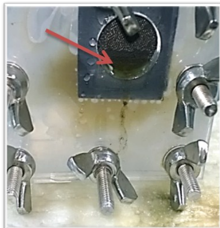
Fig. S9 A photograph of a ZnAB after long time discharging showing electrolyte leakage problem. The electrolyte turned to brown color indicating the degradation of carbon.
