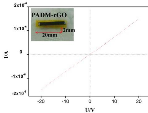
Figure S4. I-V test of PADM-rGO hybrid scaffold.
