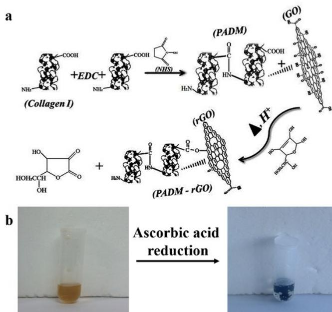
Figure S2. (a) Schematic of prepare PADM-rGO hybrid scaffold, (b) the state of GO after reduced by ascorbic acid.
