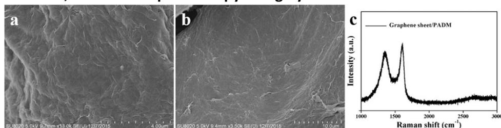
Figure S3. SEM images of ascorbic acid reduced GO (a), the channel surface of PADM-rGO hybrid
