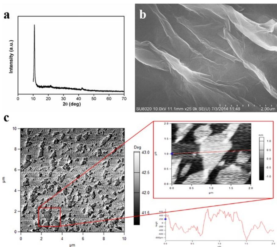
**Figure S1.** X-Ray Diffraction (XRD) pattern of GO powder (a), SEM image of GO (b), Atomic Force Microscopy (AFM) of GO nanosheets (c).
