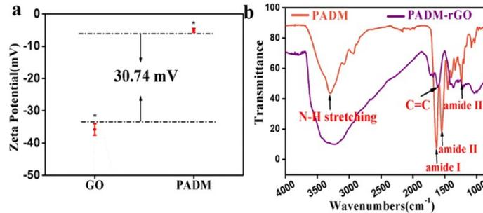
Figure S5. Zeta potential of GO solution and PADM suspension (a), FT-IR spectrum of PADM and PADM-rGO (b). (\*p ≤ 0.05, \*\*p ≤ 0.01, n=3)
