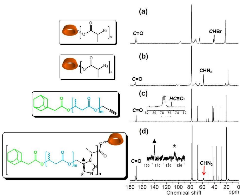
**Figure S2.** <sup>13</sup>C NMR spectra of (a) CD-s-Br, (b) CD-s-N<sub>3</sub>, (c) PHB, and (d) CD-s-PHB-Ada in CDCl<sub>3</sub>.
