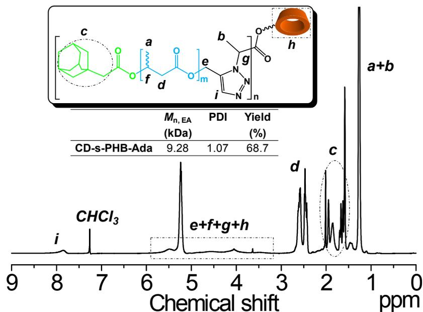
**Figure S3.**  $^1\text{H}$  NMR spectrum of CD-s-PHB-Ada in  $\text{CDCl}_3$  with corresponding peak assignments. Triazole linking group and adamantyl end group can be clearly seen in the spectrum.
