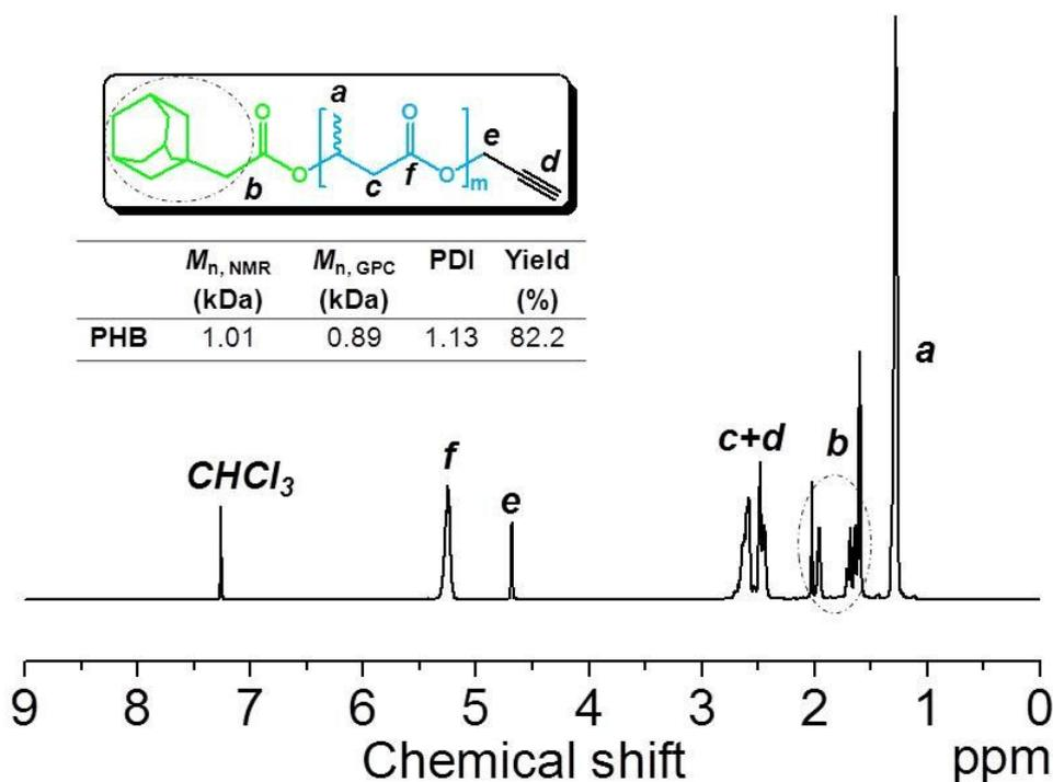
**Figure S1.**  $^1\text{H}$  NMR spectrum of heterofunctionalized PHB in  $\text{CDCl}_3$  with corresponding peak assignments. Alkynyl and adamantyl end groups can be clearly seen in the spectrum. The close agreement of  $M_n$ s as determined from NMR and GPC as well as the narrow PDI of molecular weight confirm the well-defined nature of the two PHB polymers synthesized.
