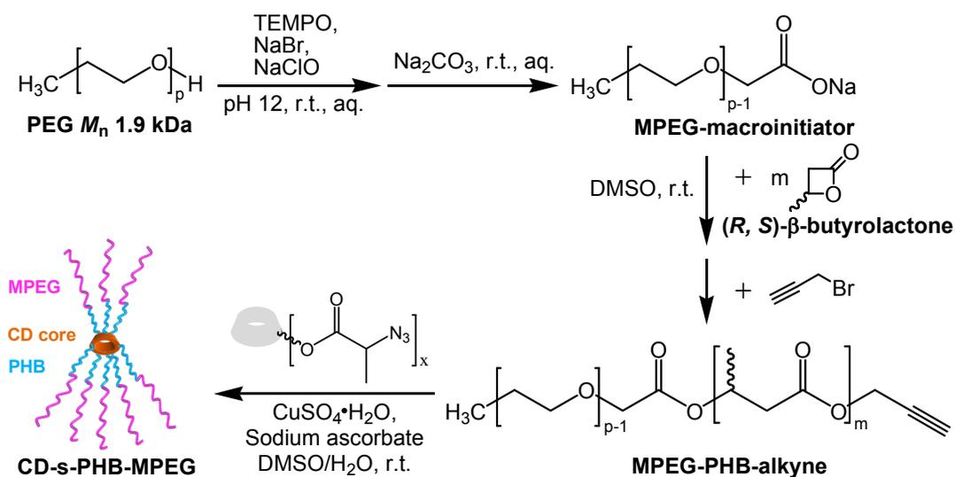
**Figure S5.** Synthetic route of CD-s-PHB-MPEG and the macroinitiator, MPEG-PHB with alkynyl functionality (MPEG-PHB-alkyne).
