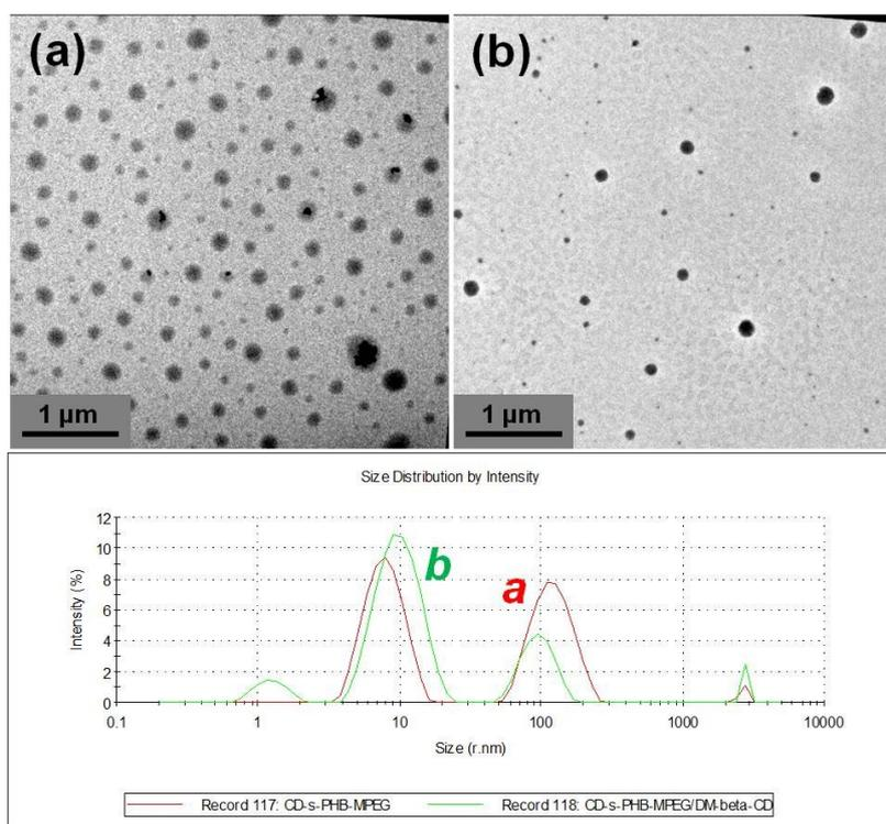
**Figure S8.** TEM images and particle size distribution of (a) CD-s-PHB-MPEG and DM- $\beta$ -CD/CD-s-PHB-MPEG (20:1) aggregates.
