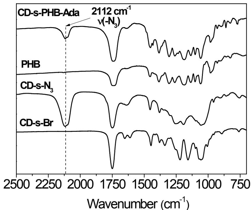
**Figure S4.** FTIR spectra of CD-s-PHB-Ada and its precursors in the form of KBr discs.
