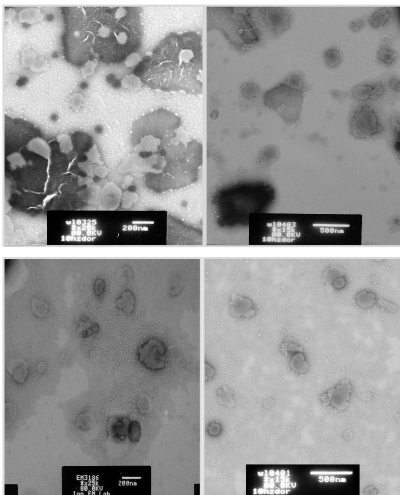
Fig. 1S Micrographs of liposomes obtained using a TEM (JEM-1230, JEOL, Japan) after adsorption of the samples on copper grids and staining negatively with 1% (w/v) uranyl acetate. A: 5-FU; B: tegafur; C: cisplatin; D: cytarabine.
