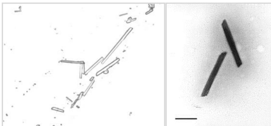
Fig. 2S Optical micrograph (left;  $\times 600$ ) and transmission electron micrograph (right; bar: 1  $\mu\text{m}$ ) of bundles of CNPTs precipitated from TFA/ $\text{CHCl}_3$ .
