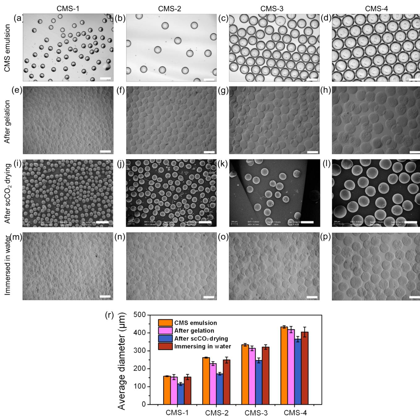
**Fig. S1** (a-d) Optical microscope images of CMS emulsions with different sizes. (e-h) Optical microscope images of solidified CMS microgels with different sizes. (i-l) Optical microscope images of dried NCMS with different sizes. (m-p) Optical microscope images show dried NCMS with different sizes immersing in water. Scale bar is 400  $\mu\text{m}$ . (r) Statistical sizes of the four types of CMS.
