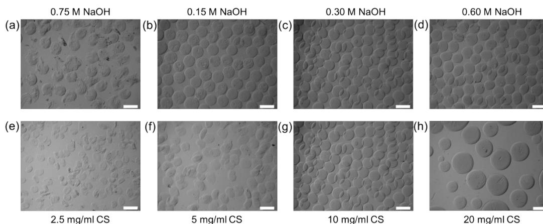
**Fig. S2** (a-d) Optical microscope images of the CMS microgels solidified with different concentrations of NaOH solutions. (e-h) Optical microscope images of the CMS microgels made from different concentrations of CS. (r) Statistical sizes of the four types of CMS. Scale bar is 400  $\mu\text{m}$ .
