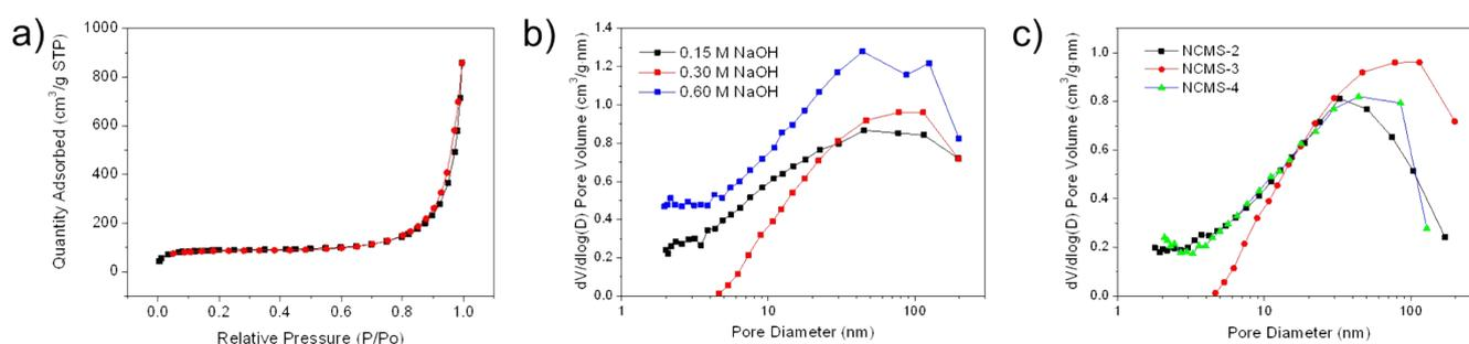
**Fig. S3**  $\text{N}_2$  sorption isotherms (a) and pore size distribution (b,c) from the BJH method reveal that the pores in the NCMS prepared at different conditions are macropores.
