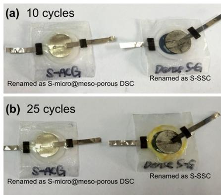
**Fig. S6** Photos of the transparent soft pack cells of S-micro@meso-porous DSC and S-SSC after (a) 10 cycles, (b) 25 cycles.
