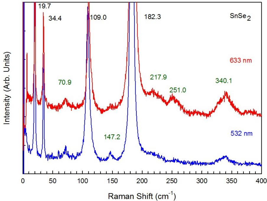
Fig. S2 Raman spectra of bulk  $\text{SnSe}_2$  under 532-nm and 633-nm excitations. These weak modes are marked in green.
