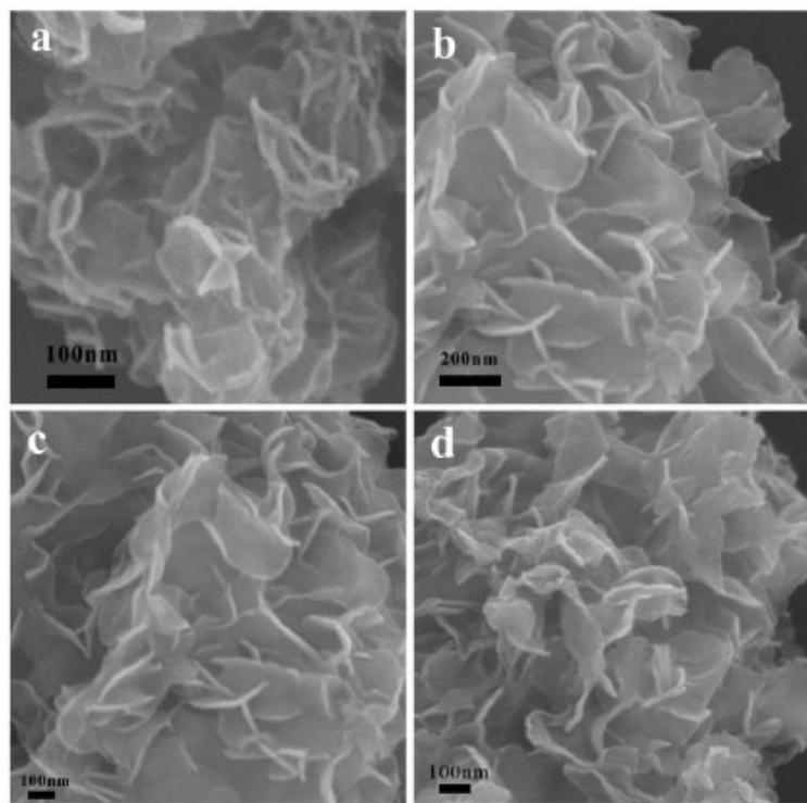
**Fig. S3** TEM images of graphene (a), C/MoS<sub>2</sub>@G<sub>1</sub> (b), C/MoS<sub>2</sub>@G<sub>2</sub> (c), C/MoS<sub>2</sub>@G<sub>3</sub> (d) and C/MoS<sub>2</sub>@G<sub>4</sub> (e).
