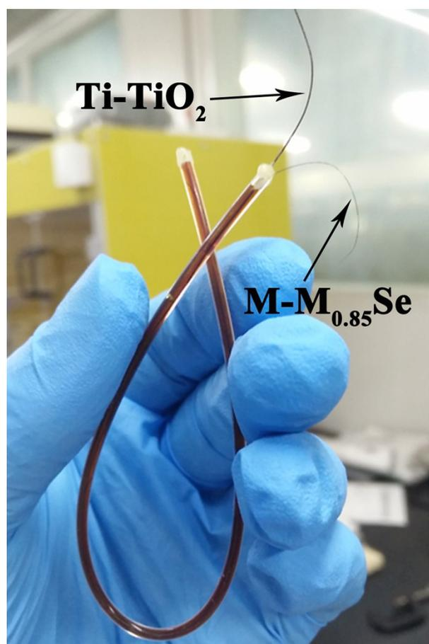
**Figure S2.** Photograph of FDSSC based on the Ni<sub>0.85</sub>Se CE.
