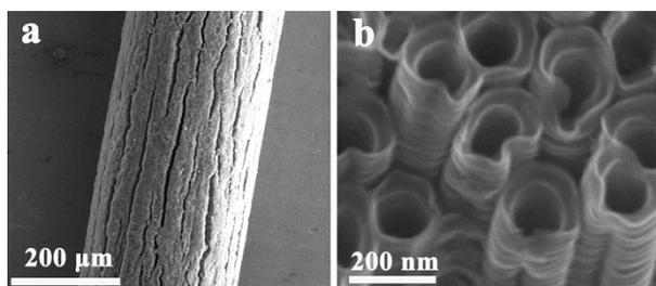
**Figure S1.** a) FE-SEM images of Ti fiber coating with TiO<sub>2</sub> nanotube, b) high magnification FE-SEM images of TiO<sub>2</sub> nanotube.
