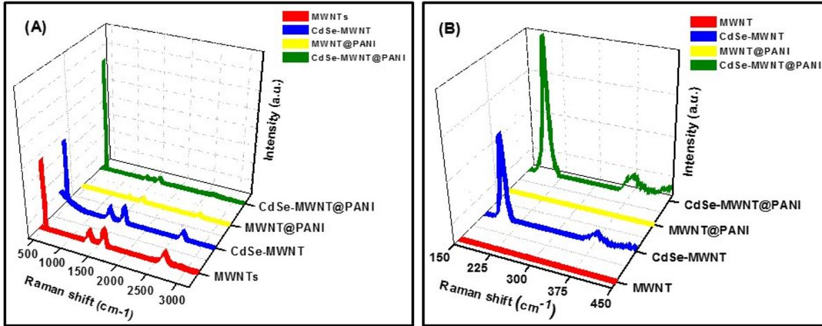
**Fig. S4.** Raman spectra of (A) MWCNTs, CdSe-MWCNT, MWCNT@PANI and CdSe-MWCNT@PANI in the range 500-3200  $\text{cm}^{-1}$  excited at 633 nm, and (B) MWCNTs, CdSe-MWCNT, MWCNT@PANI and CdSe-MWCNT@PANI in the range of 100-450  $\text{cm}^{-1}$  excited at 488 nm.
