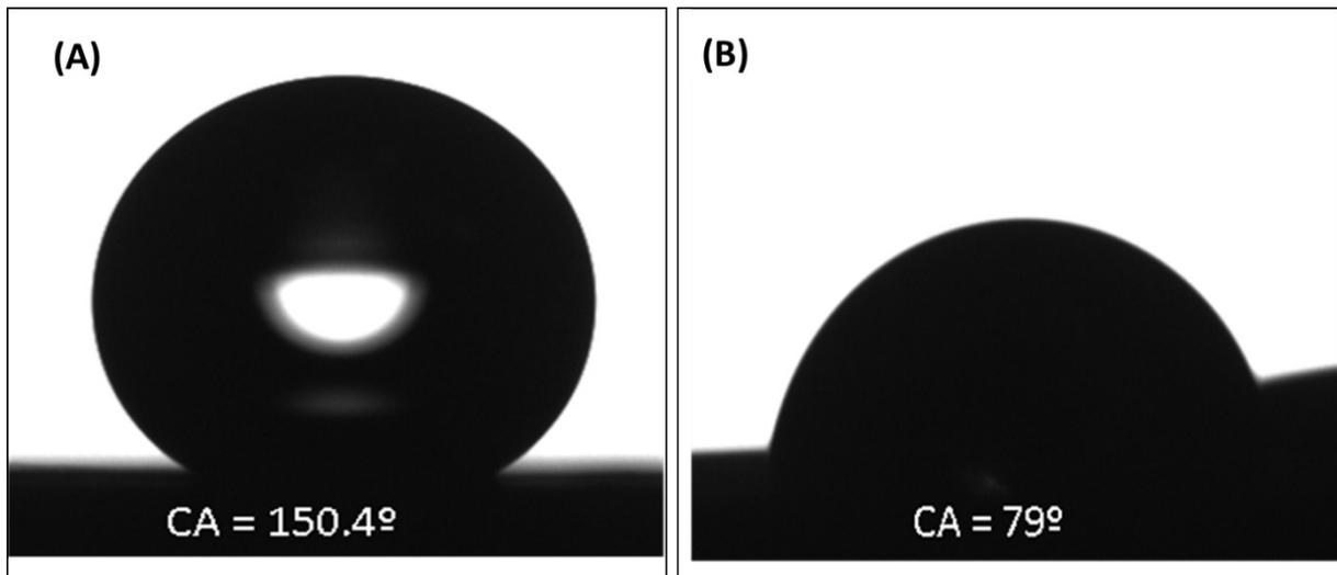
**Fig. S5.** CCD photographs showing the contact angle measurements of a water drop resting on (A) MWCNTs and (B) MWCNT@PANI.
