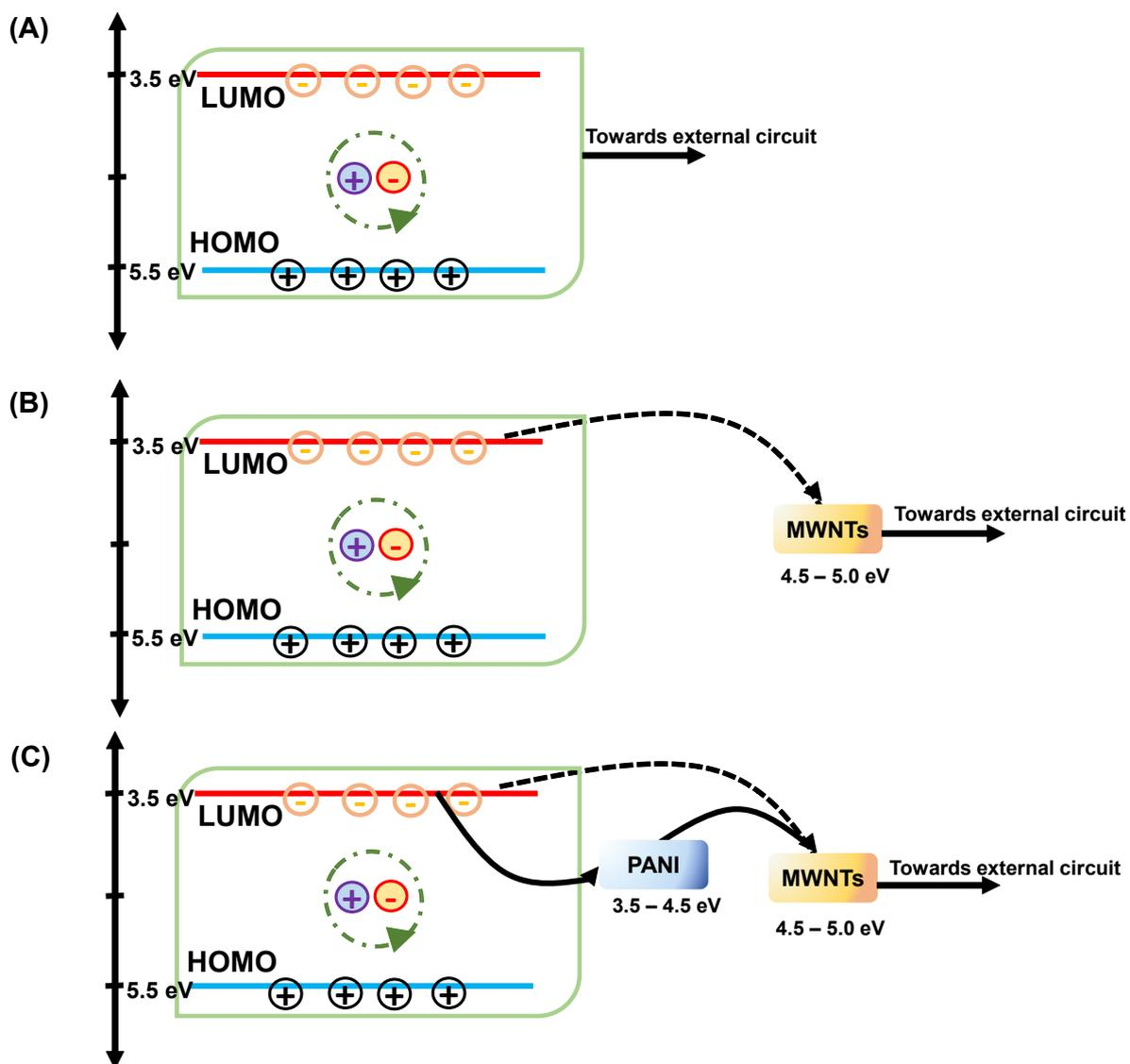
**Fig. S6.** Charge transfer mechanism occurred within (A) CdSe QDs, (B) photoactive cell containing CdSe and MWCNTs, and (C) photoactive cell based on CdSe-MWCNT@PANI (present device).
