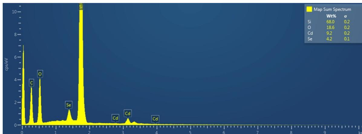
**Fig. S3.** EDS spectrum of CdSe-MWCNT@PANI indicating the presence of various elements in the device such as carbon, selenium, cadmium, and oxygen. Silicon is the base of the device.
