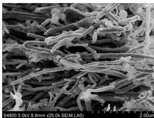
Fig. S8 FESEM image of CuNWs@ZIF-8 after reused for three times in \text{NH}_3\text{BH}_3 hydrolysis reaction. Reaction conditions are given in Figure 6.
