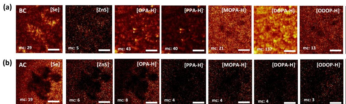
**Fig. S2** Comparison of ToF-SIMS data obtained from CdSe/ZnS QDs (a) before and (b) after purification at negative ion mode. Scale bars indicate 50  $\mu\text{m}$ .
