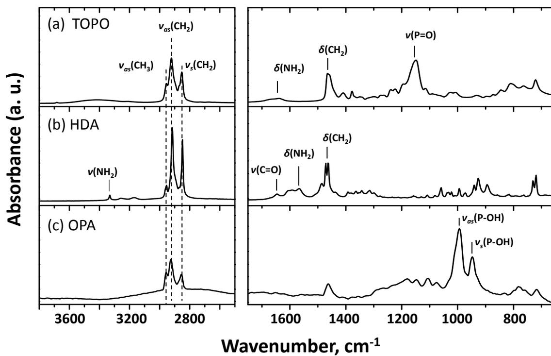
**Fig. S4** IR spectra of free ligands in hexane. The peak intensities in the right column were doubled as compared to the left column.
