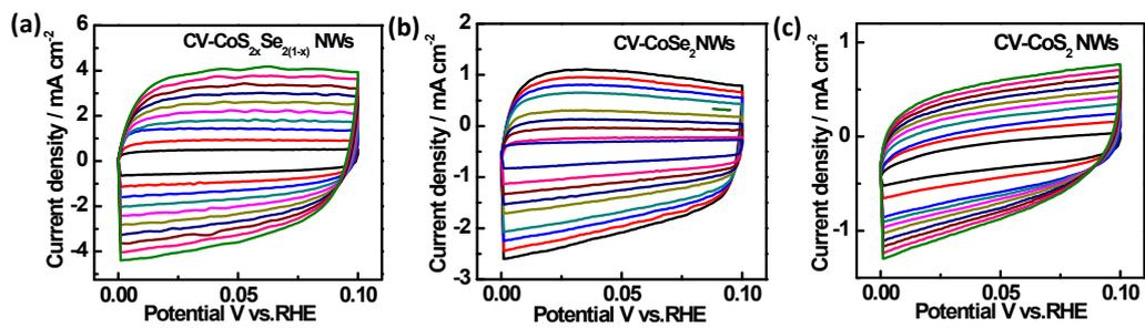
**Fig. S5.** Cyclic voltammograms (CV) curves of different catalysts:  $\text{CoS}_{2x}\text{Se}_{2(1-x)}$  NWs (a),  $\text{CoSe}_2$  NWs (b) and  $\text{CoS}_2$  NWs (c) at scan rates of 20mV/s-200 mV/s.
