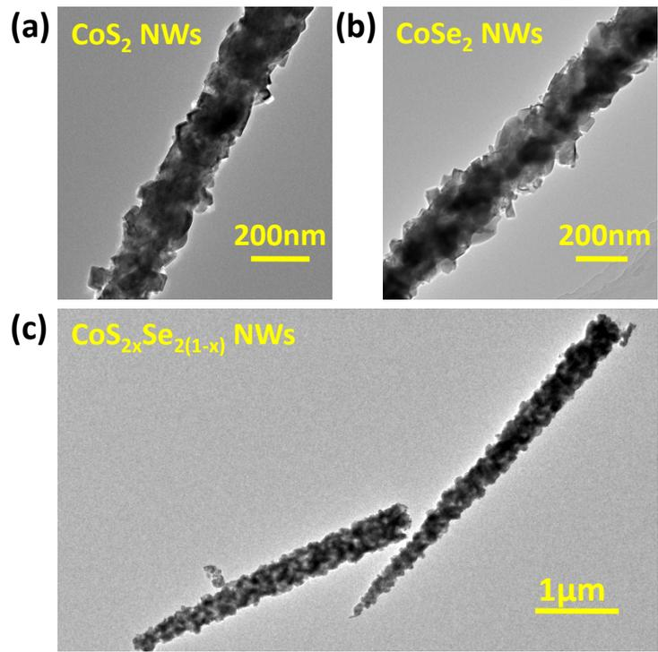
Fig. S1. TEM image of CoS<sub>2</sub> NWs (a), CoSe<sub>2</sub> NWs (b) and CoS<sub>2x</sub>Se<sub>2(1-x)</sub> NWs (c).
