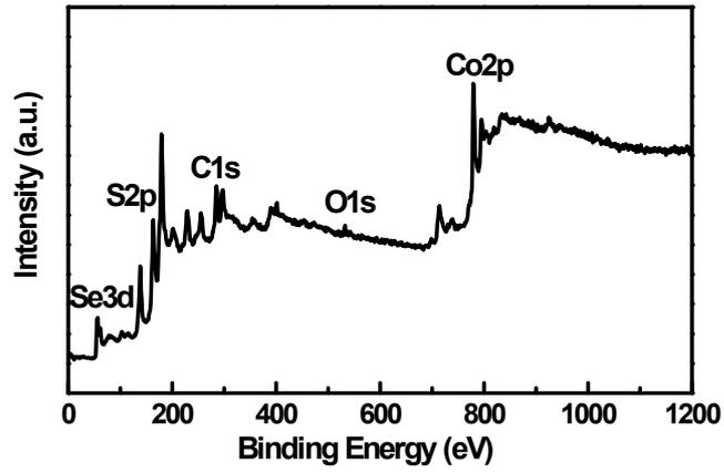
Fig. S3 XPS spectra of  $\text{CoS}_{2x}\text{Se}_{2(1-x)}$  NWs/CF.
