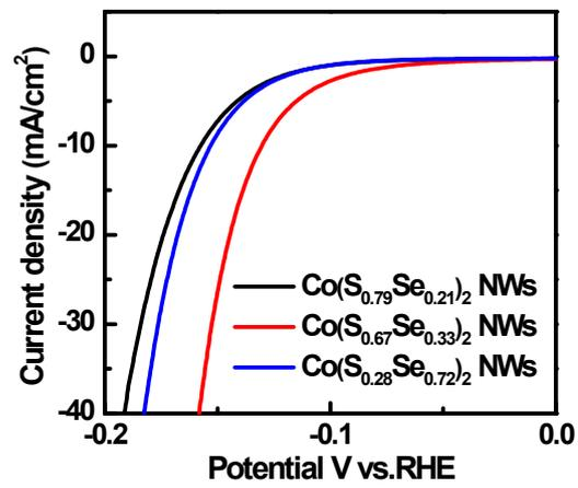
Fig. S4. Polarization curves of different ternary samples with various elemental components.
