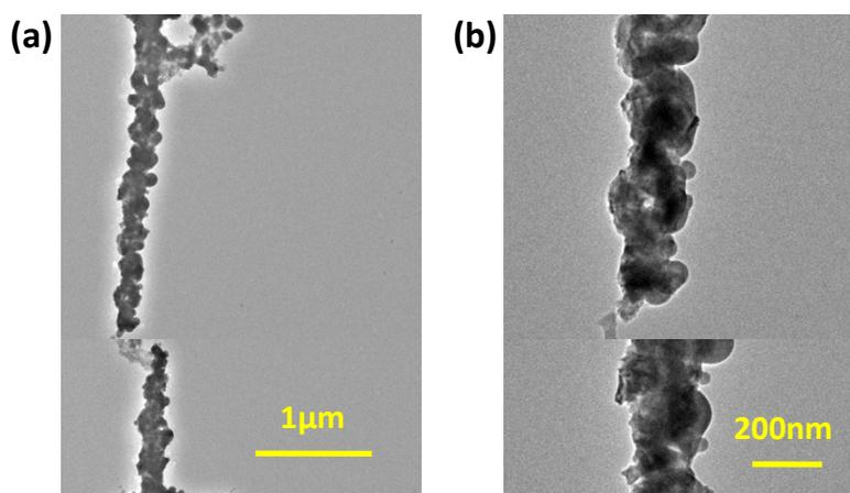
**Fig. S6.** Low magnification (a) and high magnification (b) TEM images of  $\text{CoS}_{2x}\text{Se}_{2(1-x)}$  NWs after 1000 potential cycles.
