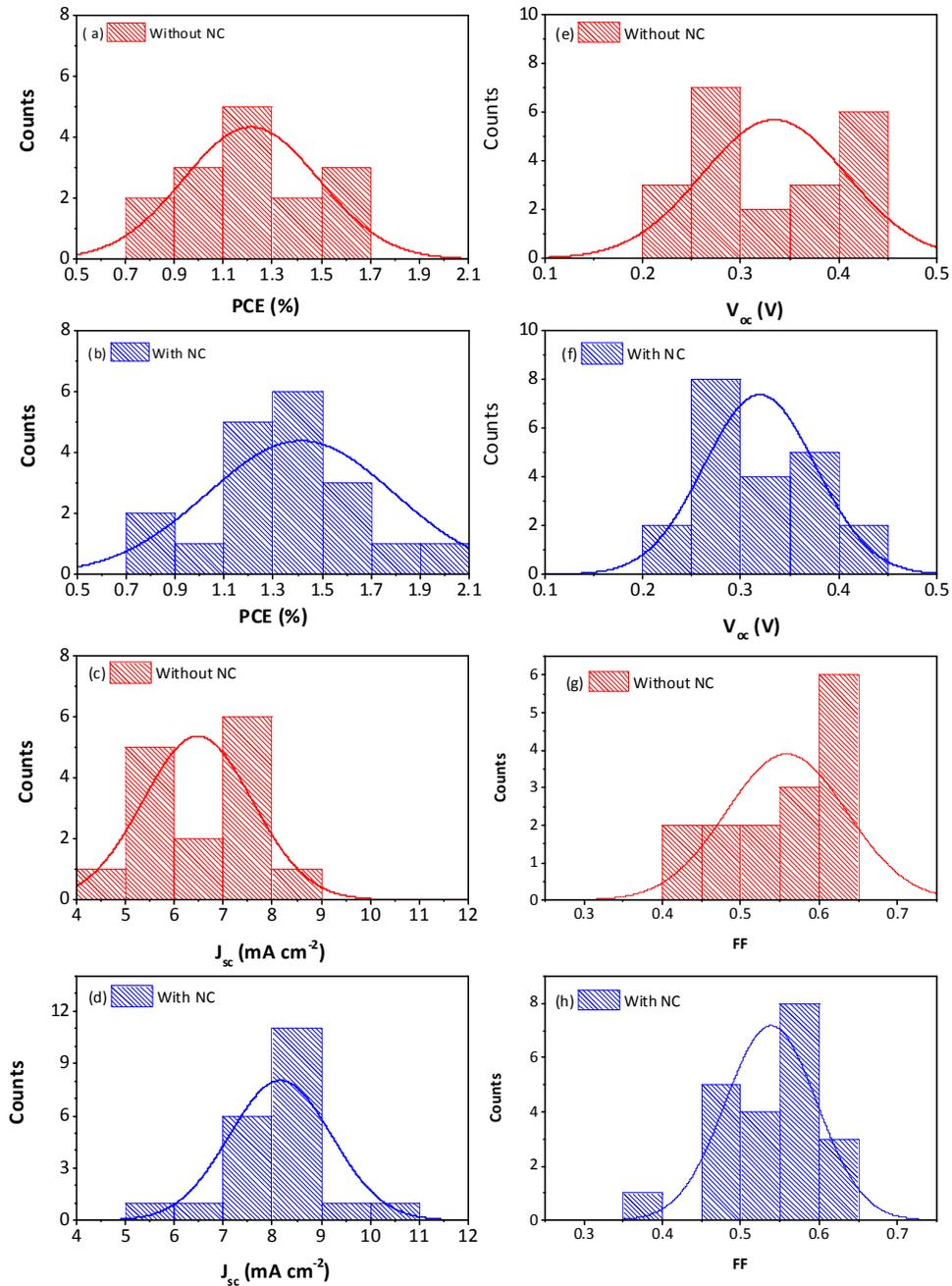
**Figure S5.** Histogram of PV characteristics of ultrathin Si solar cells having 14 nm thick  $\text{AlO}_x$  spacer, with (blue-dashed) or without (red-dashed) four monolayers of CdSe/ZnS core-shell NC energy donor.
