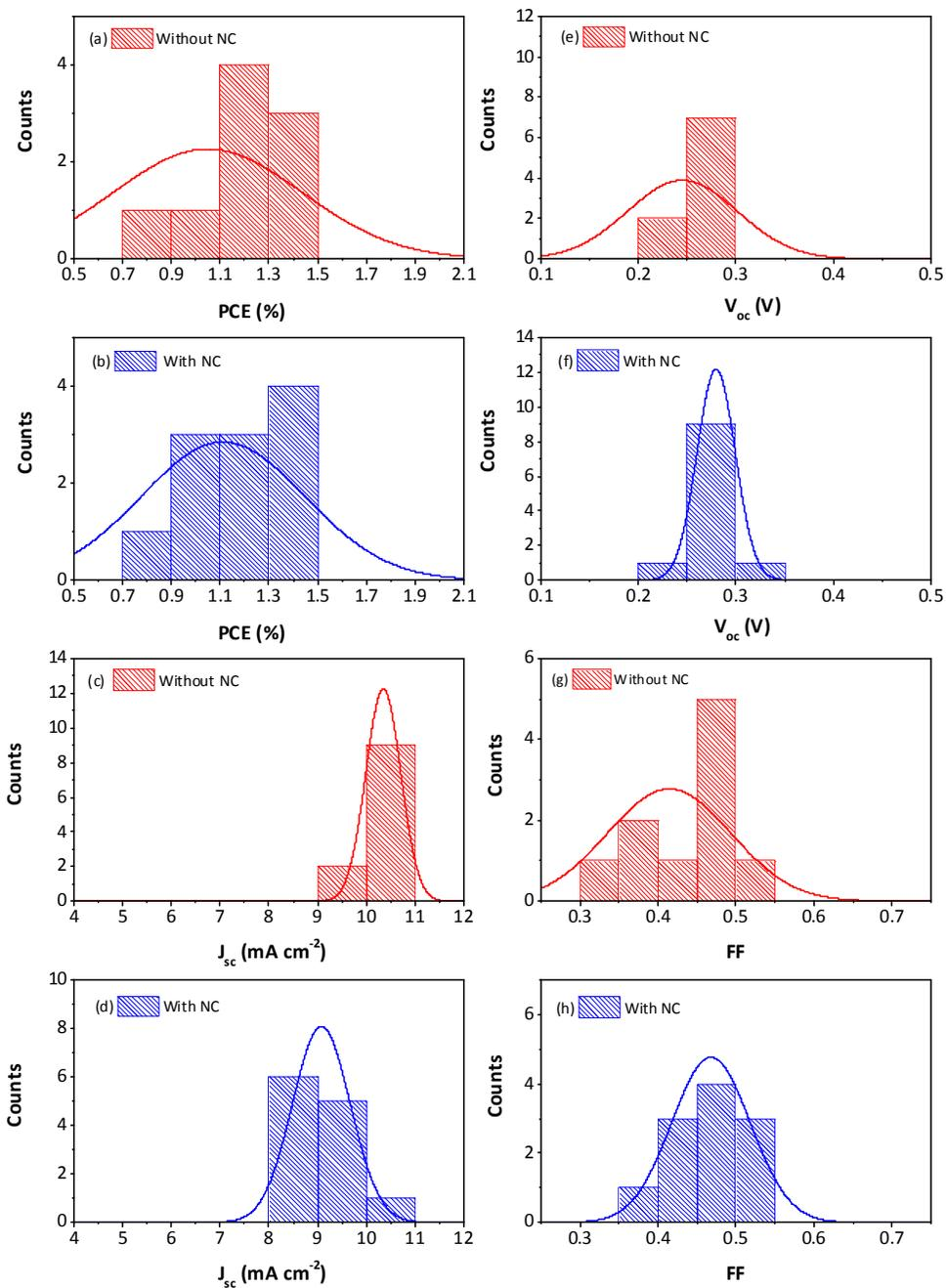
**Figure S8.** Histogram of PV characteristics of ultrathin Si solar cells having 46 nm thick  $\text{AlO}_x$  spacer, with (blue-dashed) or without (red-dashed) four monolayers of CdSe/ZnS core-shell NC energy donor.
