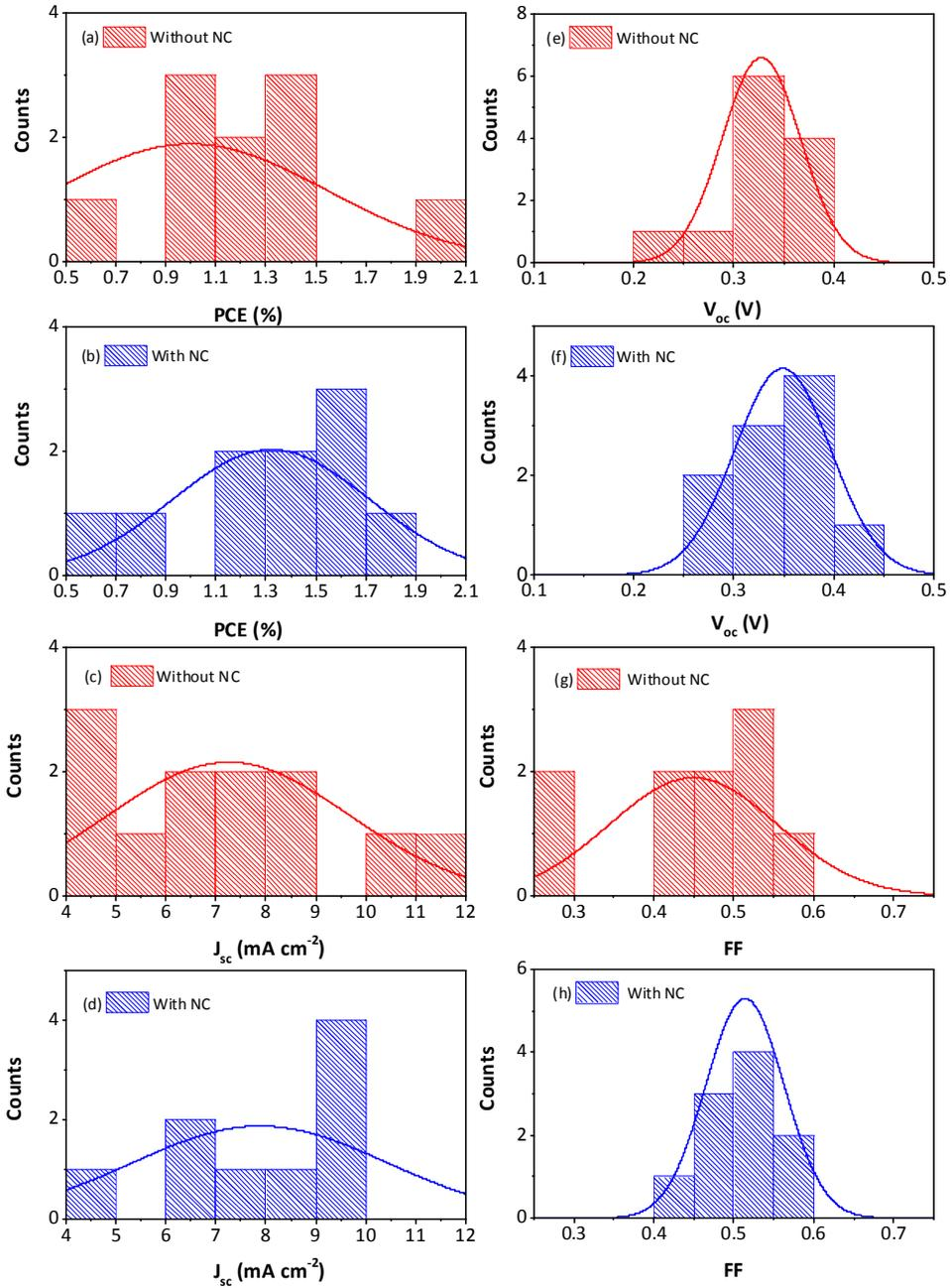
**Figure S7.** Histogram of PV characteristics of ultrathin Si solar cells having 36 nm thick  $\text{AlO}_x$  spacer, with (blue-dashed) or without (red-dashed) four monolayers of CdSe/ZnS core-shell NC energy donor.
