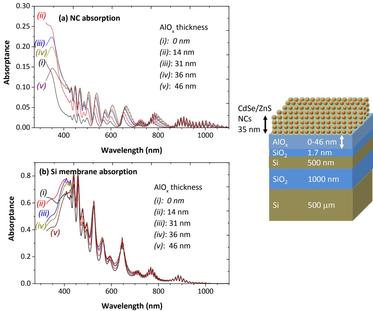
**Figure S3.** Simulated absorbance spectra of (A) 35 nm thick CdSe/ZnS NC layer and (B) 500 nm thick Si membrane in the device structure as a function of  $\text{AlO}_x$  thickness. It is noted that for calculating  $J_{ET}$  contributed by NC, the photocurrent integration over AM1.5G spectrum was done up to 650 nm cutoff wavelength to exclude the spurious optical absorption of NC layer appearing  $\lambda > 650$  nm in the simulation.
