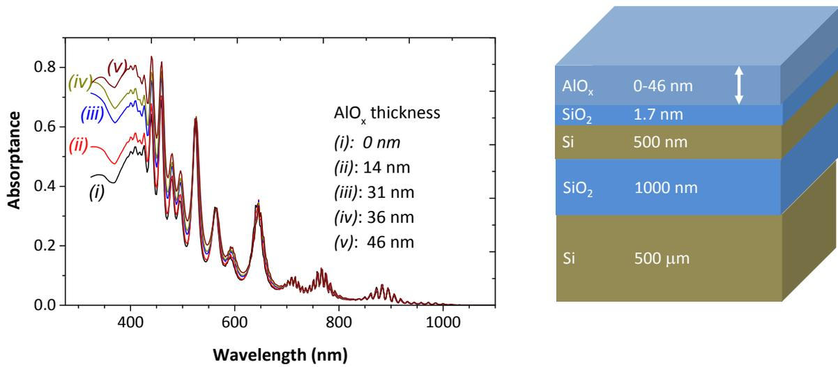
**Figure S2.** Simulated absorbance spectra of the Si membrane (500 nm thickness) in the silicon-on-insulator (SOI) substrate as a function of the thickness of the AlO<sub>x</sub> layer.
