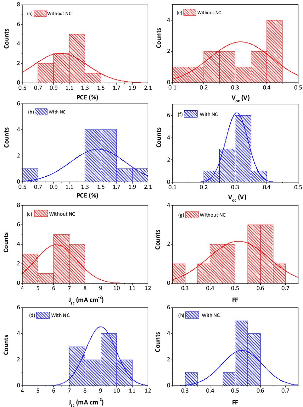
**Figure S6.** Histogram of PV characteristics of ultrathin Si solar cells having 31 nm thick  $\text{AlO}_x$  spacer, with (blue-dashed) or without (red-dashed) four monolayers of CdSe/ZnS core-shell NC energy donor.
