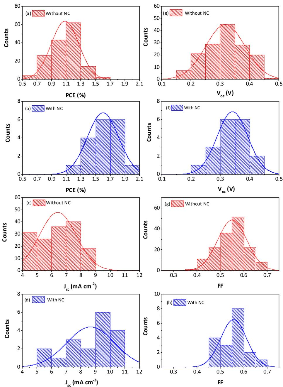
**Figure S1.** Histogram of photovoltaic (PV) characteristics of ultrathin Si solar cells having no  $\text{AlO}_x$  spacer, with (blue-dashed) or without (red-dashed) four monolayers of CdSe/ZnS core-shell NC energy donor.
