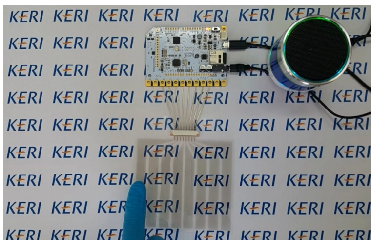
Fig. S5 Flexible touch piano consisting of a CNT touch keyboard, Ag interconnects, an Arduino-based control board, and a speaker. Movie S1 shows that we were able to play a tune ('Twinkle Twinkle Little Star') on this touch piano.
