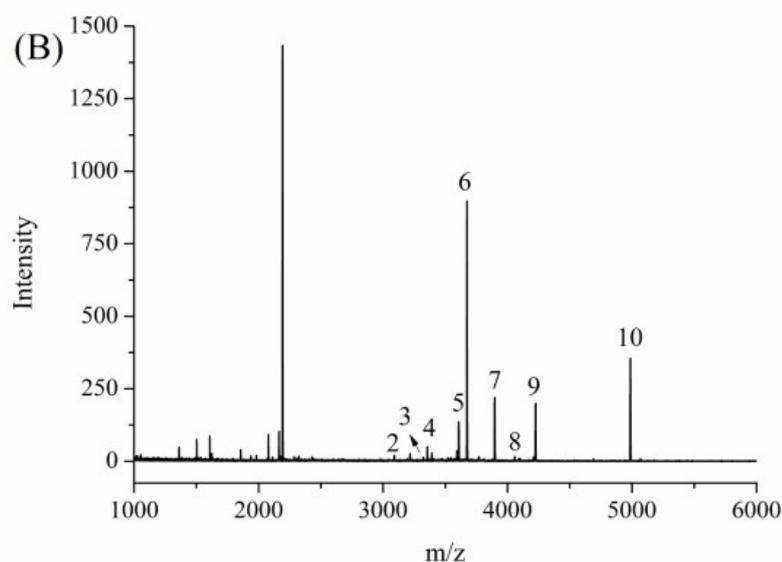
Fig. S5 MALDI-TOF MS spectra of the enriched glycopeptides from the tryptic digest mixture of HRP and Myo with the mass ratio of (A) 1:10 and (B) 1:100.
