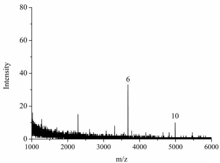
Fig. S3 MALDI-TOF MS spectra of 25 fmol tryptic HRP after enrichment by GO/Fe<sub>3</sub>O<sub>4</sub>/Au/PEG nanocomposites.
