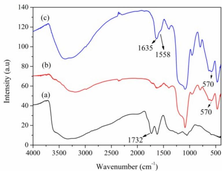
Fig. S1 FT-IR spectra of (a) GO nanosheets, (b) magnetic nanoparticles and (c) GO/Fe<sub>3</sub>O<sub>4</sub> nanocomposites.
