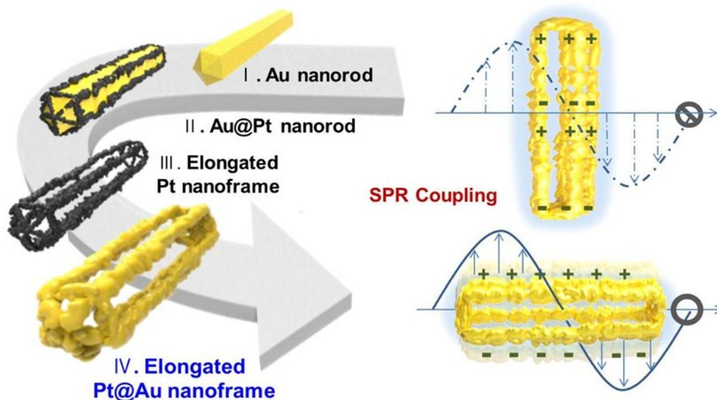
Schematic illustration of the elongated Pt@Au nanoframes; Unique surface plasmon features were observed for elongated Pt@Au nanoframes where the short-axis oscillation of surface free electrons is strongly coupled but the long-axis oscillation is not coupled among ridges.
