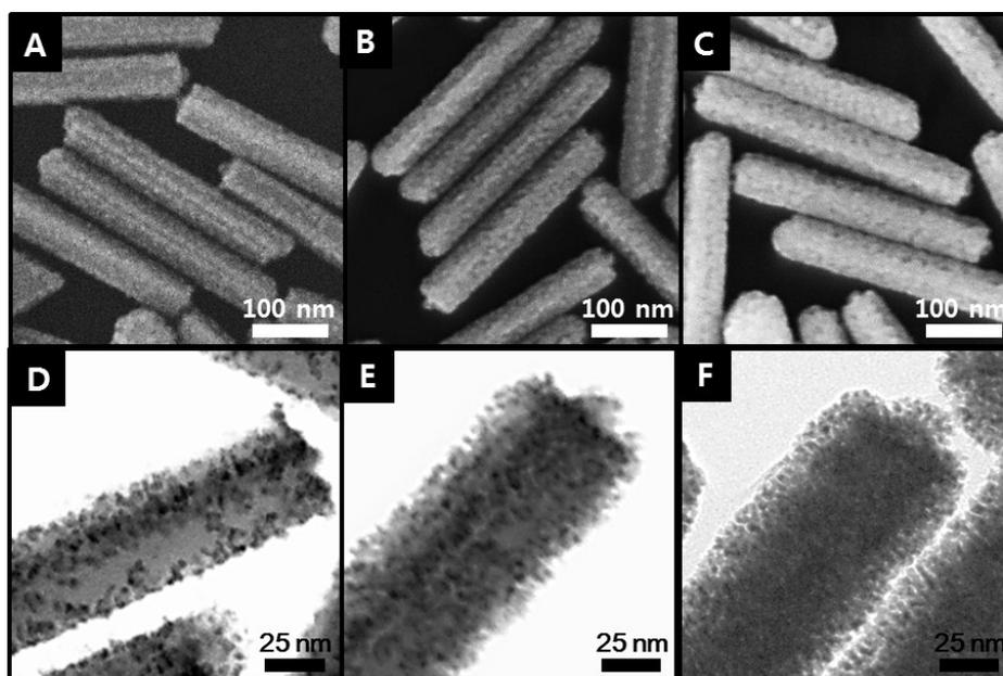
Fig.S3 SEM images (A,B,C) of Au@Pt nanorods and their corresponding TEM images (D,E,F) showing detailed morphology. As the amount of Pt increased (from A to C and D to F), the surface of nanorods is fully coated with Pt, not edge-preferential growth.
