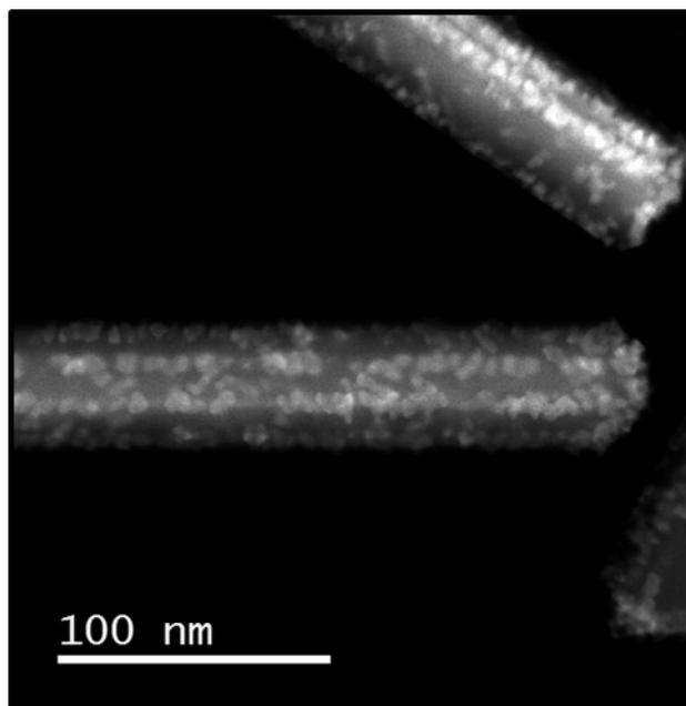
Fig.S2 TEM image demonstrating edge-preferential deposition of Pt onto Au nanorod in an island growth mode.
