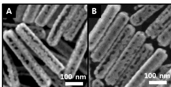
Fig.S5 SEM images of elongated Pt@Au nanoframes before (A) and after (B) O<sub>2</sub> plasma treatment for 6 min.
