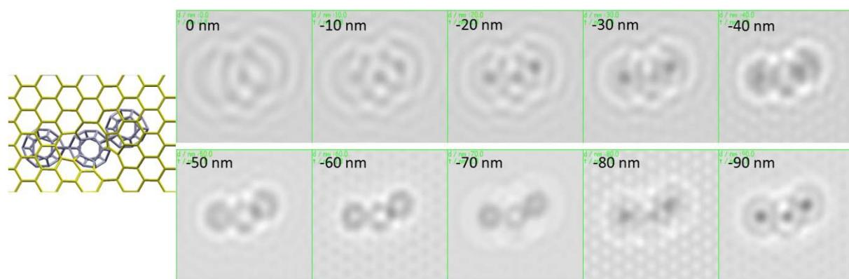
The following figure shows the simulation of two *unpolymerized* molecules of  $C_{20}$  on a graphene surface.
