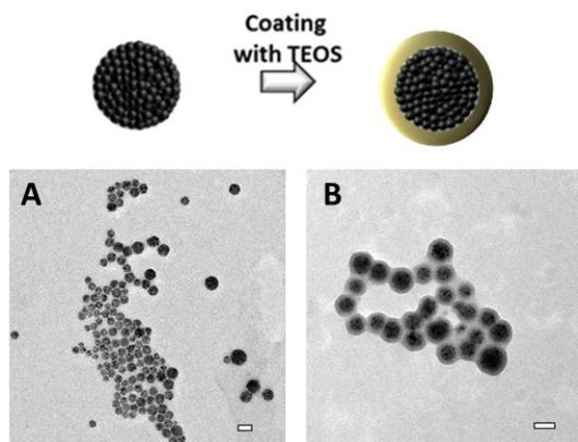
**Fig. S2.** TEM images of magnetic hybrid nanoparticles before (A) and after (B) coating them with a silica shell of *ca.* 40 nm (sample **1b**). The scale bars represent 100 nm.
