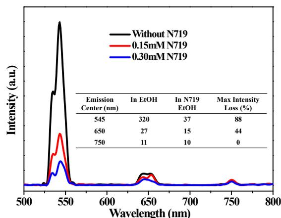
**Fig. S3** Upconversion fluorescence spectra of YbF<sub>3</sub>-Ho in N719 and EtOH solution.
