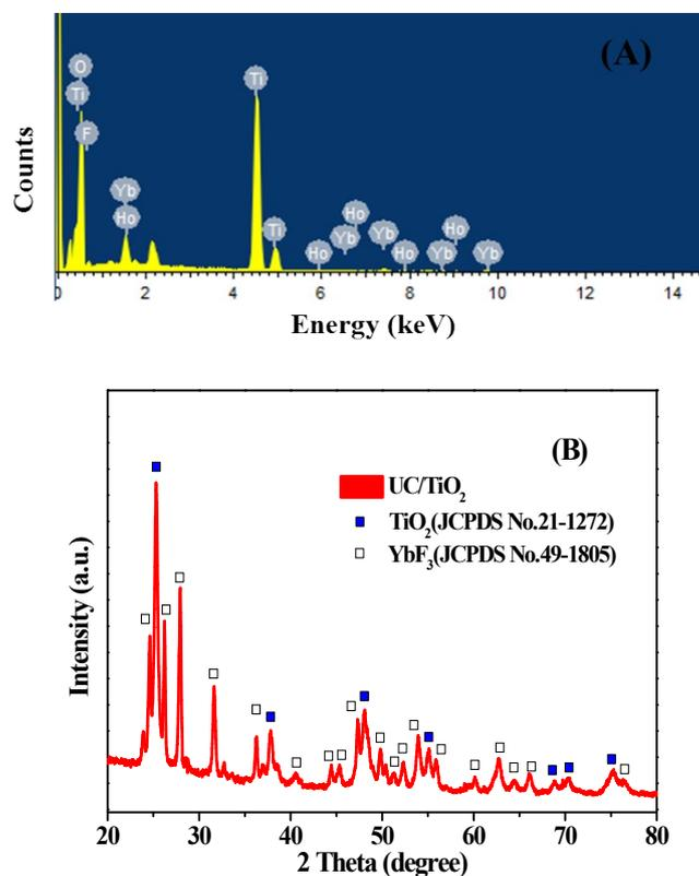
Fig. S2 EDX and XRD analyses of UC/ $\text{TiO}_2$  nanoheterostructures.
