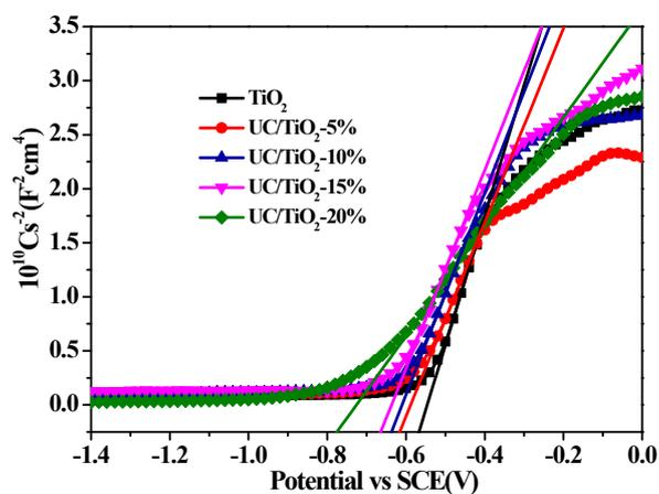
**Fig. S5** Mott-Schottky plots of the  $\text{TiO}_2$  and UC/ $\text{TiO}_2$  photoelectrode films.
