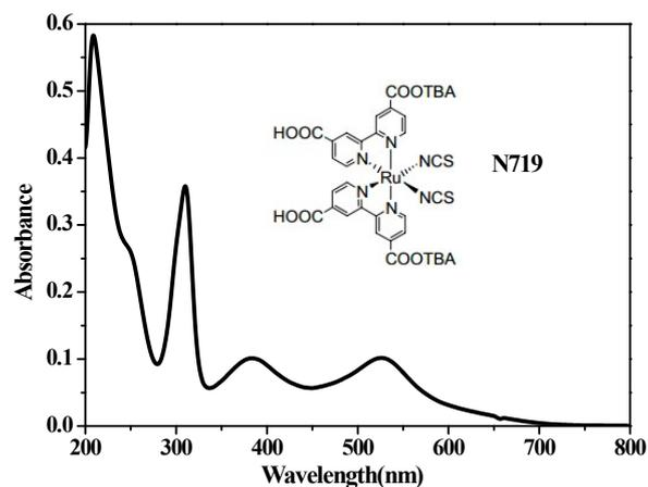
**Fig. S4** UV-vis absorption spectrum of N719 in ethanol solution and chemical structure is shown as inset.
