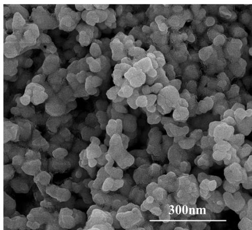
Fig. S1 SEM image of  $\text{YbF}_3\text{-Ho}$ .
