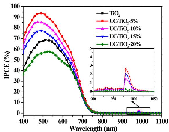
**Fig. S6** IPCE spectra of DSSCs with  $\text{TiO}_2$  and UC/ $\text{TiO}_2$  photoelectrodes.
