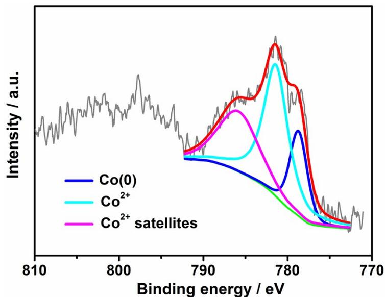
Figure S5. The high-resolution XPS spectrum of Co2p of Pd<sub>6</sub>Co/3DG.
