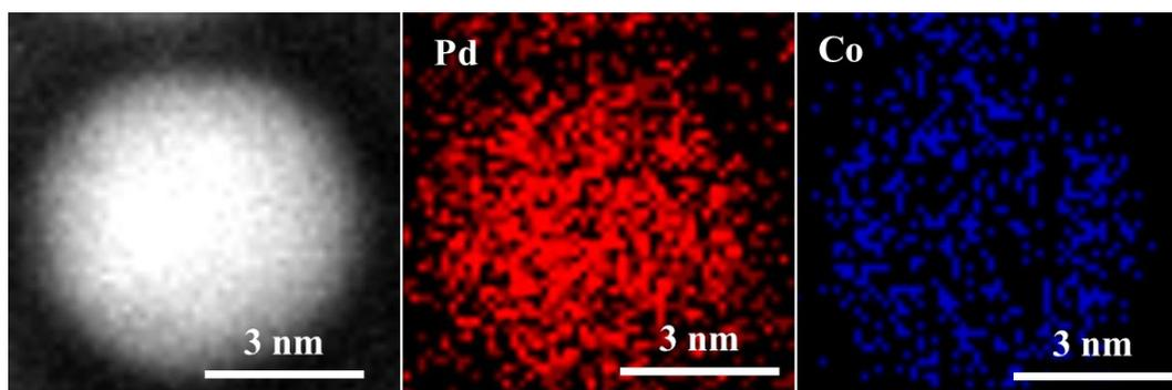
Figure S4. EDAX mapping images of Pd and Co elements distribution of a  $\text{Pd}_6\text{Co}$  nanoparticle.
