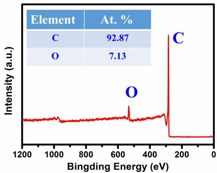
Figure S1. XPS spectrum of prepared 3DG materials.
