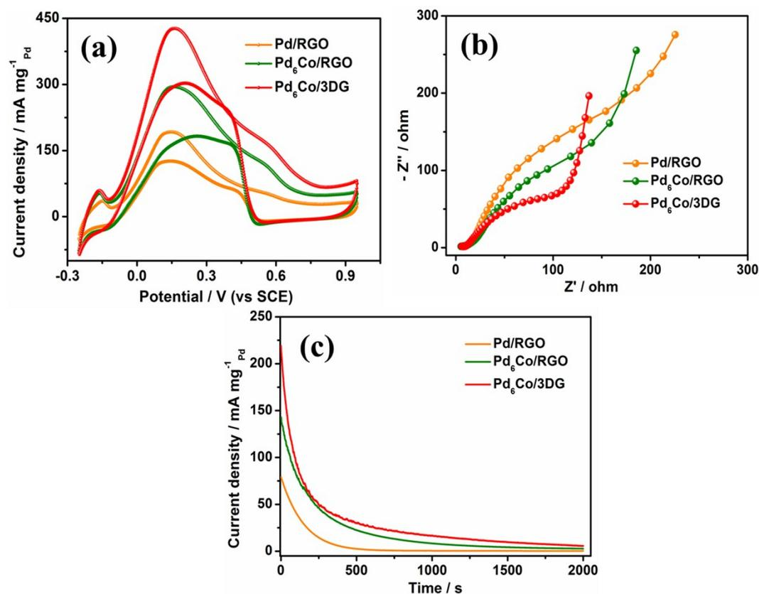
Figure S7. (a) CV curves of formic acid oxidation for Pd<sub>6</sub>Co/3DG, Pd<sub>6</sub>Co/RGO and Pd/RGO catalysts in 0.5 M H<sub>2</sub>SO<sub>4</sub> + 0.5 M HCOOH at 50 mV s<sup>-1</sup>. (b) Nyquist plots of Pd<sub>6</sub>Co/3DG, Pd<sub>6</sub>Co/RGO and Pd/RGO catalysts. (c) CA curves of Pd<sub>6</sub>Co/3DG, Pd<sub>6</sub>Co/RGO and Pd/RGO catalysts in 0.5 M H<sub>2</sub>SO<sub>4</sub> + 0.5 M HCOOH at 0.1 V.
