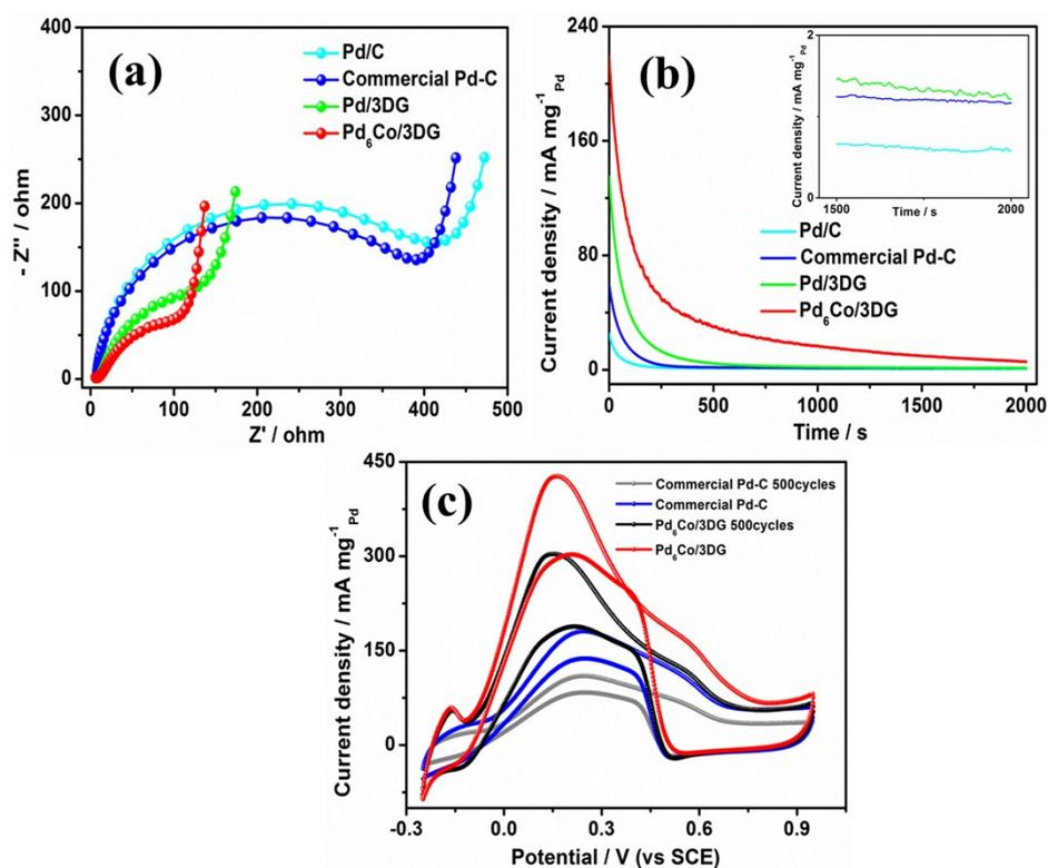
Figure S6. (a) Nyquist plots of various Pd-based catalysts. (b) chronoamperometric (CA) curves of various Pd-based catalysts in 0.5 M H<sub>2</sub>SO<sub>4</sub> + 0.5 M HCOOH at 0.1 V. (c) CV curves of Pd<sub>6</sub>Co/3DG and commercial Pd-C catalysts before and after repeated cycling (500 cycles, from -0.25V to 0.95V at 50 mV s<sup>-1</sup>)
