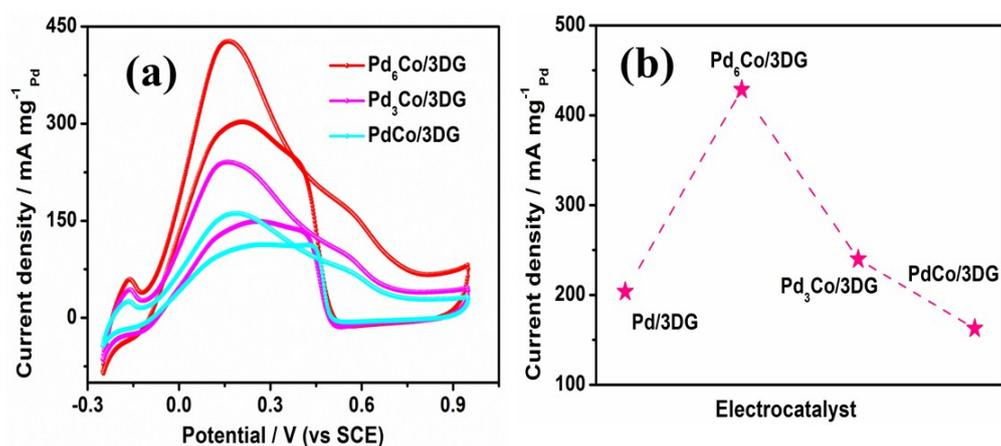
Figure S8. (a) CV curves of formic acid oxidation for Pd<sub>6</sub>Co/3DG, Pd<sub>3</sub>Co/3DG and PdCo/3DG catalysts in 0.5 M H<sub>2</sub>SO<sub>4</sub> + 0.5 M HCOOH at 50 mV s<sup>-1</sup>. (b) The catalytic peak current density of various Pd-based catalyst including Pd<sub>6</sub>Co/3DG, Pd<sub>3</sub>Co/3DG, PdCo/3DG and Pd/3DG.
