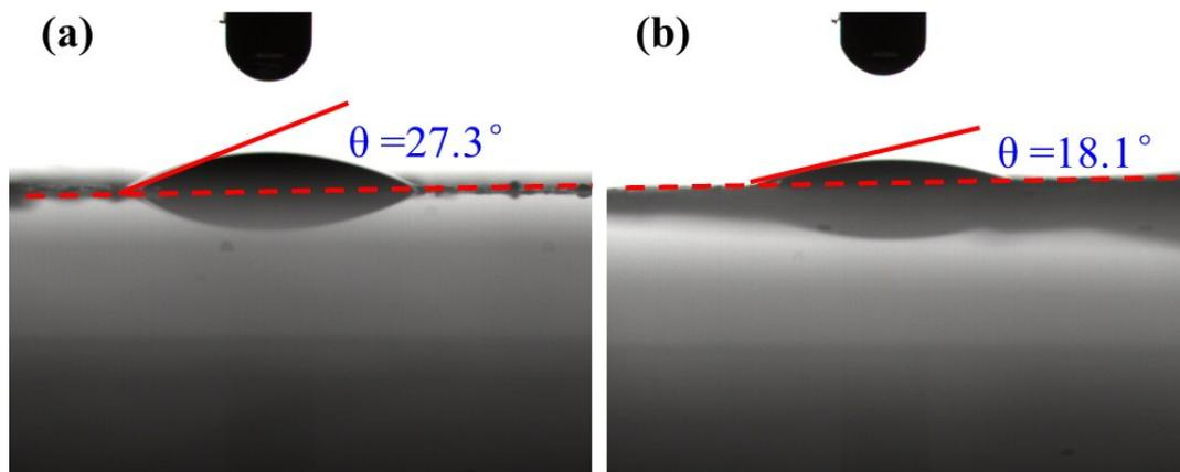
Figure S3. Ethylene glycol contact angle of XC-72 Carbon (a) and 3D graphene (b), respectively.
