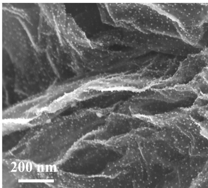
Figure S2. SEM image of prepared Pd/3DG materials.
