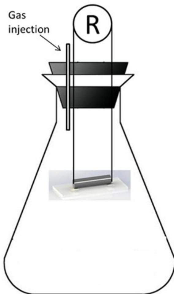
**Figure S7.** Experimental set-up for gas sensing measurement
