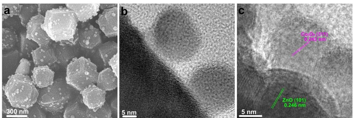
**Fig. S5** (a) SEM , (b) TEM and (c) high resolution TEM of ZIF-8@ZIF-67 derived ZnO@Co<sub>3</sub>O<sub>4</sub>.
