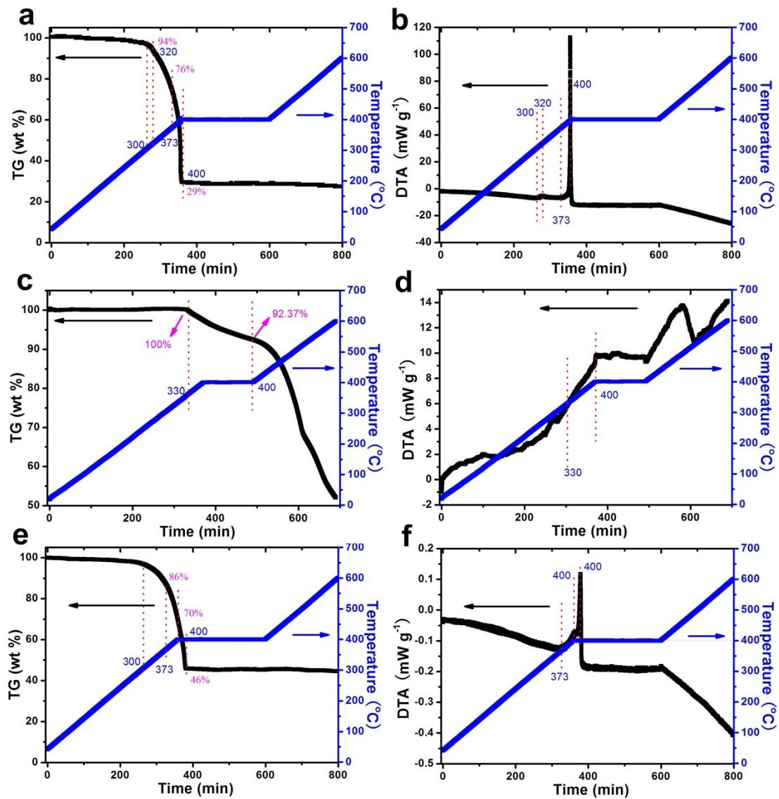
**Fig. S1** (a,b) TG and DTA curves of ZIF-8 recorded in air (one-step calcination). (c,d) TG and DTA curves of ZIF-8@ZIF-67 recorded in N<sub>2</sub> (the first-step calcination in a N<sub>2</sub> atmosphere); (e,f) TG and DTA curves of ZIF-8@ZIF-67 recorded in air (the second-step calcination in an air atmosphere).
