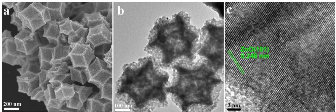
**Fig. S4** (a) SEM, (b) TEM, and (C) high resolution TEM images of ZIF-8 derived ZnO.
