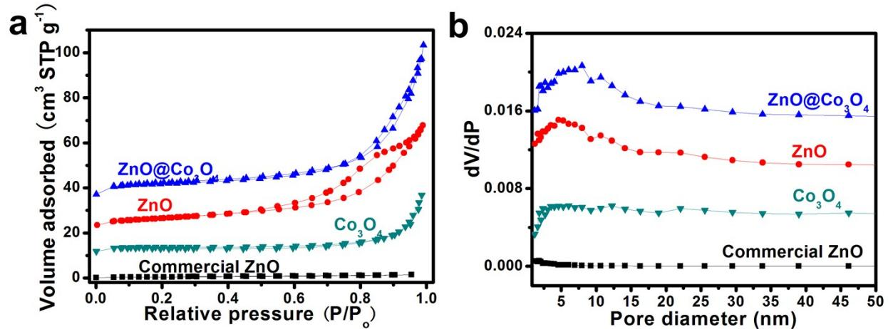
**Fig. S8** (a) N<sub>2</sub> adsorption-desorption isotherms and (b) pore size distribution of the ZIFs derived samples and the commercial ZnO.
