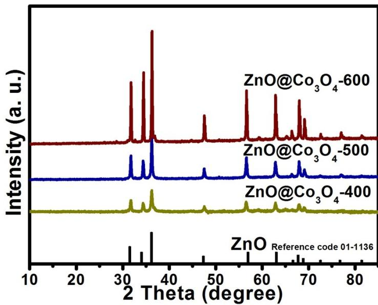
**Fig. S10** (a) XRD patterns ( $\lambda = 0.15418$  nm) of  $\text{ZnO}@\text{Co}_3\text{O}_4$ -400,  $\text{ZnO}@\text{Co}_3\text{O}_4$ -500 and (c,d)  $\text{ZnO}@\text{Co}_3\text{O}_4$ -600.
