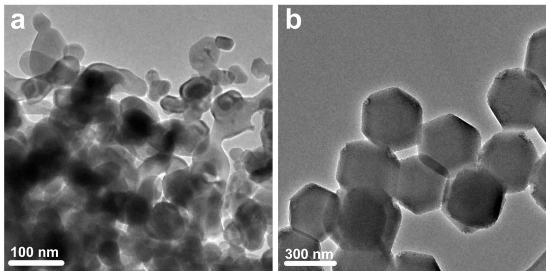
**Fig. S2** TEM image of (a) ZnO-2 prepared from ZIF-8 *via* one-step calcination in an ambient atmosphere, (b) ZnO@Co<sub>3</sub>O<sub>4</sub> precursor prepared from the core-shell ZIF-8@ZIF-67 crystals in a tubular furnace at 400 °C for 2 h under a N<sub>2</sub> atmosphere at a heating rate of 1 °C min<sup>-1</sup> to obtain.
