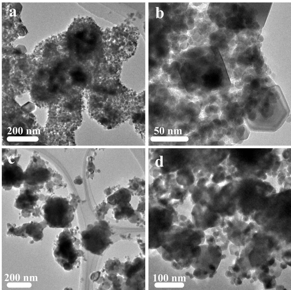
**Fig. S11** TEM images of (a,b) ZnO@Co<sub>3</sub>O<sub>4</sub>-500 and (c,d) ZnO@Co<sub>3</sub>O<sub>4</sub>-600 prepared from ZIF-8@ZIF-67.
