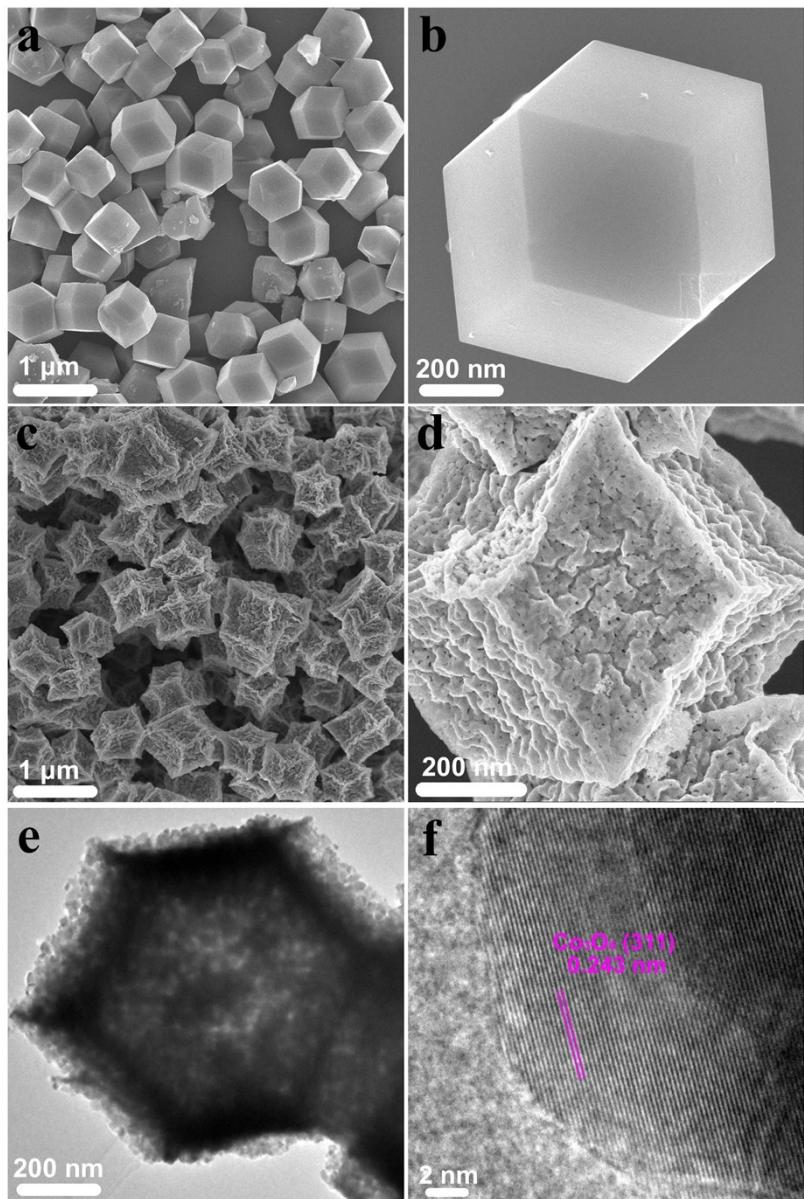
**Fig. S6** (a, b) SEM images of ZIF-67, (c, d) SEM, (e) TEM, and (f) high resolution TEM images of ZIF-67 derived Co<sub>3</sub>O<sub>4</sub>.
