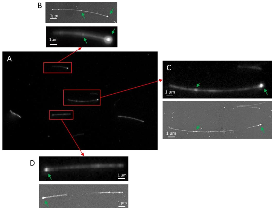
**Figure S 3.** Directly correlate the DFM image and SEM images on the same sample after GRR for  $\sim 2400$  s. (A) DFM image. (B)-(D) Examples for the direct correlation of the DFM image and SEM images SEM image.
