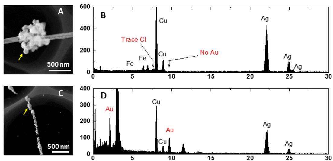
Figure S 4. TEM and EDX measurement of hot spots. (A) TEM of hot spots generated at 0.02 mM HAuCl<sub>4</sub>. (B) EDX of hot spots generated at 0.02 mM HAuCl<sub>4</sub>. (C) TEM of hot spots generated at 0.50 mM HAuCl<sub>4</sub>. (D) EDX of hot spots generated at 0.50 mM HAuCl<sub>4</sub>.
