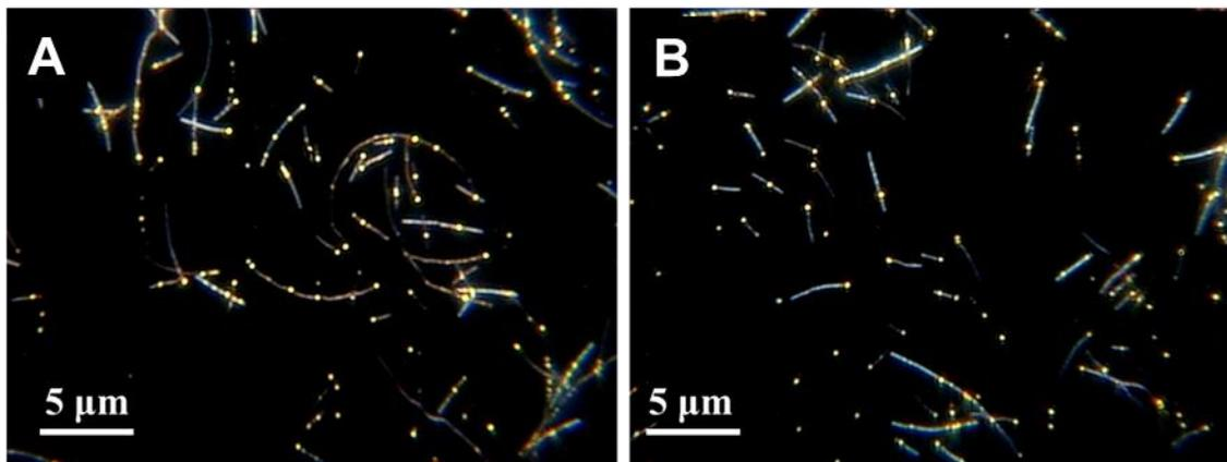
Figure S 2. Dark-field image of well dispersed single Ag nanowires taken by color camera after 2.4 ks GRR at 0.02 mM [HAuCl<sub>4</sub>].
