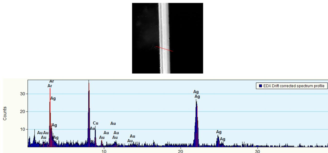
**Figure S 5.** STEM and EDX for the body of Ag nanowire reacted with 0.02 mM HAuCl<sub>4</sub> reacted for about 1200 s.
