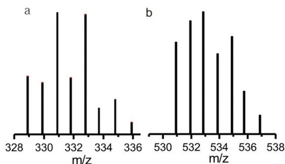
**Fig.S1** Characterization of intermediate product  $\text{c,c,t-Pt}(\text{NH}_3)_2\text{Cl}_2(\text{OH})_2$  and Pt(IV) prodrug. ESI-MS data of intermediate product (a) and Pt(IV) drug (b) in the negative ion mode. Formula of intermediate product:  $[\text{H}_8\text{O}_2\text{N}_2\text{Cl}_2\text{Pt}]^-$ ,  $m/z = 333.8$ ; Formula of Pt(IV) drug:  $[\text{C}_8\text{H}_{16}\text{N}_2\text{O}_8\text{Cl}_2\text{Pt}]^-$ ,  $m/z = 532.920$ .
