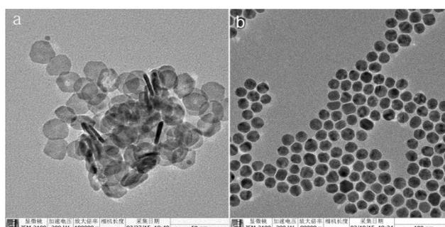
**Fig.S3** (a) Typical TEM images of  $\approx 30\text{ nm Pd@Au}$  with thickness of 4 nm and (b) 30 nm Au nanoparticles.
