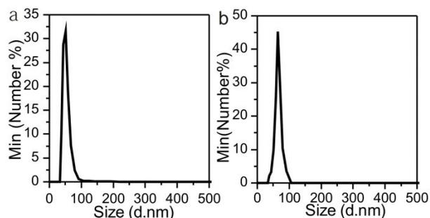
**Fig.S8** Size distribution of Pd@Au-PEG-Pt (52 nm) and Au-PEG-Pt (64 nm) nanoparticles in water.
