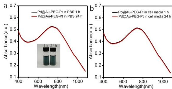
**Fig.S4** Absorption spectra of Pd@Au-PEG-Pt nanocomposite in PBS and cell media for 1 h and 24 h, respectively. Insert: photos of Pd@Au-PEG-Pt nanocomposite in PBS for 1 h and 24 h.
