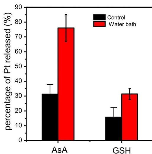
**Fig.S5** Chemical reduction of Pt(II) from the Pd@Au-PEG-Pt by 0.1 mM AsA or 0.6 mM GSH without or incubation in 39 °C water bath for 60 min, respectively.
