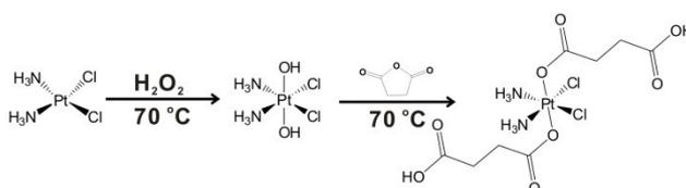
**Scheme S1.** Synthesis process of intermediate product  $\text{c,c,t-Pt}(\text{NH}_3)_2\text{Cl}_2(\text{OH})_2$  and Pt(IV) prodrug  $\text{c,c,t-Pt}(\text{NH}_3)_2\text{Cl}_2(\text{OOCCH}_2\text{CH}_2\text{CO}_2\text{H})_2$ .
