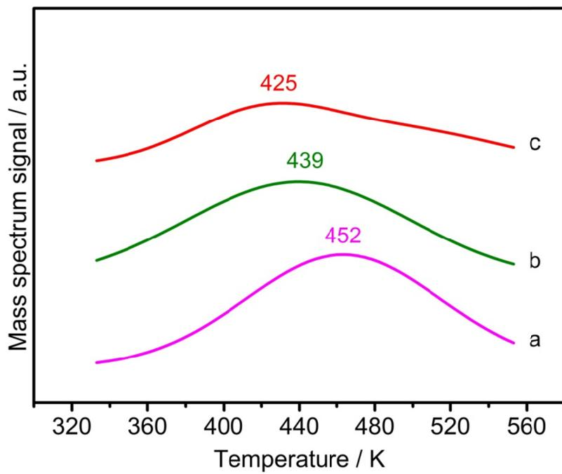
**Figure S35.** Mass spectra of H<sub>2</sub>-TPD for surface “clean” (a) Rh<sub>2</sub>Ni nanocubes, (b) Rh<sub>2</sub>Ni truncated nanoctahedrons and (c) Rh<sub>2</sub>Ni nanoctahedrons.
