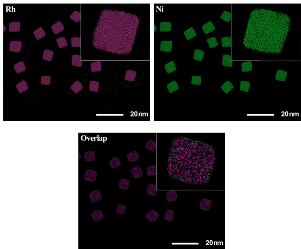
**Figure S27.** The elemental maps of the as-prepared Rh<sub>2</sub>Ni nanocubes in this work.
