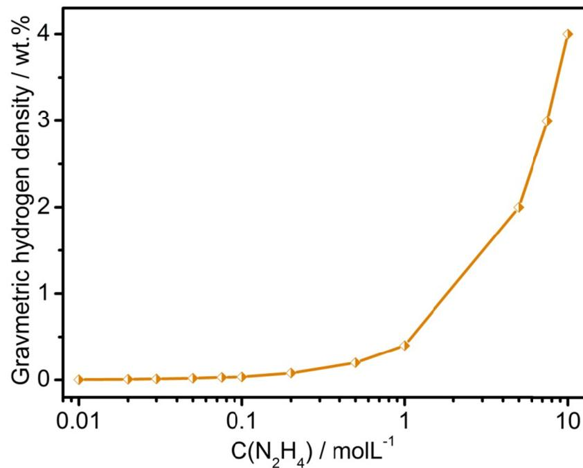
**Figure S41.** Solution gravimetric hydrogen densities versus  $N_2H_4$  concentrations for the decomposition of  $N_2H_4$  over 0.297 mmol surface “clean”  $Rh_2Ni$  nanooctahedrons supported on 30mg carbon at 293 K.
