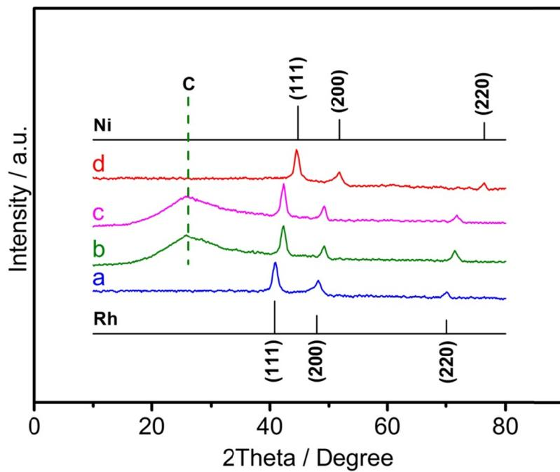
**Figure S43.** XRD profiles of (a) Rh nanoctahedrons; (b) the deactivated Rh<sub>2</sub>Ni nanoctahedrons/C; (c) the deactivated Rh<sub>2</sub>Ni nanoctahedrons /C after reactivation by solution plasma process; (d) Ni nanoctahedrons.
