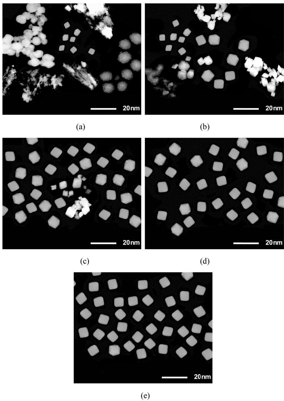
**Figure S22.** STEM images of  $\text{Rh}_2\text{Ni}$  synthesized by varying the amounts of 1-aminoheptadecane: (a) 0.01 mmol; (b) 0.025 mmol, (c) 0.05 mmol, (d) 0.075 mmol and (d) 0.1 mmol, respectively.
