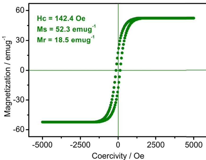
**Figure S46.** Hysteresis loop and magnetic properties of Ni nanoctahedrons.
