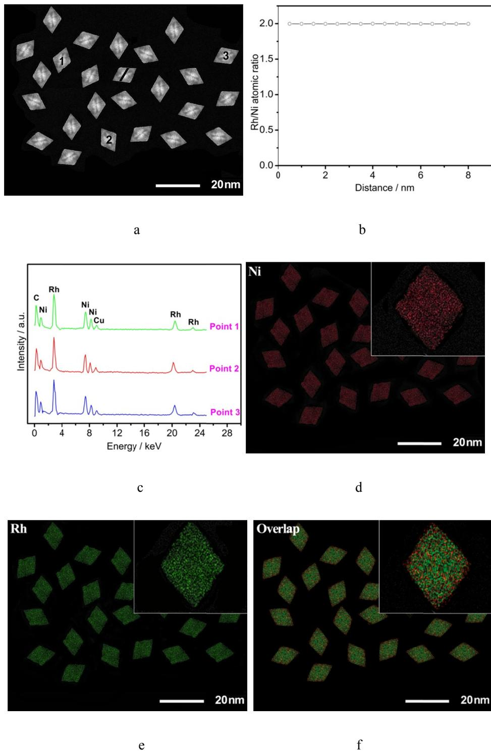
**Figure S3.** (a) The high-angle annular dark-field scanning transmission electron microscopy (HAADF-STEM); (b) Rh/Ni atomic ratios recorded along the white cross-sectional compositional line shown in (a); (c) the Energy-dispersive X-ray spectroscopy (EDS) at points 1-3 in (a); (d)-(f)the elemental maps of the as-prepared  $\text{Rh}_2\text{Ni}$  nano-octahedrons
