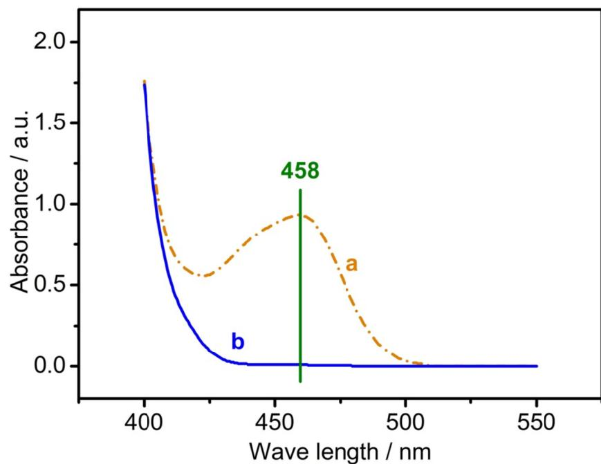
**Figure S30.** Typical UV-Vis spectra of hydrazine in aqueous solution (a) before and (b) after the completion of hydrazine decomposition reaction over surface “clean”  $\text{Rh}_2\text{Ni}$  or Rh or Ni NCs supported on carbon.
