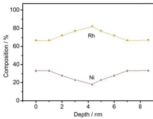
**Figure S25.** XPS Depth profile curves obtained using X-ray photoelectron spectroscopy of the as-prepared  $\text{Rh}_2\text{Ni}$  nanocubes in this work.
