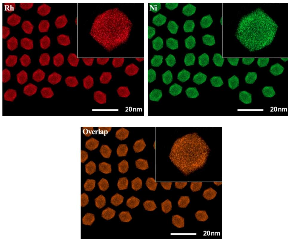
**Figure S21.** The elemental maps of the as-prepared  $\text{Rh}_2\text{Ni}$  trunked nanoctahedrons in this work.
