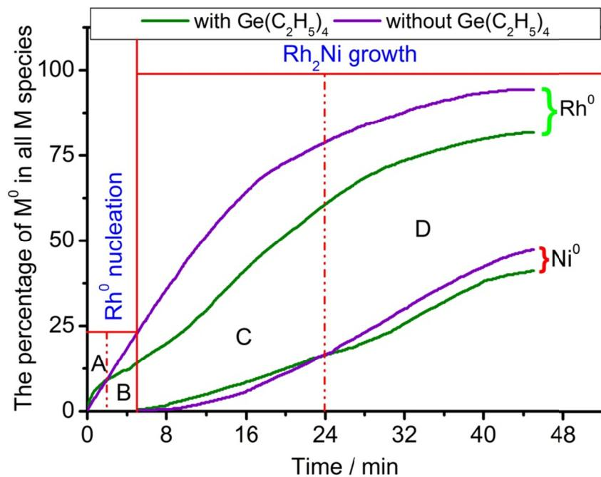
**Figure S26.** The  $\text{Rh}^0$  and  $\text{Ni}^0$  percentage in all Rh and Ni species obtained from the *in-situ* XPS measurement during the preparation process of  $\text{Rh}_2\text{Ni}$  NCs with or without the presence of  $\text{Ge}(\text{C}_2\text{H}_5)_4$ , respectively.
