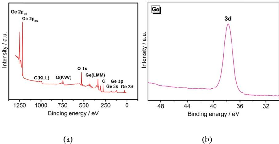
**Figure S10.** (a) Overall XPS spectrum and (b) Ge 3d spectrum for the reaction residue after the preparation of Rh<sub>2</sub>Ni nanoctahedrons.
