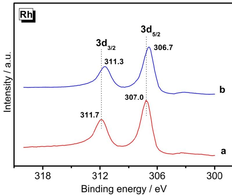
**Figure S5.** *In-situ* Rh3d XPS spectra of (a) Rh and (b) the as-prepared Rh<sub>2</sub>Ni nano-octahedrons in this work.
