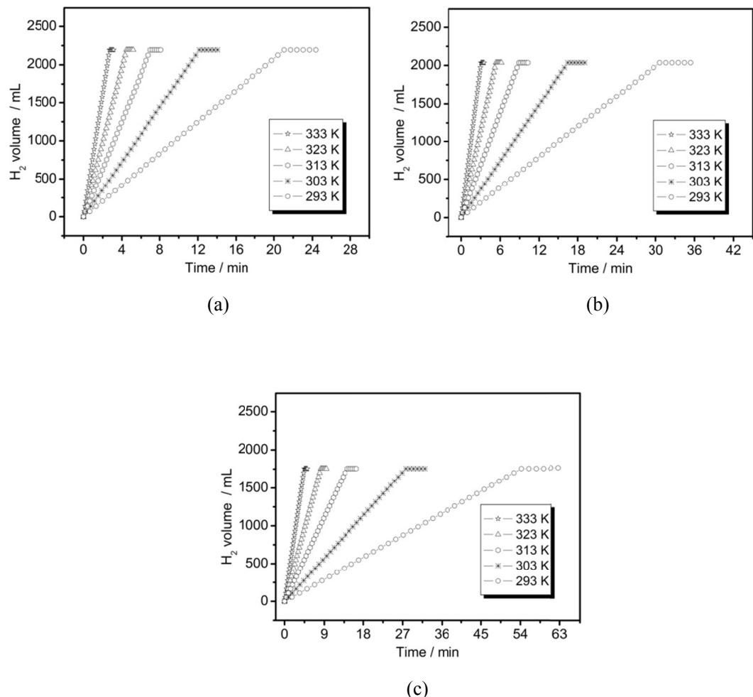
**Figure S32.** Plots of volume of hydrogen generated versus time during the hydrazine decomposition over 0.297 mmol of surface “clean” (a)  $Rh_2Ni$  nanooctahedrons, (b)  $Rh_2Ni$  truncated nanooctahedrons and (c)  $Rh_2Ni$  nanocubes supported on 30 mg carbon at different temperatures in the range 293 K–333 K ( $[N_2H_4] = 0.49 \text{ mol L}^{-1}$ ).
