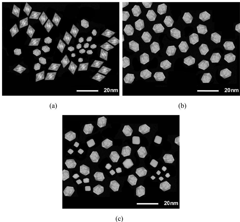
**Figure S16.** STEM images of  $\text{Rh}_2\text{Ni}$  synthesized by varying the molar ratio of margaric acid /1-aminoheptadecane : (a) 2, (b) 1, (c) 0.5, respectively.
