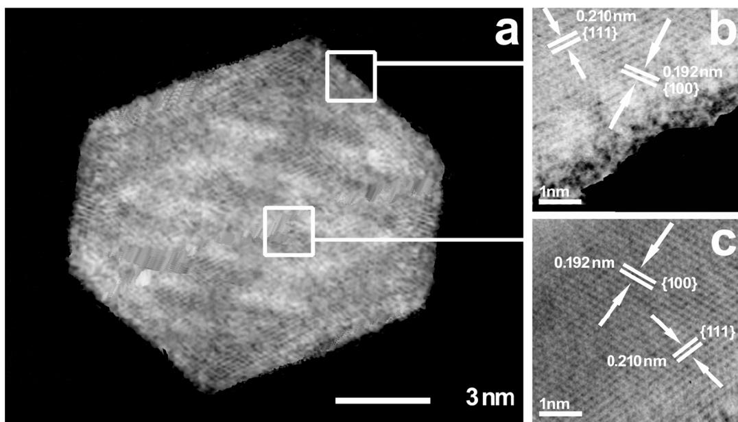
**Figure S18.** (a)The high resolution STEM (HR-STEM) image of a single  $\text{Rh}_2\text{Ni}$  trunked nanoctahedron; (b, c) Corresponding HR-STEM images of the regions marked in (a).
