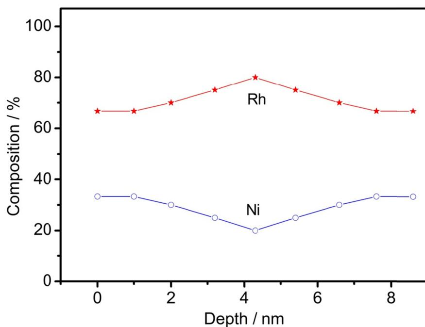
**Figure S7.** Depth profile curves obtained using X-ray photoelectron spectroscopy of the as-prepared  $\text{Rh}_2\text{Ni}$  nanoctahedrons in this work.
