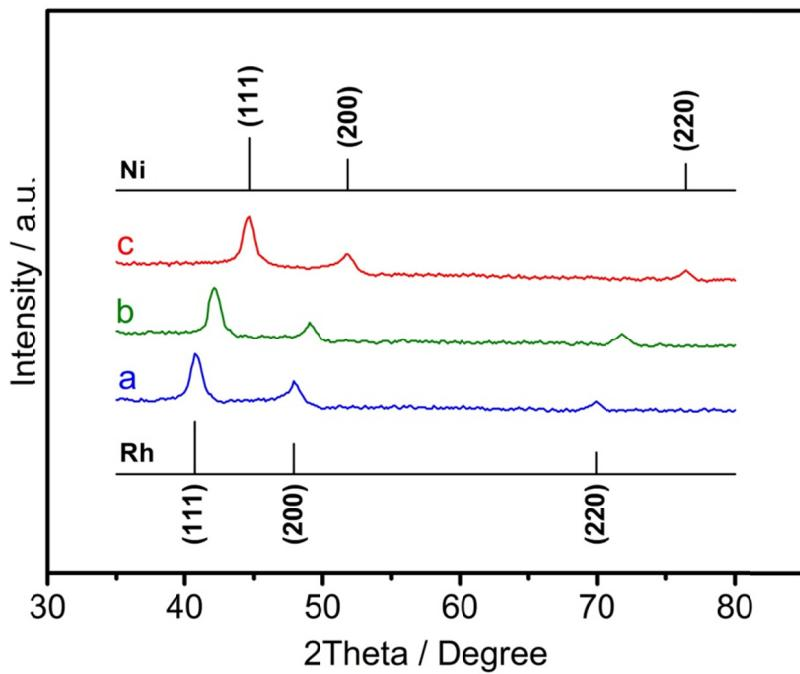
**Figure S2.** The XRD patterns of the as-prepared (a) Rh nano-octahedrons; (b)  $\text{Rh}_2\text{Ni}$  nano-octahedrons; (c) Ni nano-octahedrons.
