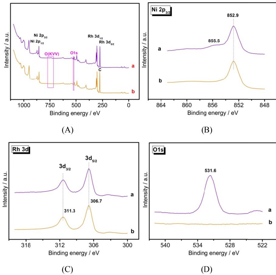
**Figure S44.** *in-situ* (A) Overall XPS spectra; (B) Ni2p<sub>3/2</sub> XPS spectra; (C) Rh 3d XPS spectra; and (D) O1s XPS spectra of the deactivated Rh<sub>2</sub>Ni nanoctahedrons /C (a) before reactivation and (b) after reactivation by solution plasma process.
