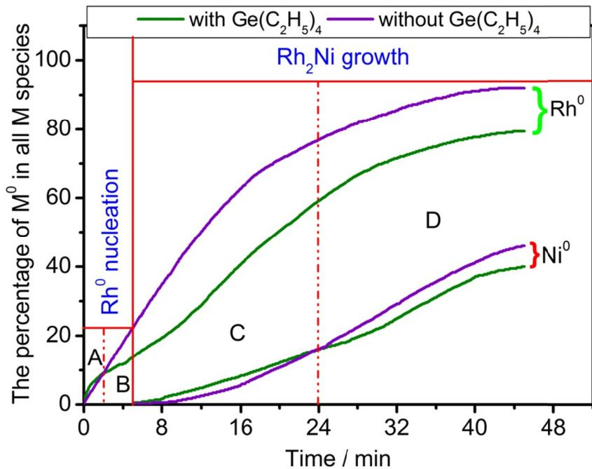
**Figure S9.** The  $\text{Rh}^0$  and  $\text{Ni}^0$  percentage in all Rh and Ni species obtained from the *in-situ* XPS measurement during the preparation process of  $\text{Rh}_2\text{Ni}$  NCs with or without the presence of  $\text{Ge}(\text{C}_2\text{H}_5)_4$ , respectively.
