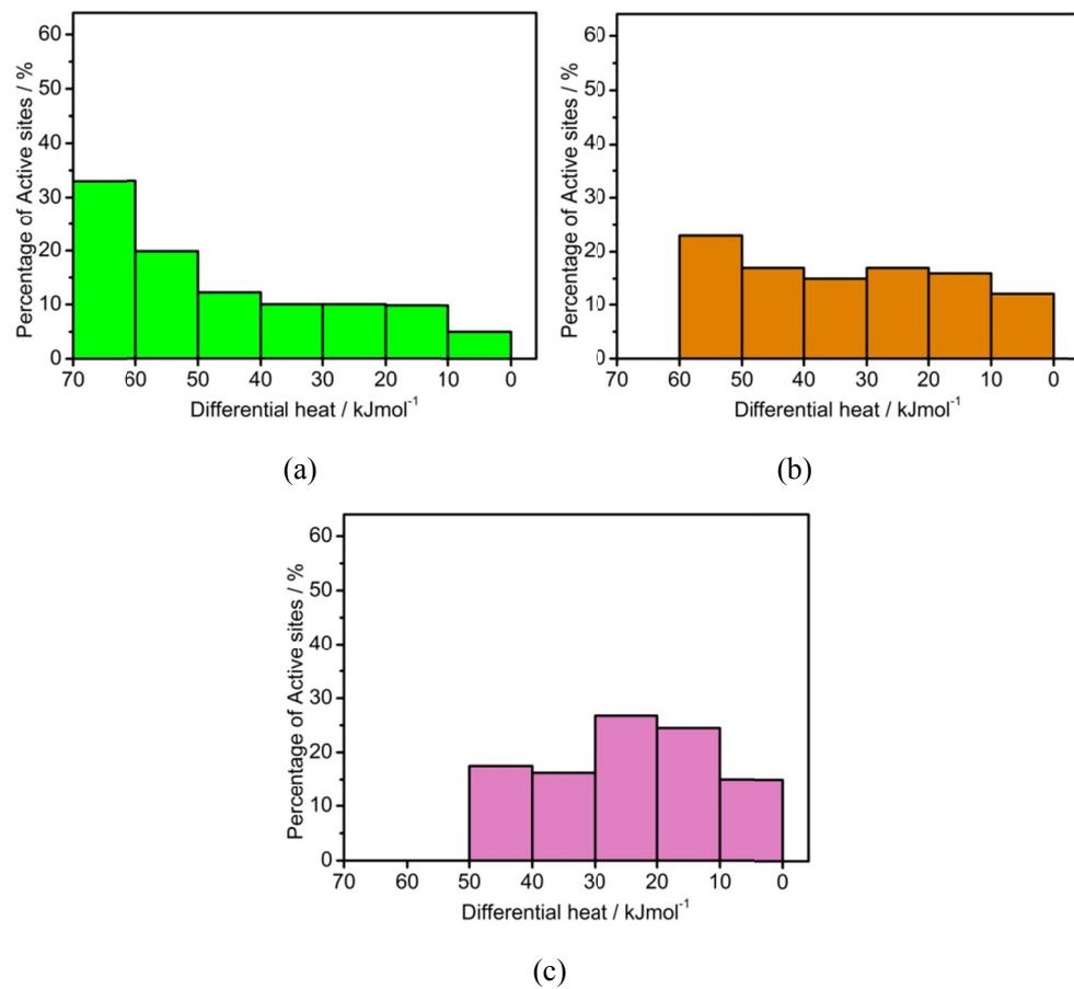
**Figure S34.** The differential heat of H<sub>2</sub> adsorption distribution histograms of surface “clean” (a) Rh<sub>2</sub>Ni nanocubes, (b) Rh<sub>2</sub>Ni truncated nanoctahedrons and (c) Rh<sub>2</sub>Ni nanoctahedrons.
