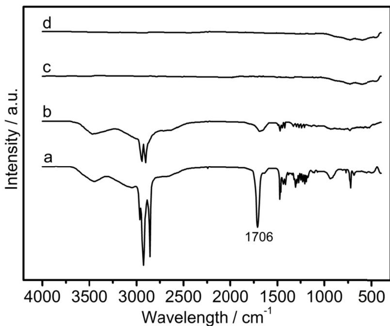
**Figure S12.** FT-IR spectra of (a) margaric acid; (b) the as-prepared  $\text{Rh}_2\text{Ni}$  nanoctahedrons only washed with water; (c) the as-prepared  $\text{Rh}_2\text{Ni}$  nanoctahedrons washed with ethanol; and (d) commercial  $\text{Rh}_2\text{Ni}$  NPs.
