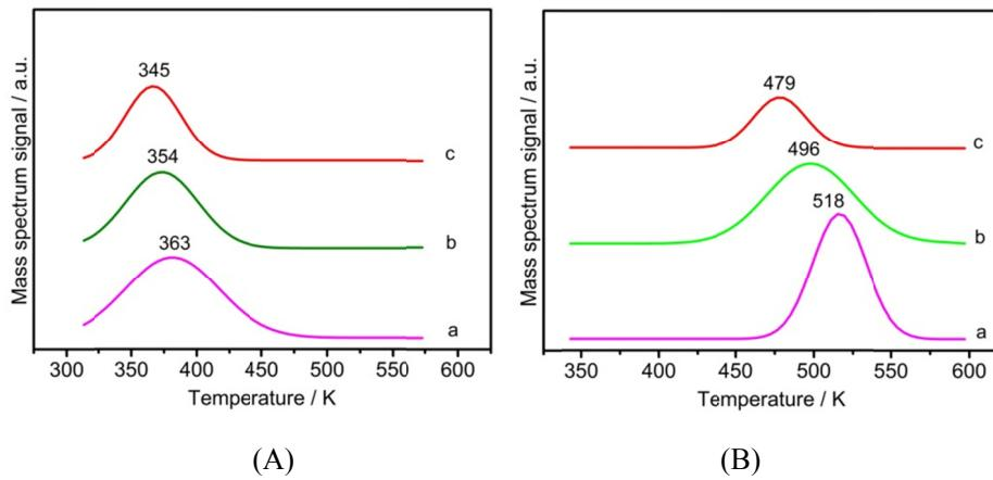
**Figure S36.** Mass spectra of NH<sub>3</sub> TPD-MS for (A) NH<sub>3</sub> desorption signal and (B) N<sub>2</sub> desorption signal for surface “clean” (a) Rh<sub>2</sub>Ni nanocubes, (b) Rh<sub>2</sub>Ni truncated nanoctahedrons and (c) Rh<sub>2</sub>Ni nanoctahedrons.
