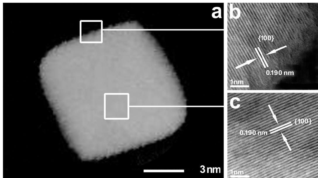
**Figure S24.** (a)The high resolution STEM (HR-STEM) image of a single Rh<sub>2</sub>Ni nanocube; (b, c) Corresponding HR-STEM images of the regions marked in (a).
