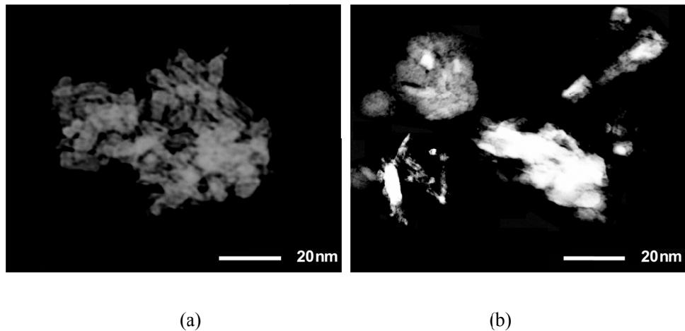
**Figure S8.** STEM images of the as-prepared  $\text{Rh}_2\text{Ni}$ : (a) without  $\text{Ge}(\text{C}_2\text{H}_5)_4$ ; (b) without margaric acid
