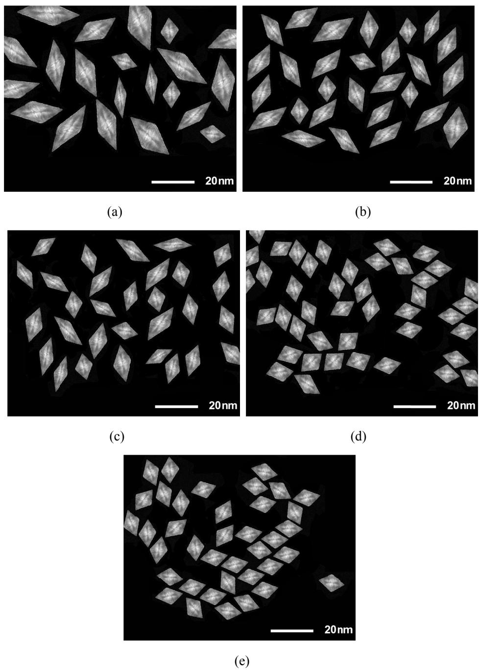
**Figure S15.** STEM images of the  $\text{Rh}_2\text{Ni}$  NCs synthesized by varying the molar ratio of  $\text{Ge}(\text{C}_2\text{H}_5)_4 / (\text{Rh} + \text{Ni})$  = (a) 1:40, (b) 1:30, (c) 1:20, (d) 1:10 and (e) 1:8, respectively.
