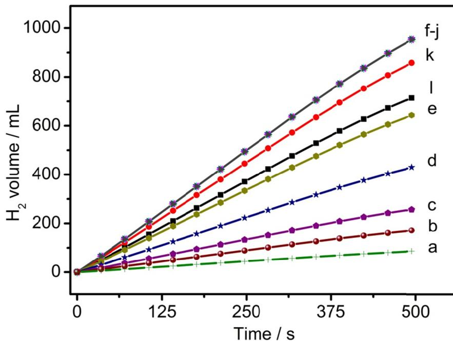
**Figure S39.** Hydrogen released from 20mL N<sub>2</sub>H<sub>4</sub> solution with different concentrations (a) 0.01, (b) 0.02, (c) 0.03, (d) 0.05, (e) 0.075, (f) 0.1, (g) 0.2, (h) 0.5, (i) 1, (j) 5, (k) 7.5 and(l) 10.0molL<sup>-1</sup> in the presence of 0.297 mmol surface “clean” Rh<sub>2</sub>Ni nanoctahedrons supported on 30mg carbon at 293 K.
