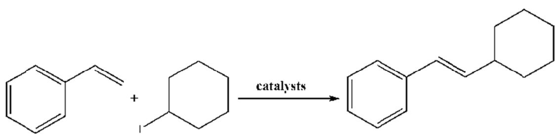
**Figure S47.** Heck-type coupling reaction between cyclohexyl iodide and styrene over catalysts.
