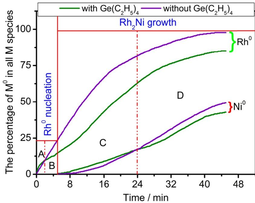
**Figure S20.** The  $\text{Rh}^0$  and  $\text{Ni}^0$  percentage in all Rh and Ni species obtained from the *in-situ* XPS measurement during the preparation process of  $\text{Rh}_2\text{Ni}$  NCs with or without the presence of  $\text{Ge}(\text{C}_2\text{H}_5)_4$ , respectively.
