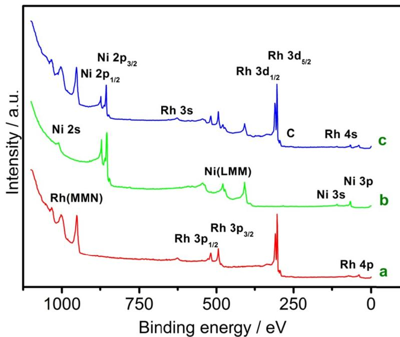
**Figure S4.** *In-situ* overall XPS spectra of (a) Rh, (b) Ni and (c) the as-prepared Rh<sub>2</sub>Ni nano-octahedrons in this work.
