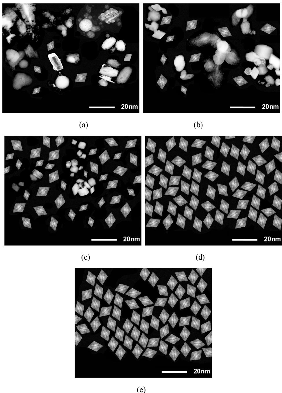
**Figure S13.** STEM images of  $\text{Rh}_2\text{Ni}$  synthesized by varying the amounts of margaric acid: (a) 0.01 mmol; (b) 0.025 mmol, (c) 0.05 mmol, (d) 0.075 mmol and (d) 0.1 mmol, respectively.
