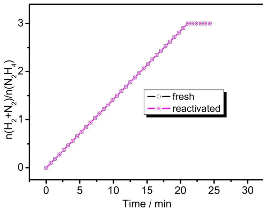
**Figure S45.** Time profiles for decomposition of hydrazine in aqueous solution (a) fresh and (b) reactivated Rh<sub>2</sub>Ni nanoctahedrons /C
