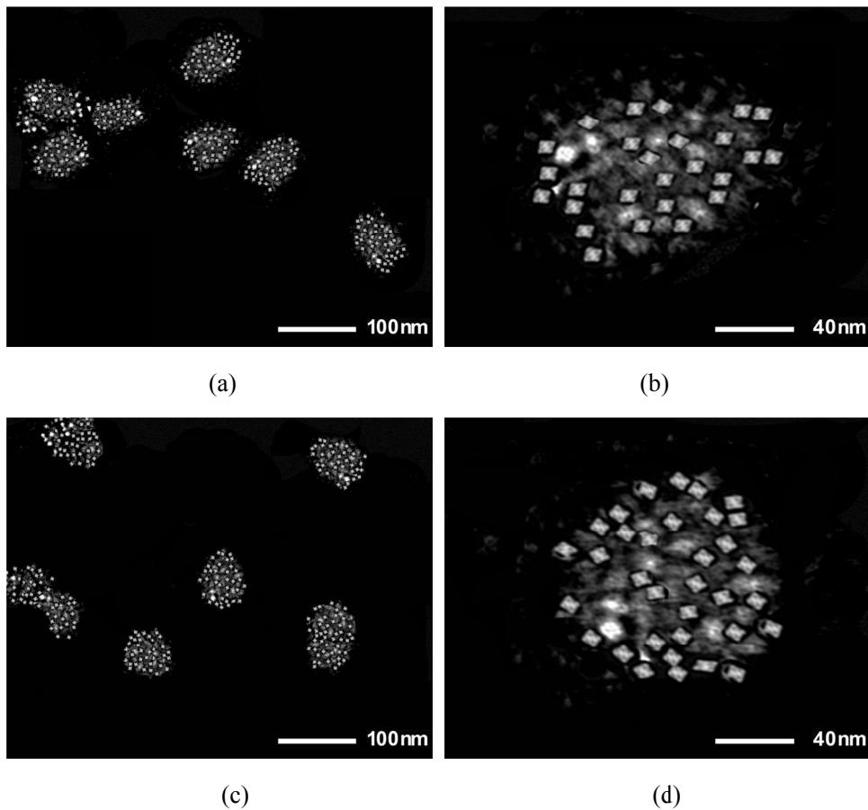
**Figure S42.** (a) STEM image and (b) enlarged STEM image of the deactivated  $\text{Rh}_2\text{Ni}$  nanoctahedrons/C; (c) STEM image and (d) enlarged STEM image of the deactivated  $\text{Rh}_2\text{Ni}$  nanoctahedrons/C after reactivation by solution plasma process.
