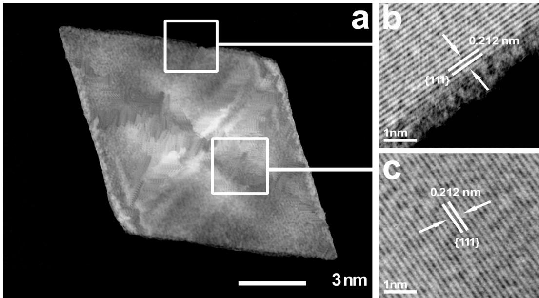
**Figure S1.** (a)The high resolution STEM (HR-STEM) image of a single  $\text{Rh}_2\text{Ni}$  nanoctahedron; (b, c) Corresponding HR-STEM images of the regions marked in (a).
