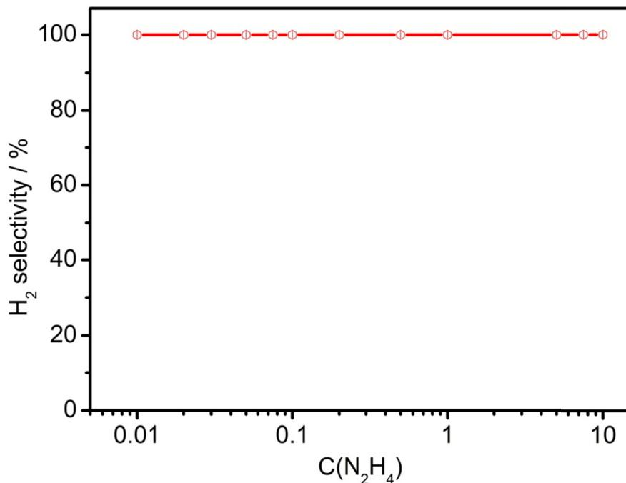
**Figure S38.** Hydrogen selectivity versus N<sub>2</sub>H<sub>4</sub> concentrations for the decomposition of N<sub>2</sub>H<sub>4</sub> over 0.297 mmol surface “clean” Rh<sub>2</sub>Ni nanoctahedrons supported on 30mg carbon at 293 K.
