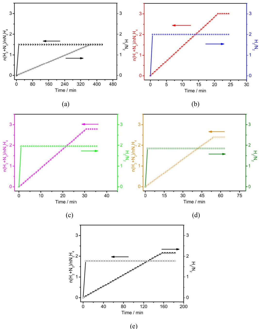
**Figure S29.** The  $n(\text{H}_2 + \text{N}_2)/n(\text{N}_2\text{H}_4)$  and  $\text{H}_2/\text{N}_2$  molar ratio versus time for 0.297 mmol of surface “clean” (a) Rh nanooctahedrons, (b) Rh<sub>2</sub>Ni nanooctahedrons, (c) Rh<sub>2</sub>Ni truncated nanooctahedrons, (d) Rh<sub>2</sub>Ni nanocubes and (e) Ni nanooctahedrons supported on 30 mg carbon during the decomposition of 100 mL of hydrazine in aqueous solution with a concentration of 0.49 mol L<sup>-1</sup> at 293 K.
