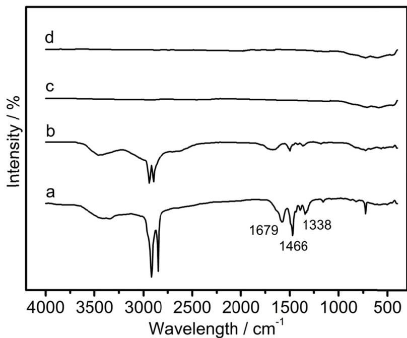
**Figure S23.** FT-IR spectra of (a) 1-aminoheptadecane; (b) the as-prepared Rh<sub>2</sub>Ni nanocubes only washed with water; (c) the as-prepared Rh<sub>2</sub>Ni nanocubes washed with ethanol; and (d) commercial Rh<sub>2</sub>Ni NPs.
