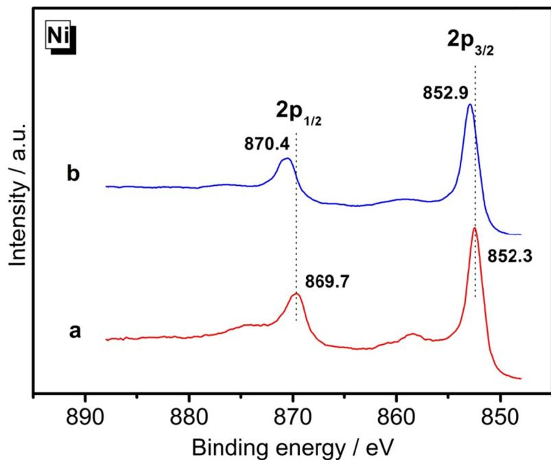
**Figure S6.** *In-situ* Ni2p XPS spectra of (a) Ni and (b) the as-prepared  $\text{Rh}_2\text{Ni}$  nanoctahedrons in this work.
