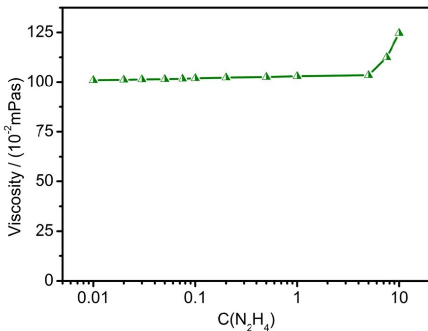
**Figure S40.** Viscosity versus  $N_2H_4$  concentrations at 293 K.
