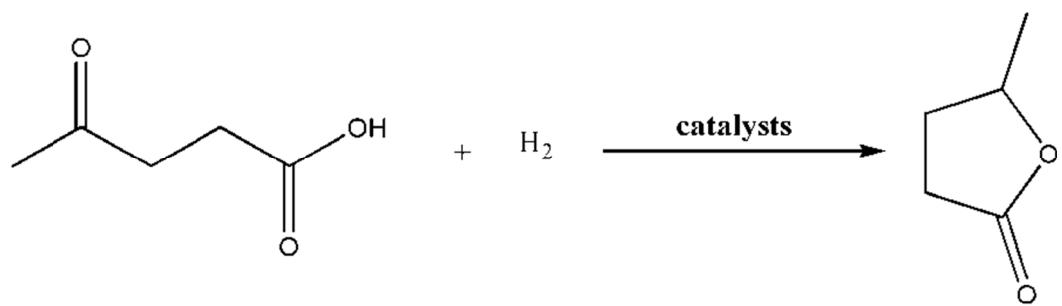
**Figure S49.** Hydrogenation of LA to GAL over catalysts
