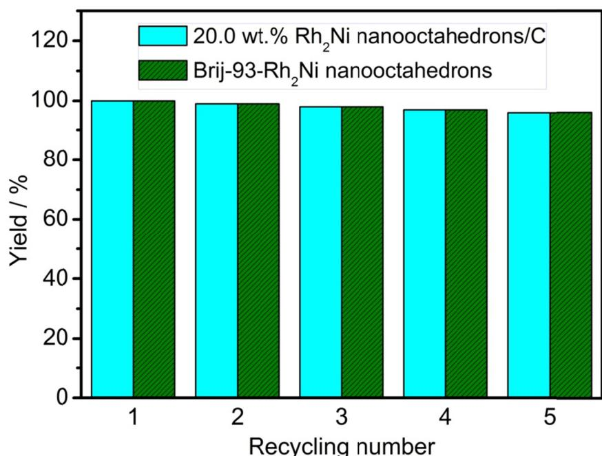
**Figure S50.** Recycling tests of 20.0 wt.%  $Rh_2Ni$  nanoctahedrons/C and Brij-93- $Rh_2Ni$  nanoctahedrons for LA hydrogenation to GAL. Reaction conditions: catalyst containing 10 mg of  $Rh_2Ni$  nanoctahedrons, 20 mmol of LA, 50 mL of n-dodecane,  $P_{H_2} = 4.2$  MPa  $H_2$ ,  $T = 413$  K, reaction time = 2 h, stirring rate = 1100 rpm.
