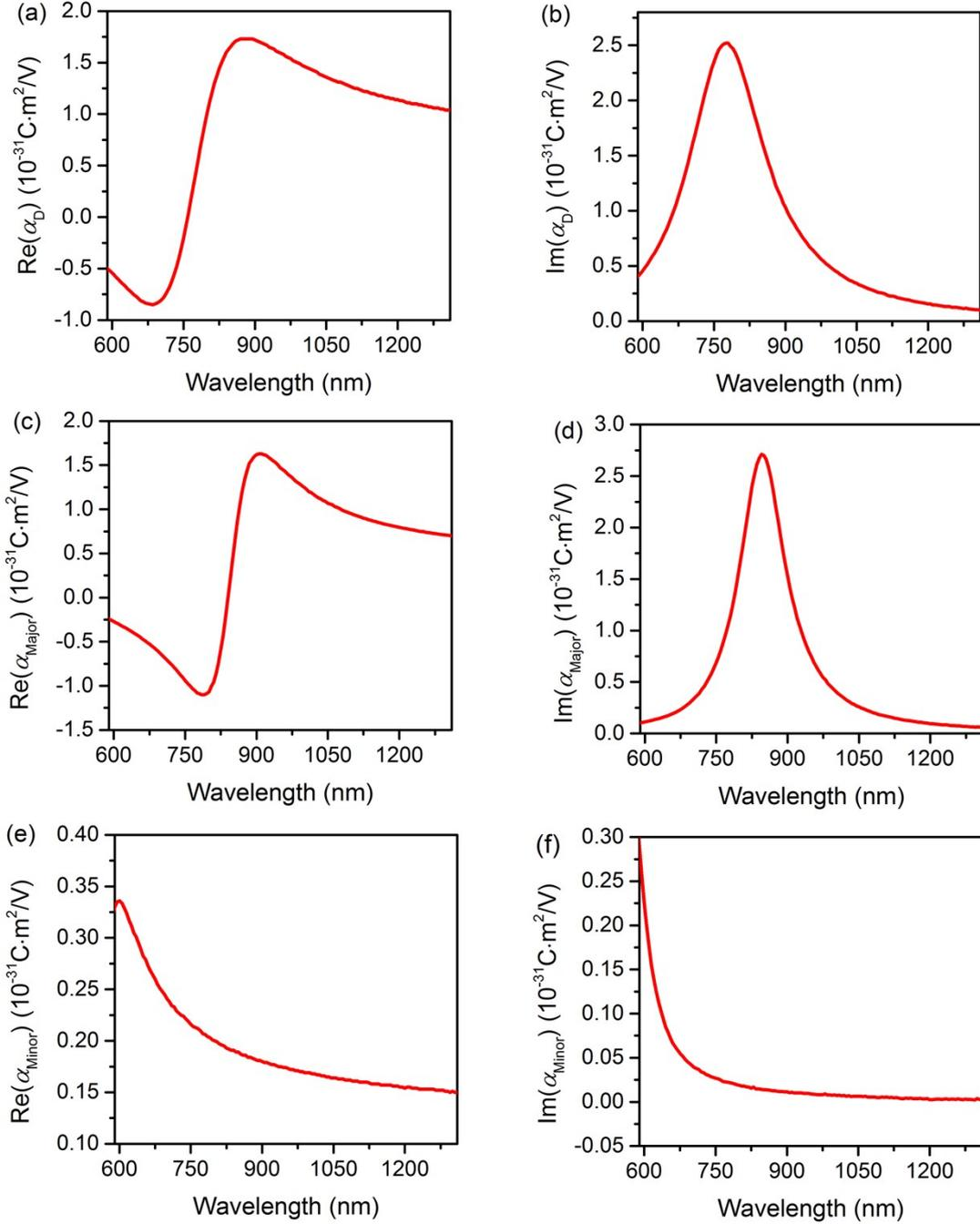
The FEM calculated real and imaginary part of the polarizabilities of the disk (a-b), the major axis of the ellipse (c-d) and the minor axis of the ellipse (e-f).
