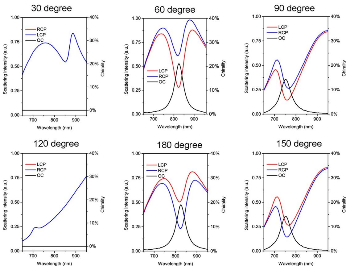
**Fig. S3** FEM simulations for the scattering cross section of chiral oligomers with different surrounding ellipse rotation angle. All of the main spectral features have a good agreement with the experimental results, and the difference between the experiment and simulations possibly is induced by the sample nanofabrication..
