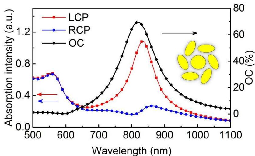
**Fig. S1** The absorption cross section of chiral Fano oligomers calculated by FEM simulation under LCP (red line) and RCP (blue line).
