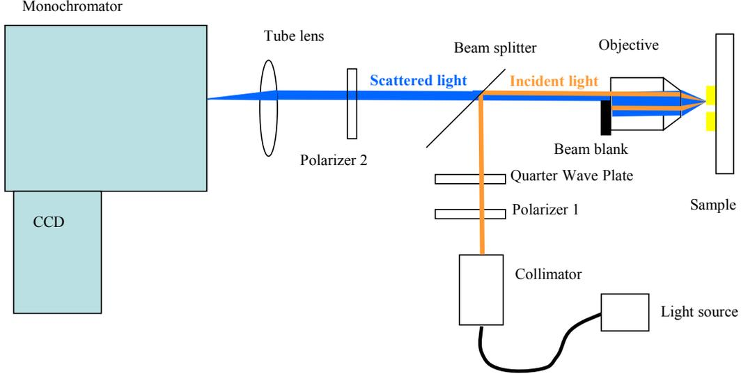
Schematic view of near-normal incident dark-field optical microscope.
