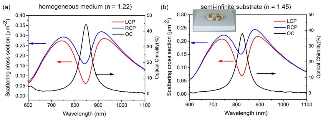
**Fig. S2** The FEM simulated scattering cross section of chiral Fano oligomers (a) embedded in homogeneous medium ( $n = 1.22$ ) and (b) on semi-infinite substrate ( $n = 1.45$ ) under LCP (red line) and RCP (blue line).
