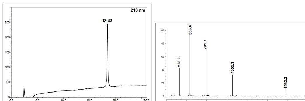
**Figure S1** RP-HPLC and ESI-MS traces of purified peptide **5**; column: Phenomenex Gemini C18 (5 $\mu$  110Å, 4.6 x 150mm); gradient: 0-1min, 1%B then 1%B to 51%B over 25 min., eluting at 1mL/min.,  $R_t$  18.48 min.
