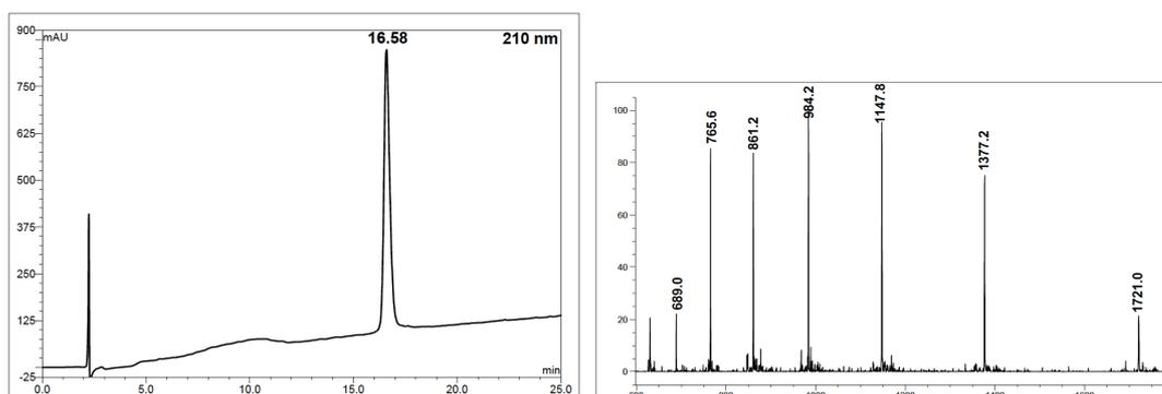
**Figure S8** RP-HPLC and ESI-MS traces of purified peptide **12**; column: Dionex Acclaim C18 (4.6 x 150mm); gradient: 0-1min, 1%B then 1%B to 61%B over 25 min., eluting at 1mL/min.;  $R_t$  16.58 min.
