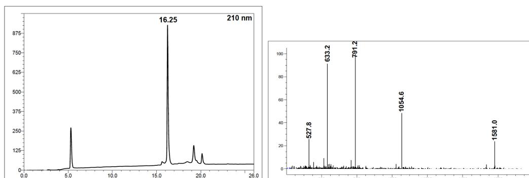
**Figure S2** RP-HPLC and ESI-MS traces showing conversion to disulfide **6**; column: Phenomenex Gemini C18 (5 $\mu$  110Å, 4.6 x 150mm); gradient: 0-1min, 1%B then 1%B to 51%B over 25 min., eluting at 1mL/min.,  $R_t$  16.25 min.
