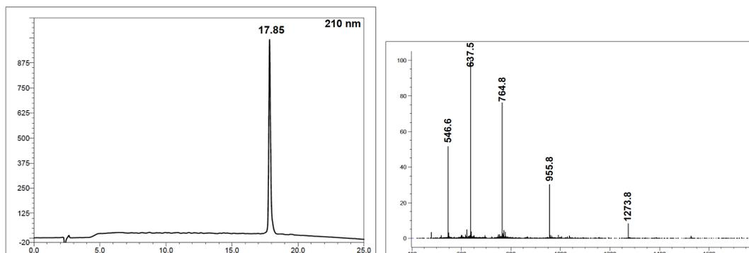
**Figure S3** RP-HPLC and ESI-MS traces of purified peptide **7**; column: Dionex Acclaim C18 (4.6 x 150mm); gradient: 0-1min, 1%B then 1%B to 61%B over 25 min., eluting at 1mL/min.;  $R_t$  17.85 min.
