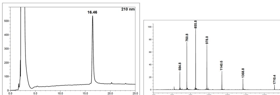
**Figure S7** RP-HPLC and ESI-MS traces of purified peptide **11**; column: Dionex Acclaim C18 (4.6 x 150mm); gradient: 0-1min, 1%B then 1%B to 61%B over 25 min., eluting at 1mL/min.;  $R_t$  16.46 min.
