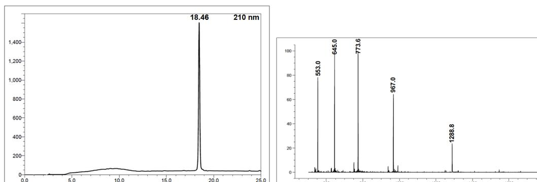
**Figure S4** RP-HPLC and ESI-MS traces of purified peptide **8**; column: Dionex Acclaim C18 (4.6 x 150mm); gradient: 0-1min, 1%B then 1%B to 61%B over 25 min., eluting at 1mL/min.;  $R_t$  18.46 min.
