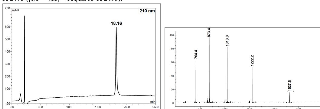
**Figure S10** RP-HPLC and ESI-MS traces of purified peptide **4**; column: Dionex Acclaim C18 (4.6 x 150mm); gradient: 0-1min, 1%B then 1%B to 61%B over 25 min., eluting at 1mL/min.;  $R_t$  18.16 min.
