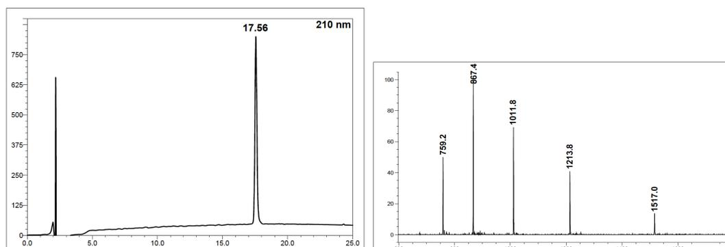
**Figure S9** RP-HPLC and ESI-MS traces of purified peptide **3**; column: Dionex Acclaim C18 (4.6 x 150mm); gradient: 0-1min, 1%B then 1%B to 61%B over 25 min., eluting at 1mL/min.;  $R_t$  17.56 min.
