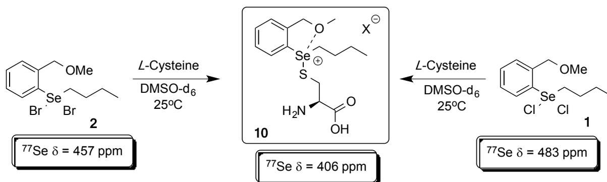
**Scheme S1:** Plausible product of reaction of organoselenenanes **2** or **1** with *L*-cysteine monitored by  $^{77}\text{Se}$  NMR in  $\text{DMSO-d}_6$  at 25  $^\circ\text{C}$ .
