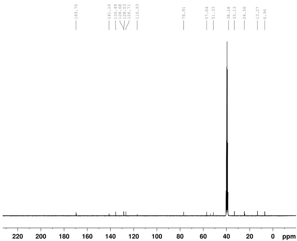
**Figure S13:**  $^{13}\text{C}$  NMR spectrum of organotellurane **8** in  $\text{DMSO-d}_6$  at 25 °C
