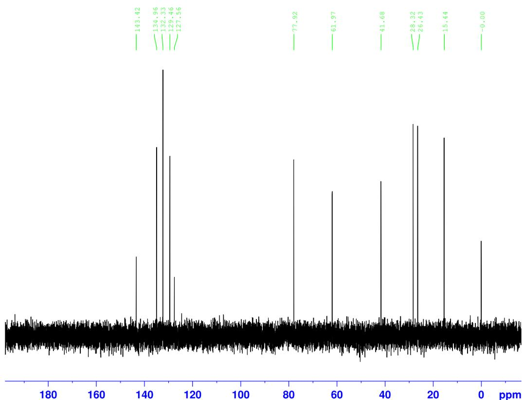
**Figure S4:**  $^{13}\text{C}$  NMR spectrum of organotellurane **5** in  $\text{D}_2\text{O}$  at 25 °C
