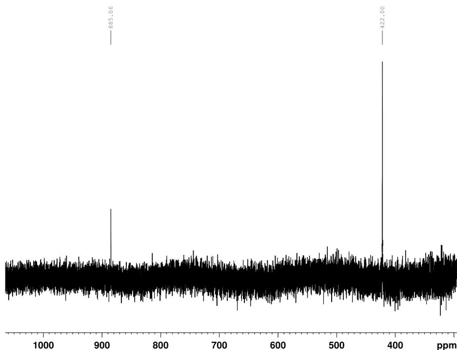
**Figure S1:**  $^{125}\text{Te}$  NMR spectrum of organotellurane **4** in  $\text{DMSO-d}_6$  at 25  $^\circ\text{C}$
