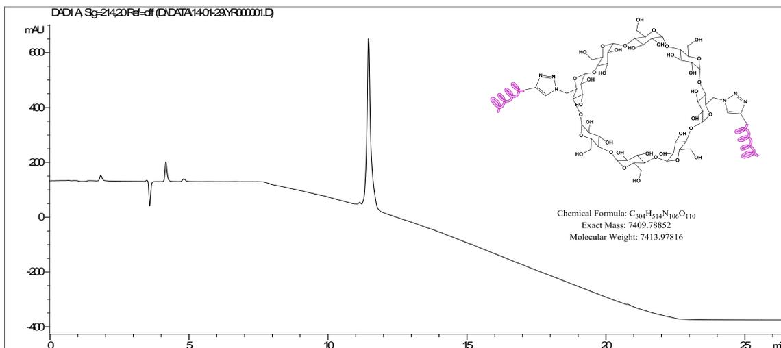
Figure S15: RP-HPLC Chromatogram of pure compound **10** (Jupiter C4, 300Å column using a gradient from 0 to 100 %  $CH_3CN$  in 15 minutes)
