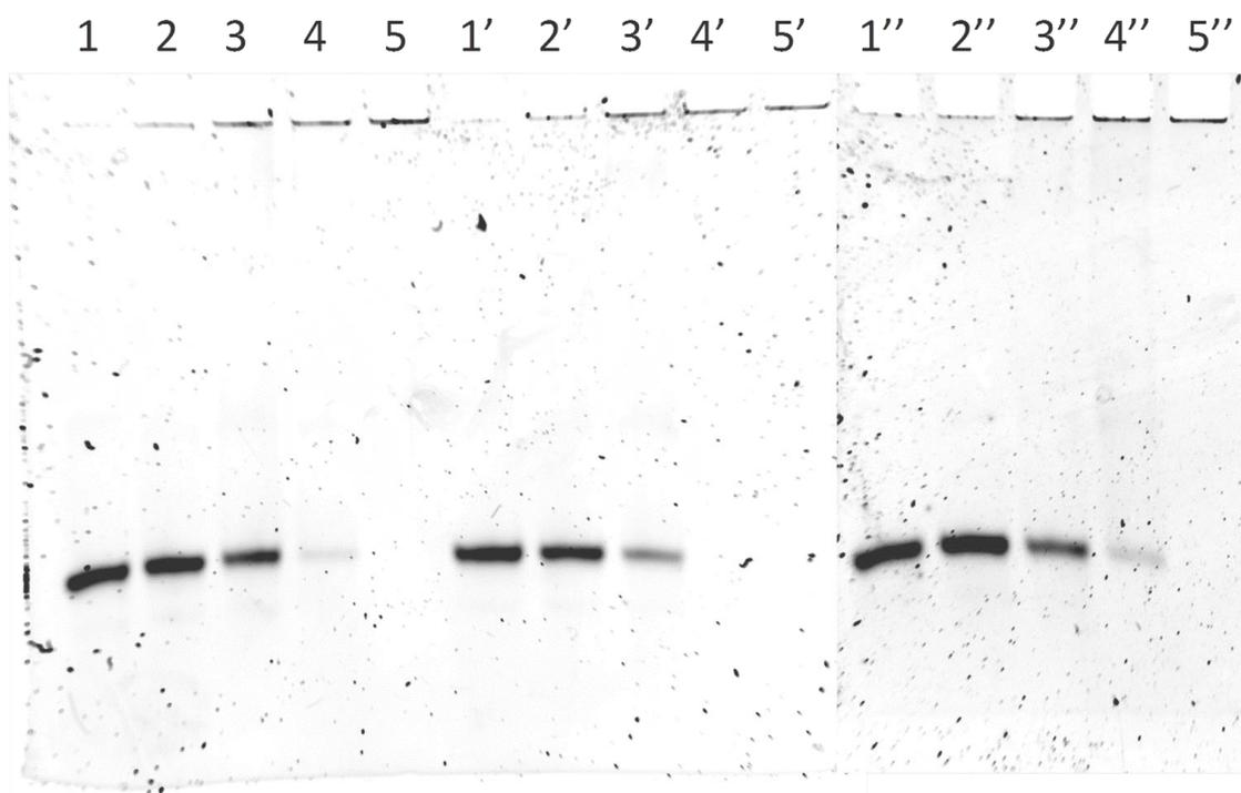
Figure S23: EMSA titration of the dipodal peptidocyclodextrin conjugates to the random sequence: Concentrations: 0.167 µM dsDNA; Lanes 1-5: 0, 0.167, 0.501, 0.668, 1.67 µM. Lanes 1-5 for compound **8** (alfa conjugate). Lanes 1'-5' compound **9** (beta conjugate). Lanes 1''-5'' Compound **10** (gamma conjugate).
