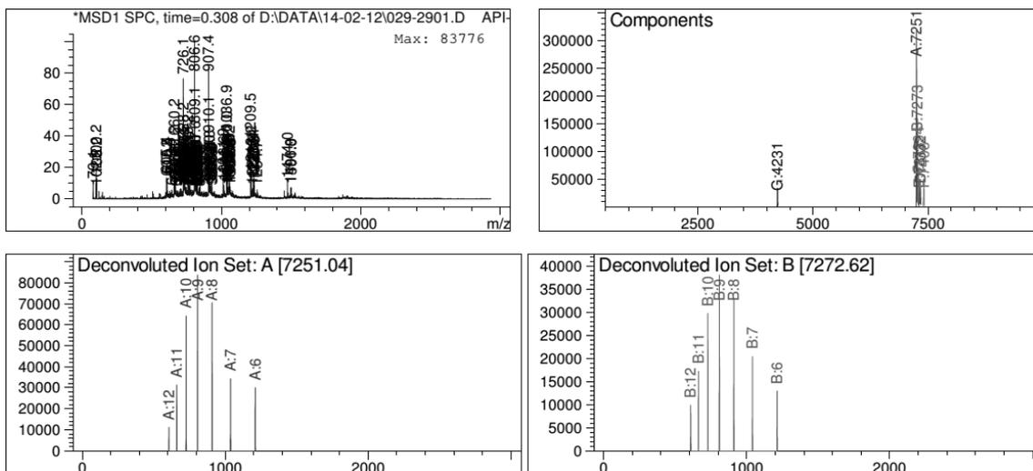
Figure S12: ESI-MS of compound **9**. Calcd. E.M. = 7247.74,  $M + Na^+$  = 7270.74 and deconvoluted masses found 7251.04 and 7272.62 + other minor impurities.
