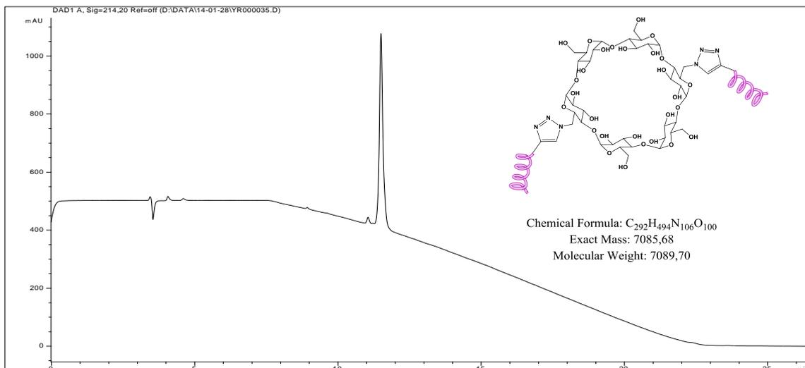
Figure S7: RP-HPLC Chromatogram of pure compound **8** (C4, 300Å column using a gradient from 0 to 100 % CH<sub>3</sub>CN in 15 minutes)
