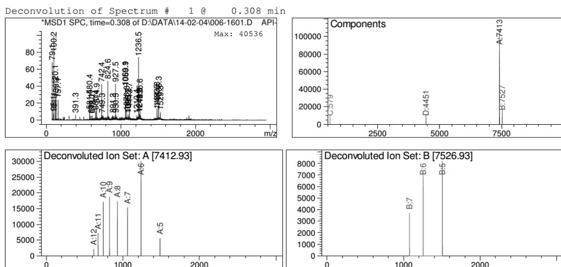
Figure S16: ESI-MS of compound **10**. Calcd. E.M. = 7409.79,  $M + 114.02$  (TFA salt) = 7523.81 and deconvoluted masses found 7412.93 and 7526.93 + other minor impurities.
