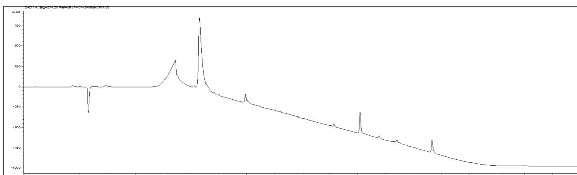
Figure S9: HPLC trace of compound **8** from LC-MS (0-100% ACN in 6 min on Kinetex C18 100 Å, 150 x 2.1 mm, 2.6 μm, at 35 °C)
