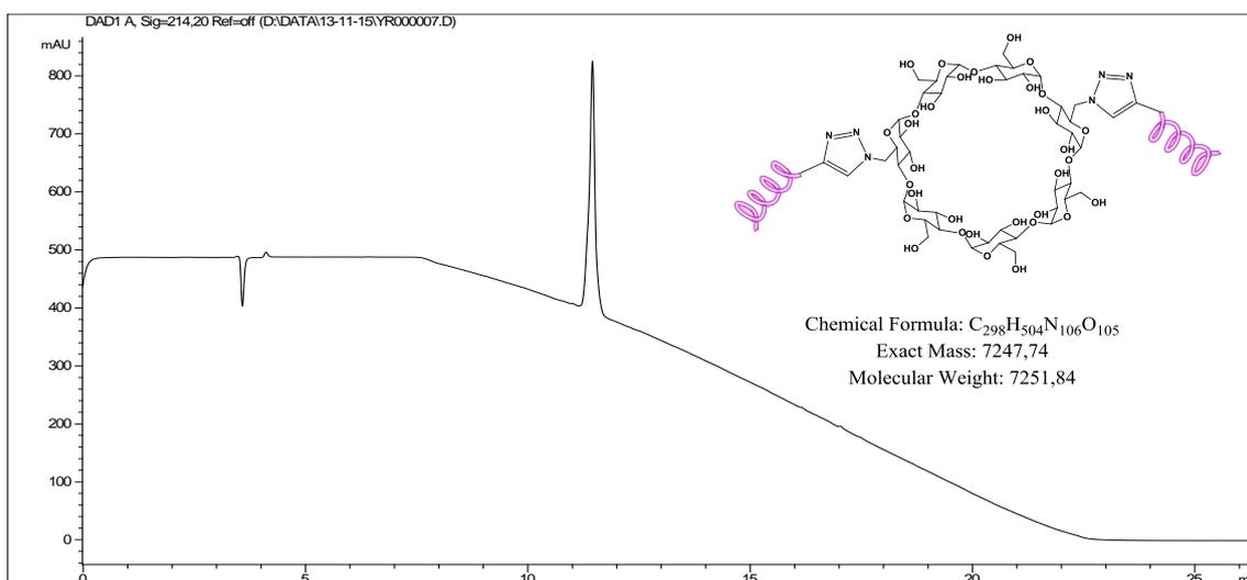
Figure S11: RP-HPLC Chromatogram of pure compound **9** (Jupiter C4, 300Å column using a gradient from 0 to 100 %  $CH_3CN$  in 15 minutes)
