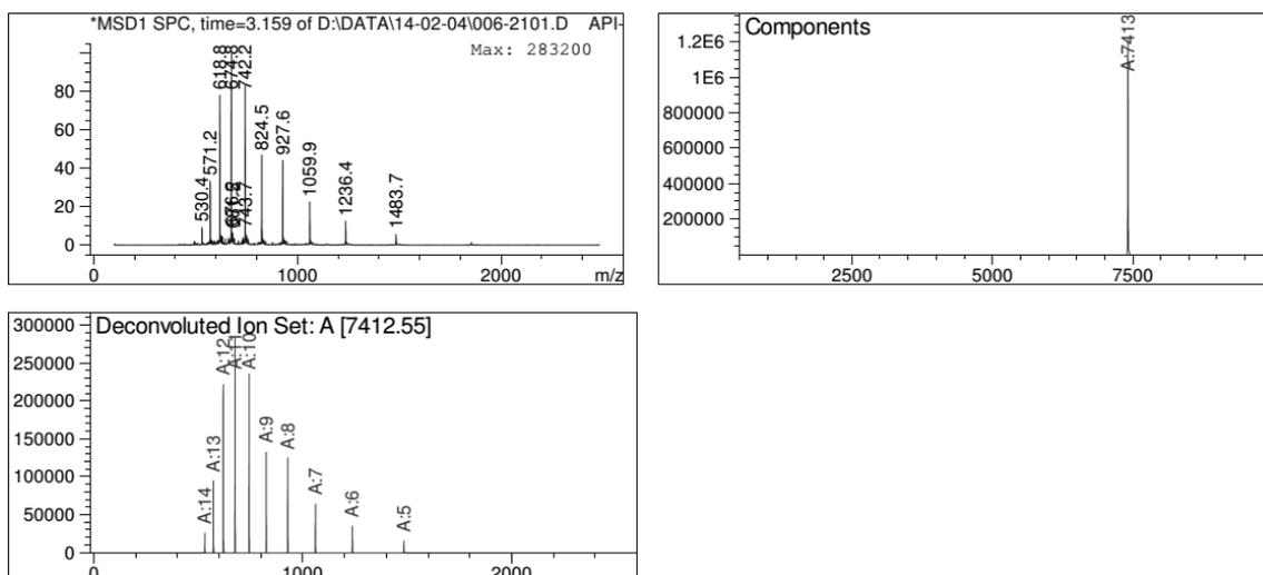
Figure S18: ESI-MS from LC-MS at r.t. = 3.159 min. Cacl'd. E.M. = 7409.79 and deconvoluted mass found 7412.55
