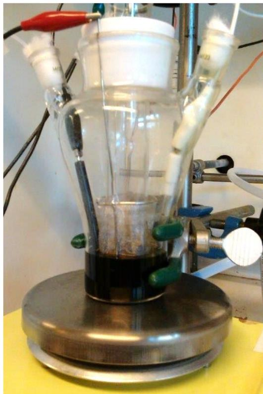
**Fig. S18** The electrochemical cell used for constant current oxidation of **11**. The dark color of the solution appeared upon oxidation.
