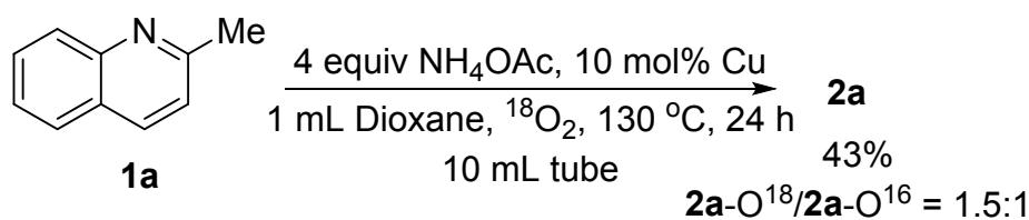
Under an  ${}^{18}\text{O}_2$  atmosphere (1 atm), **1a** (0.2 mmol),  $\text{NH}_4\text{OAc}$  (0.8 mmol, dried in vacuum), metallic Cu (0.02 mol) and dioxane (1.0 mL, dried by  $\text{CaH}_2$ ) were placed into a glass tube (10 mL) and sealed. The mixture was heated at 130 °C for 24 hours. The yield and ratio were determined by GC and GC-MS.
