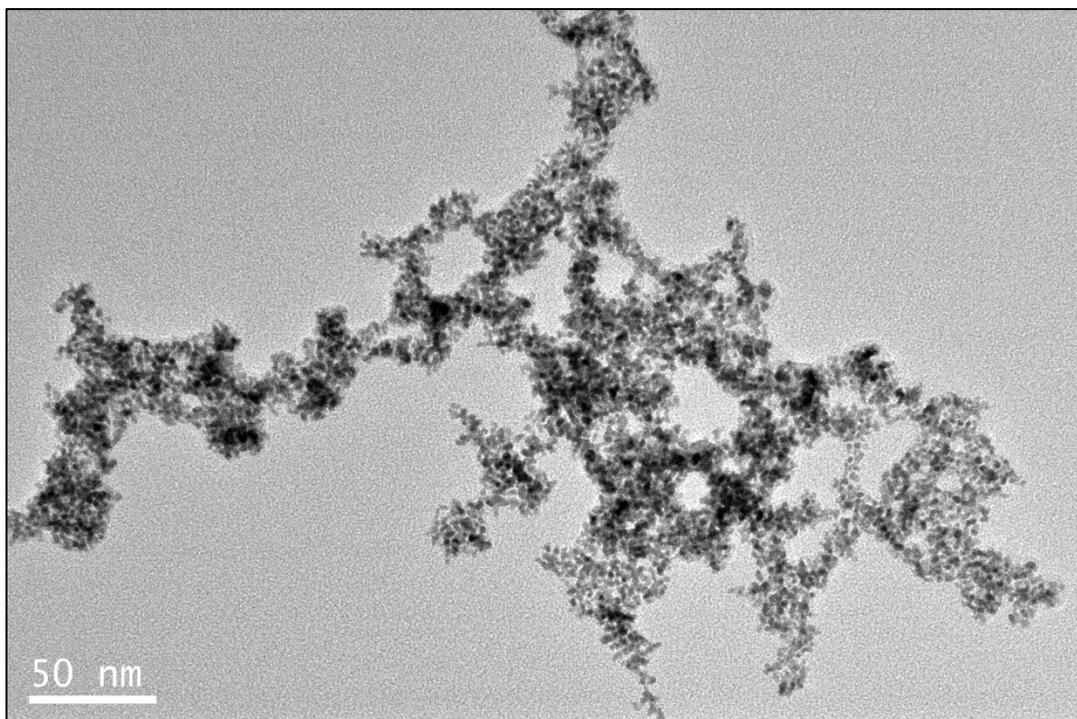
**Figure S8:** Low magnification TEM image of PtNPs-HALNN.
