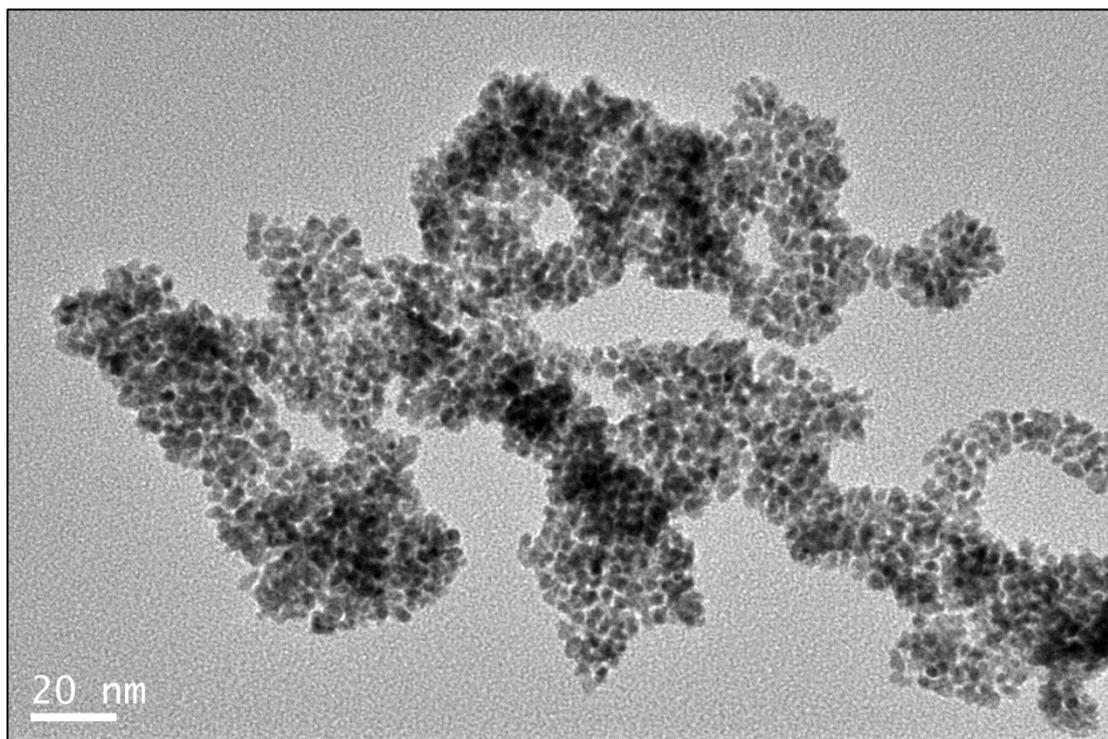
**Figure S13:** Low magnification TEM image of PtNPs-HALNNE<sub>6</sub>.
