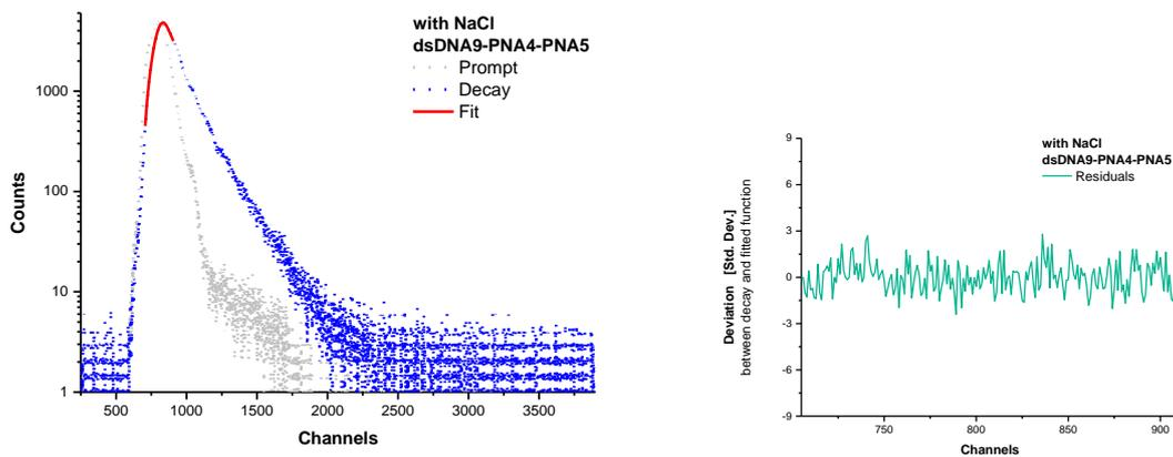
Scheme S158: Fluorescence lifetime decay of donor dye 4 (left) and residuals (right) of strand invasion complex dsDNA9 with 1.5 equivalents PNA4/PNA5 in presence of NaCl.
