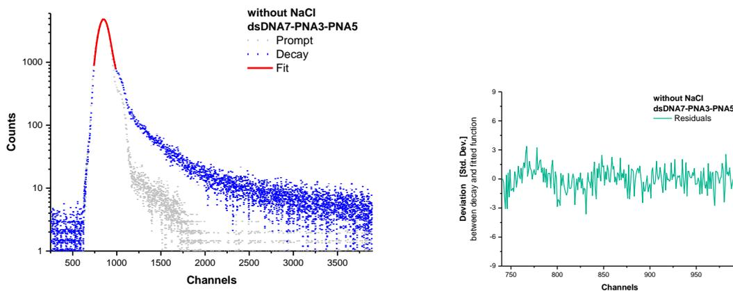
Scheme S149: Fluorescence lifetime decay of donor dye 1 (left) and residuals (right) of strand invasion complex dsDNA7 with 3.0 equivalents PNA3/PNA5 in absence of NaCl.
