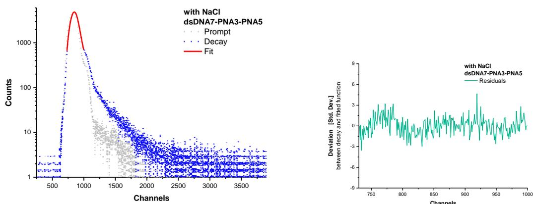
Scheme S143: Fluorescence lifetime decay of donor dye 1 (left) and residuals (right) of strand invasion complex dsDNA7 with 3.0 equivalents PNA3/PNA5 in presence of NaCl.
