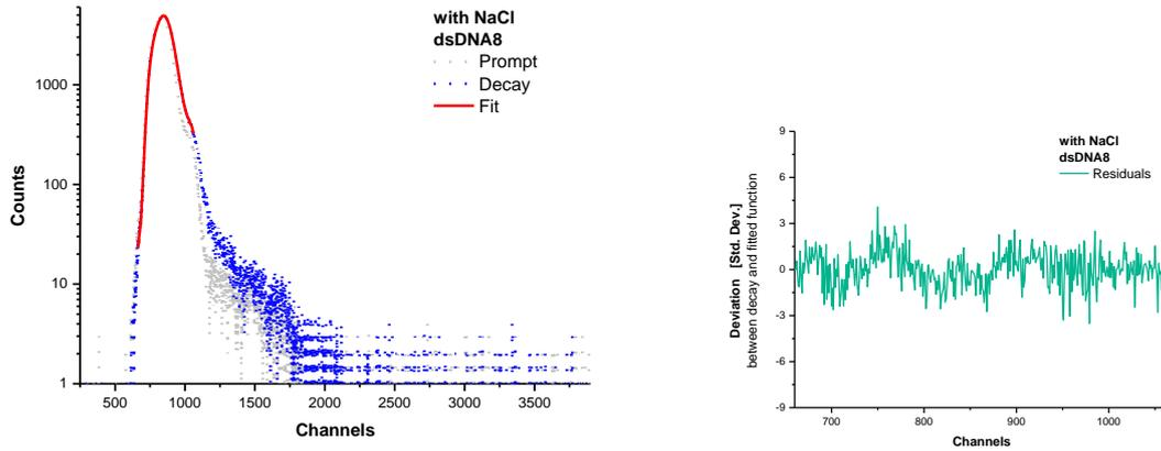
Scheme S145: Fluorescence lifetime decay of donor dye 1 (left) and residuals (right) of strand invasions dsDNA8 in presence of NaCl.
