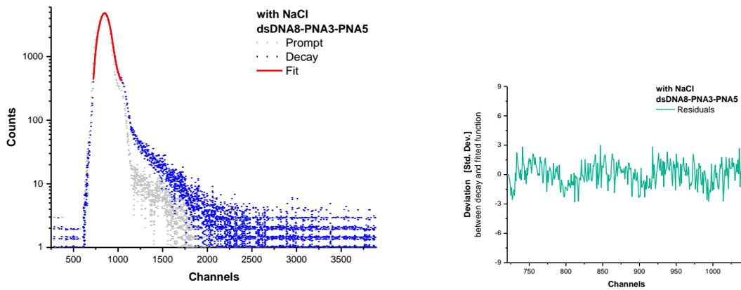
Scheme S146: Fluorescence lifetime decay of donor dye 1 (left) and residuals (right) of strand invasion complex dsDNA8 with 3.0 equivalents PNA3/PNA5 in presence of NaCl.
