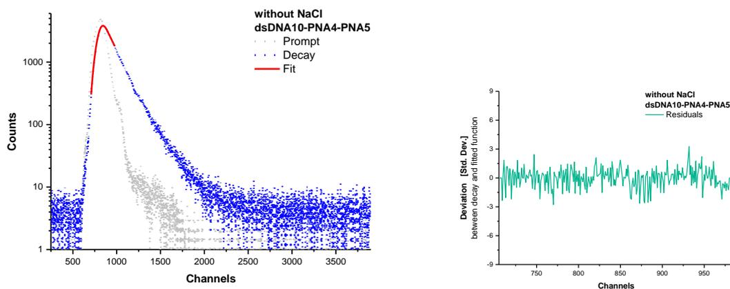
Scheme S167: Fluorescence lifetime decay of donor dye 4 (left) and residuals (right) of strand invasion complex dsDNA10 with 1.5 equivalents PNA4/PNA5 in absence of NaCl.
