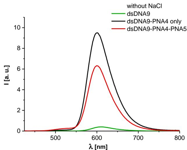
Scheme S128: Comparison of fluorescence spectra of final strand invasion measurement of dsDNA9-PNA4-PNA5 and dsDNA9-PNA4 in absence of NaCl, respectively.
