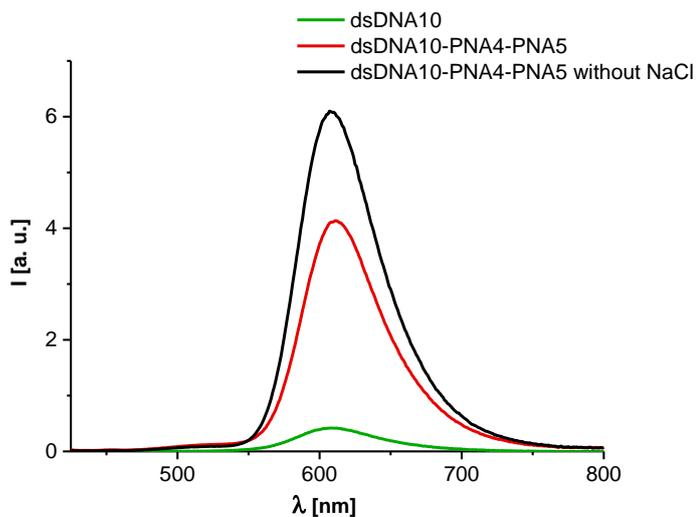
Scheme S133: Comparison of fluorescence spectra of final strand invasion measurement of dsDNA10-PNA4-PNA5 in presence and absence of NaCl, respectively.
