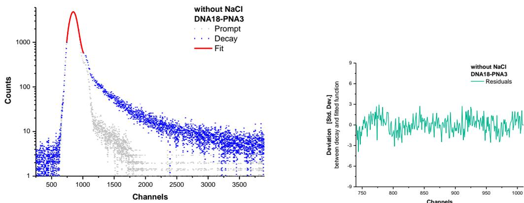
Scheme S153: Fluorescence lifetime decay of donor dye 1 (left) and residuals (right) of strand invasion compare solution with DNA18 and 3.0 equivalents PNA3 in absence of NaCl.
