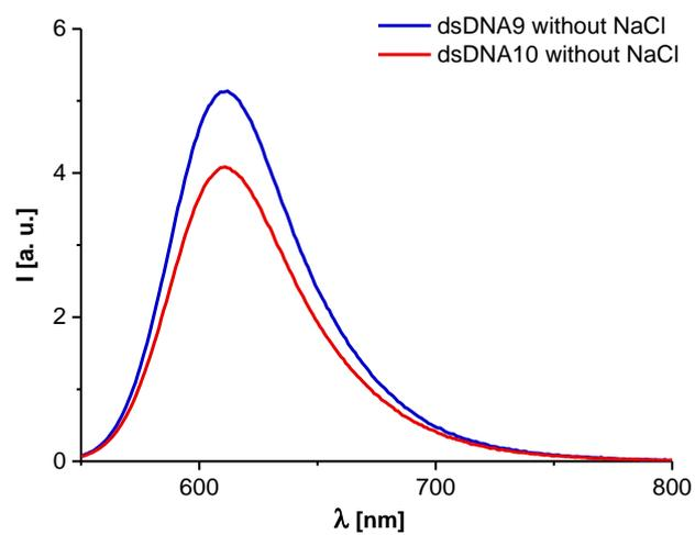
Scheme S139: Comparison of fluorescence spectra of dsDNA9 (dye 3 at 2' of adenosine) and dsDNA10 (dye 3 at 2' of uridine) in absence of NaCl, respectively.
