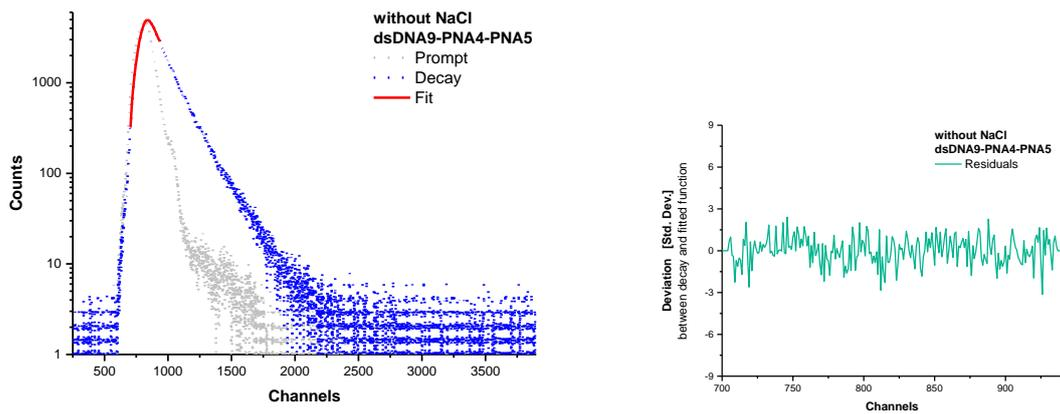
Scheme S164: Fluorescence lifetime decay of donor dye 4 (left) and residuals (right) of strand invasion complex dsDNA9 with 1.5 equivalents PNA4/PNA5 in absence of NaCl.
