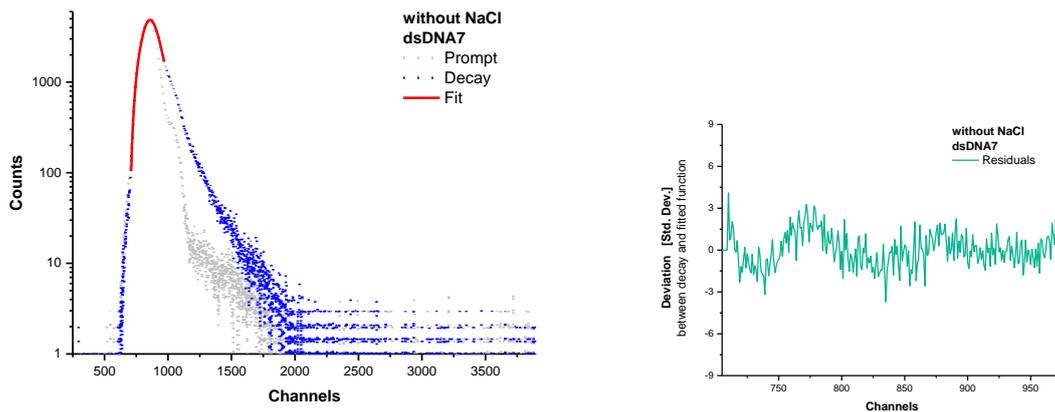
Scheme S148: Fluorescence lifetime decay of donor dye 1 (left) and residuals (right) of strand invasions dsDNA7 in absence of NaCl.
