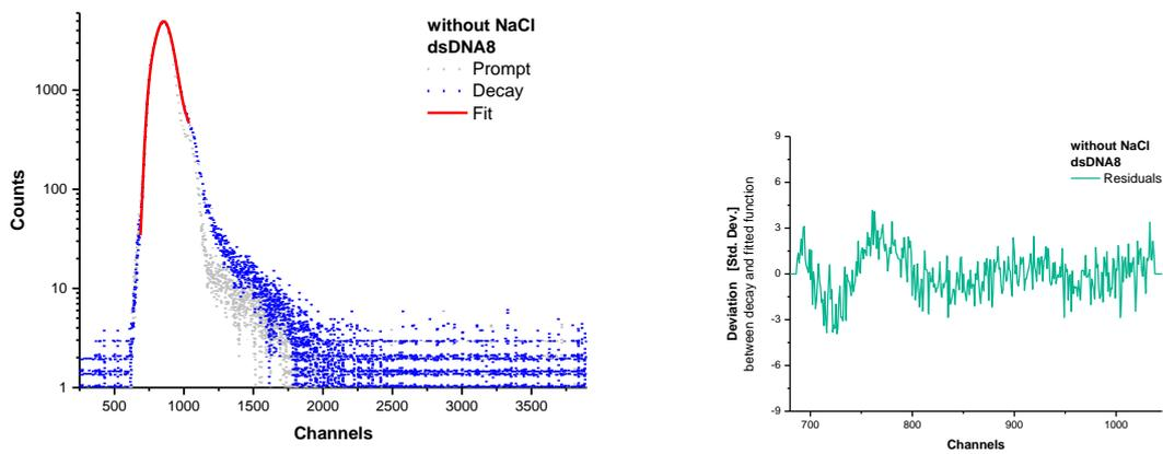
Scheme S151: Fluorescence lifetime decay of donor dye 1 (left) and residuals (right) of strand invasions dsDNA8 in absence of NaCl.
