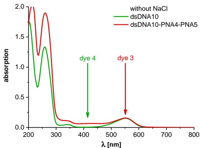
Scheme S131: Absorption spectra of final strand invasion measurement of dsDNA10-PNA4-PNA5 in absence of NaCl.
