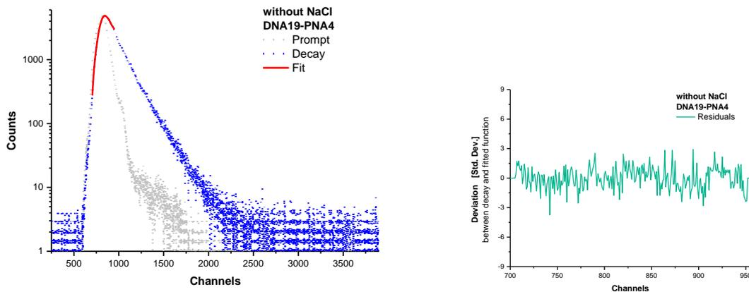
Scheme S166: Fluorescence lifetime decay of donor dye 4 (left) and residuals (right) of strand invasion compare solution with DNA19 and 1.5 equivalents PNA4 in absence of NaCl.
