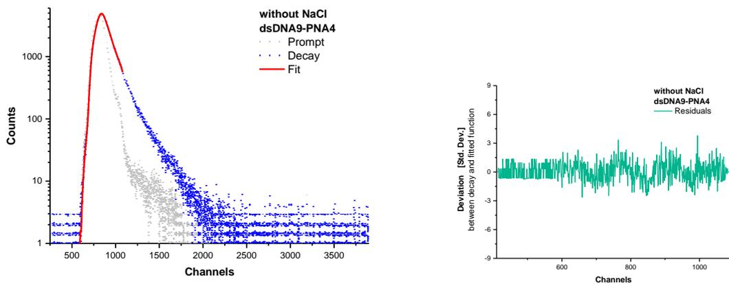
Scheme S165: Fluorescence lifetime decay of donor dye 4 (left) and residuals (right) of strand invasion complex dsDNA9 with 1.5 equivalents PNA4 in absence of NaCl.
