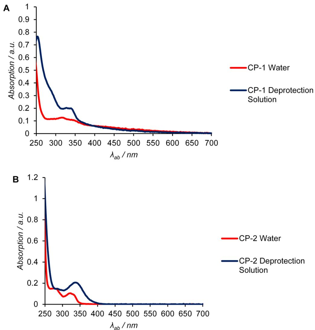
**Figure S2.** UV-Vis Spectra of A) **CP-1** and B) **CP-2**. Compounds were dissolved at  $0.1 \text{ mgmL}^{-1}$  in either water or deprotection buffer (2:1:1, v:v:v, methanol:water:saturated  $\text{NaHCO}_3$ ) for 30 minutes prior to measurement of spectra.
