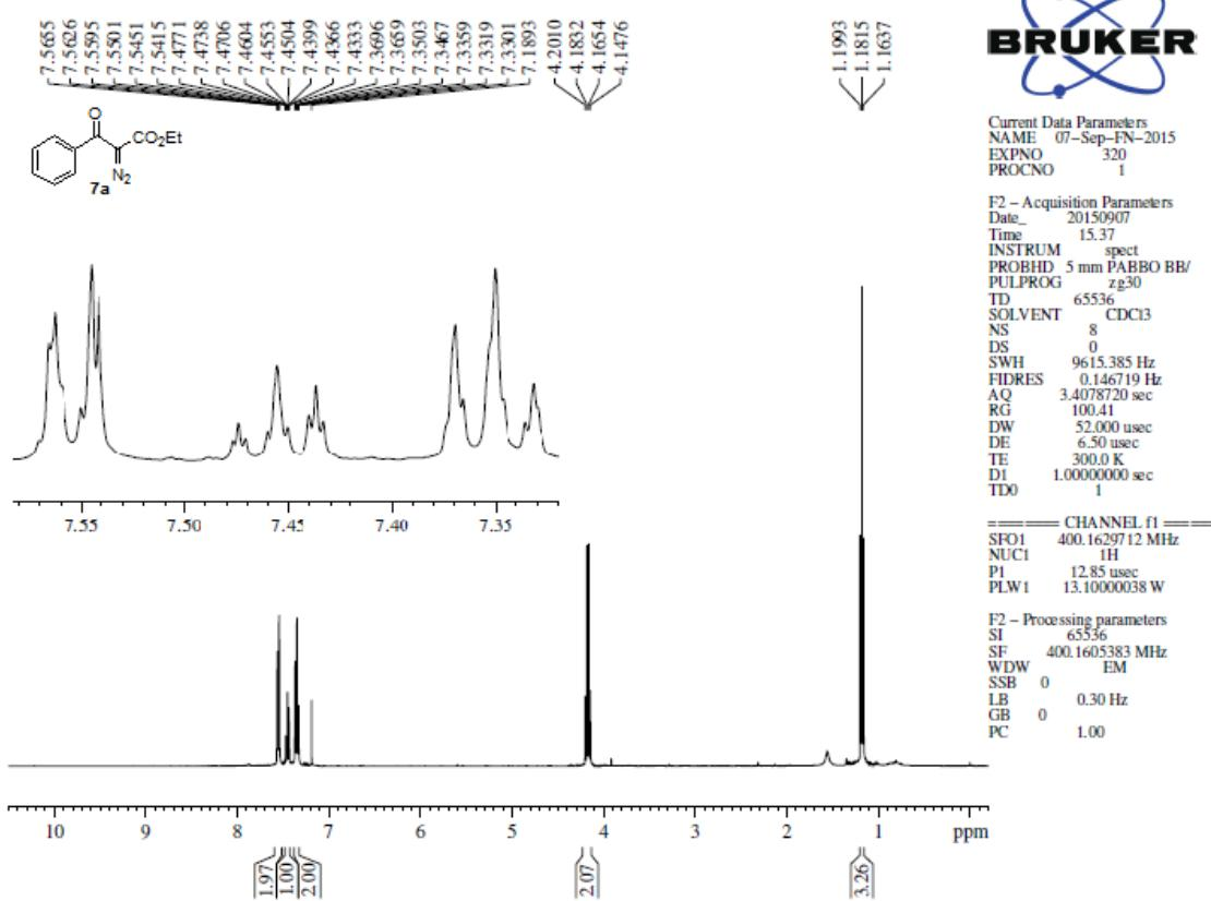
Figure 72: <sup>1</sup>H NMR spectrum of 7a
