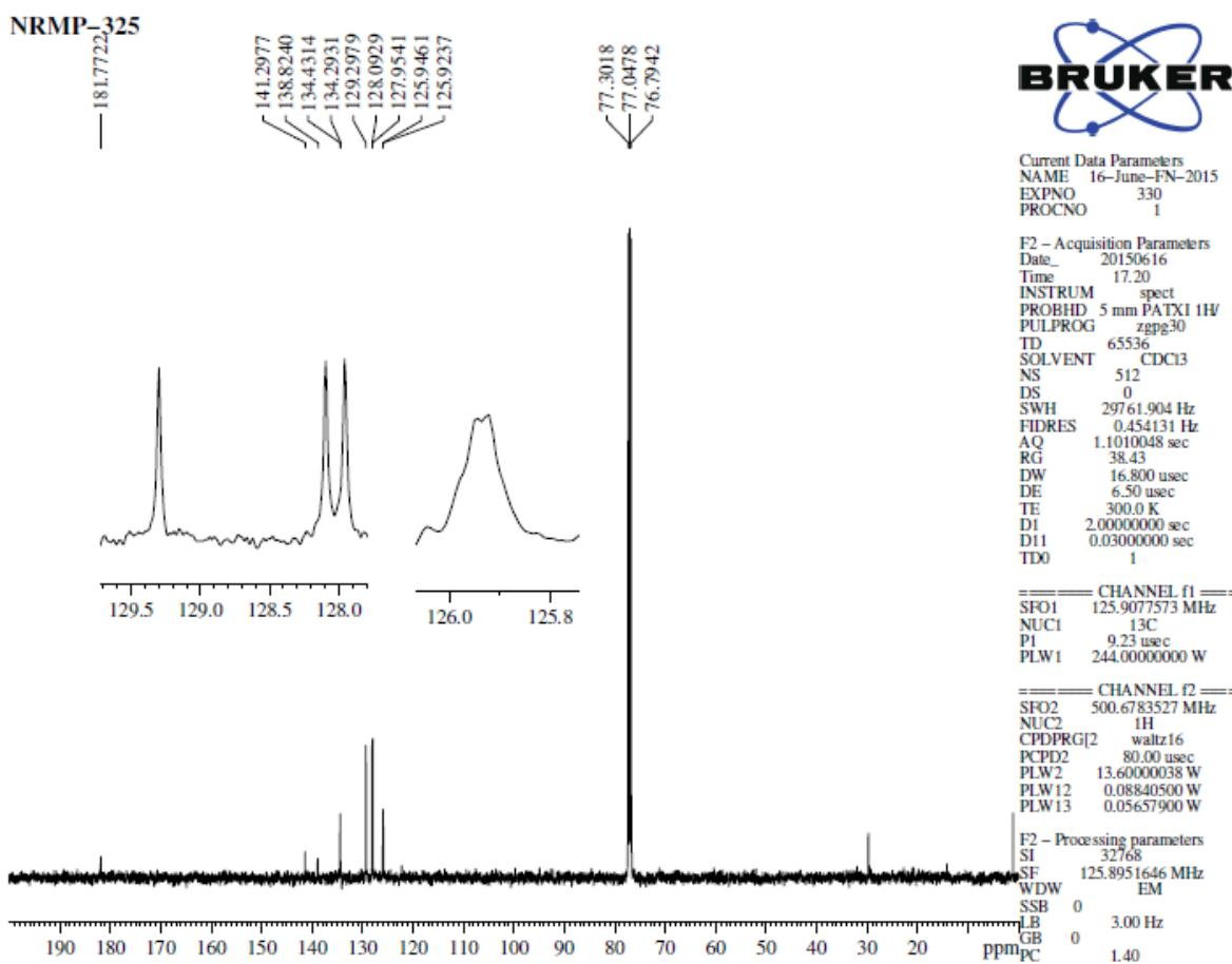
Figure 63:  $^{13}\text{C}$  NMR spectrum of **5h**
