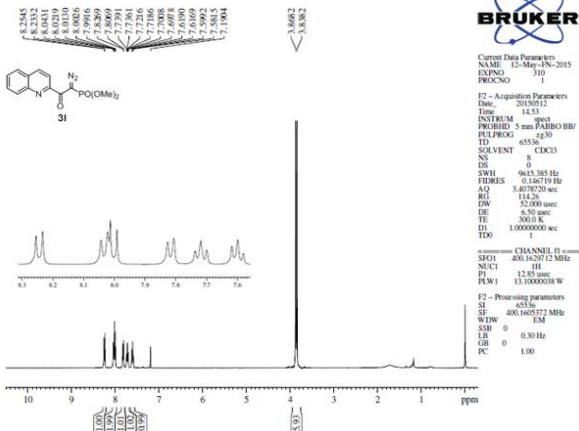
Figure 38: <sup>1</sup>H NMR spectrum of 3l
