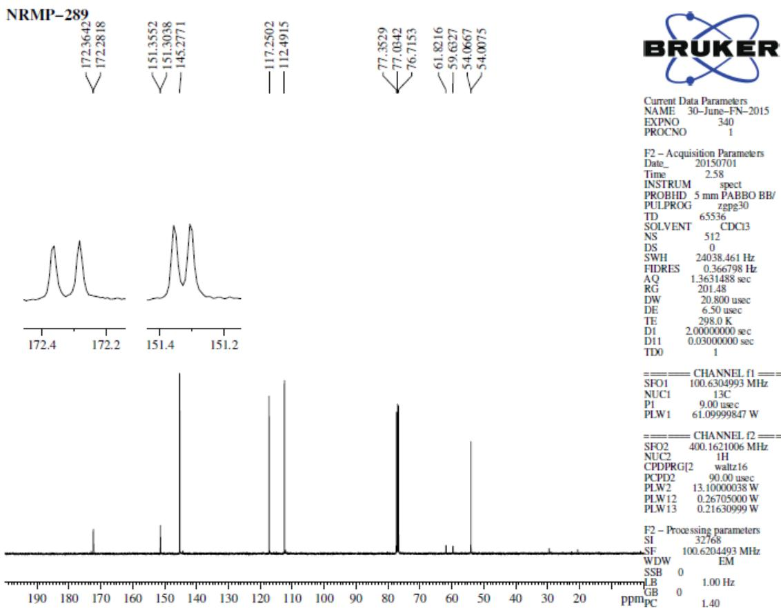
Figure 33:  $^{13}\text{C}$  NMR spectrum of 3j
