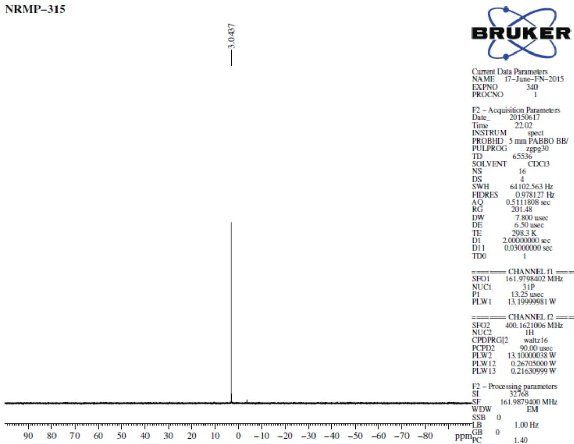
Figure 85: <sup>31</sup>P NMR spectrum of 9c
