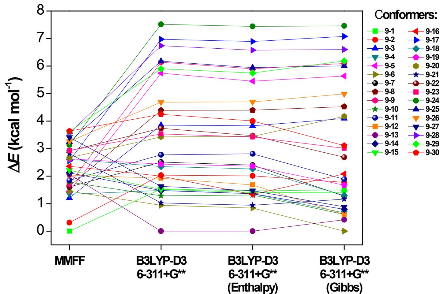
**Figure S3:** Compound **9** conformer relative energies for the 30 lowest energy minima (from 9714 conformers found in the MM calculations in the gas phase) obtained at different theoretical levels. MMFF and B3LYP/6-311+G\*\* energies correspond to optimised geometries on the same levels, respectively. B3LYP/6-311+G\*\* corrected energies with enthalpies and Gibbs free energies were obtained from B3LYP/6-311+G\*\* frequency calculations.
