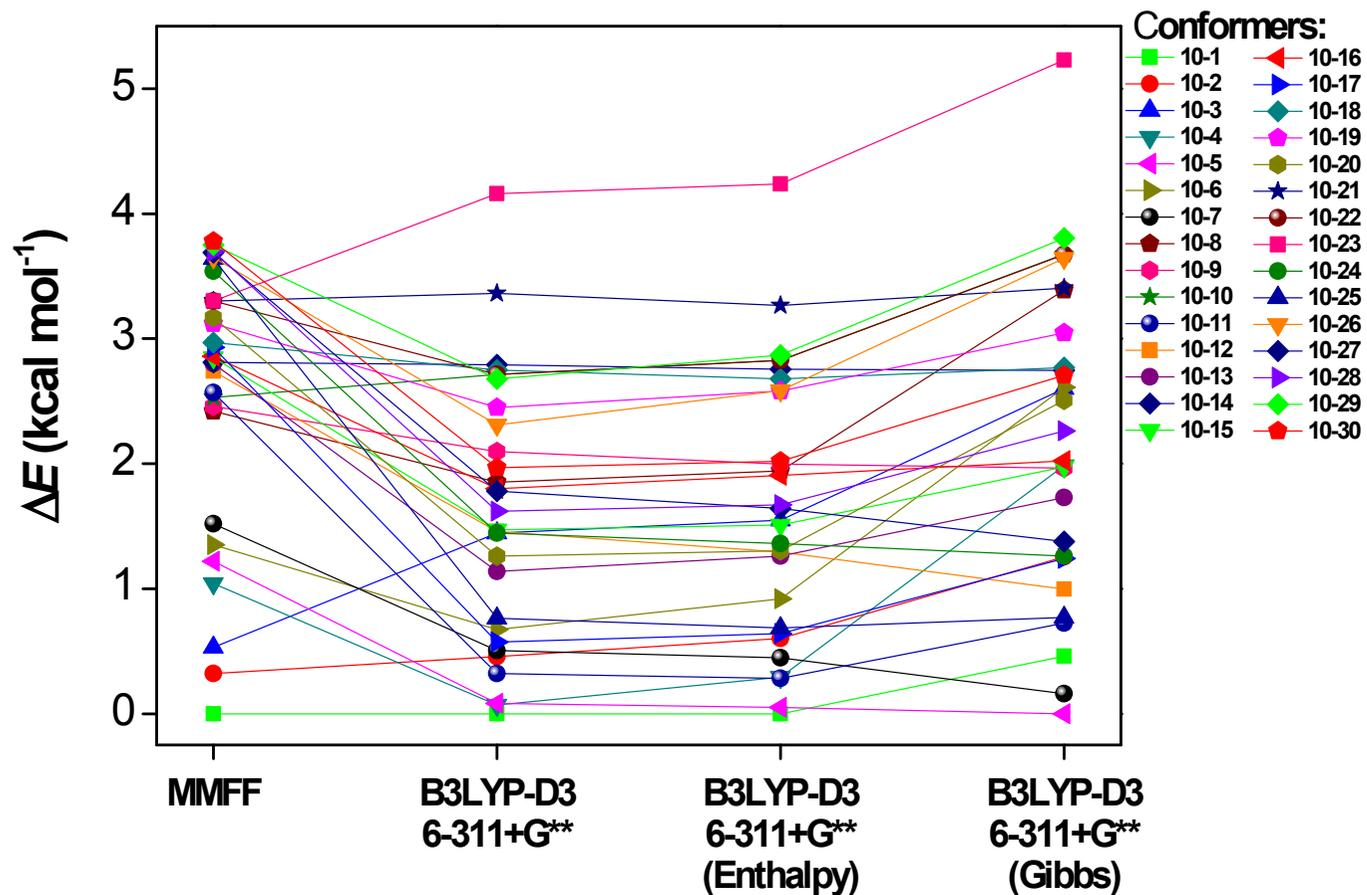
**Figure S2:** Compound 10 conformer relative energies for the 30 lowest energy minima (from 7948 conformers found in the MM calculations in the gas phase) obtained at different theoretical levels. MMFF and B3LYP/6-311+G\*\* energies correspond to optimised geometries on the same levels, respectively. B3LYP/6-311+G\*\* corrected energies with enthalpies and Gibbs free energies were obtained from B3LYP/6-311+G\*\* frequency calculations.
