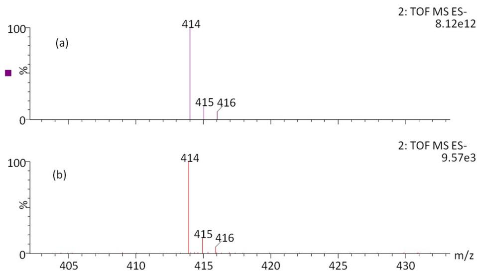
**Figure S28.** (a) The isotopic pattern of the signal at  $m/z$  414 as compared to (b) the theoretical isotopic pattern of  $C_{11}H_{18}N_2O_{11}PS$ . Negative mode ESI mass spectrum acquired on the Waters LCT Q-TOF.
