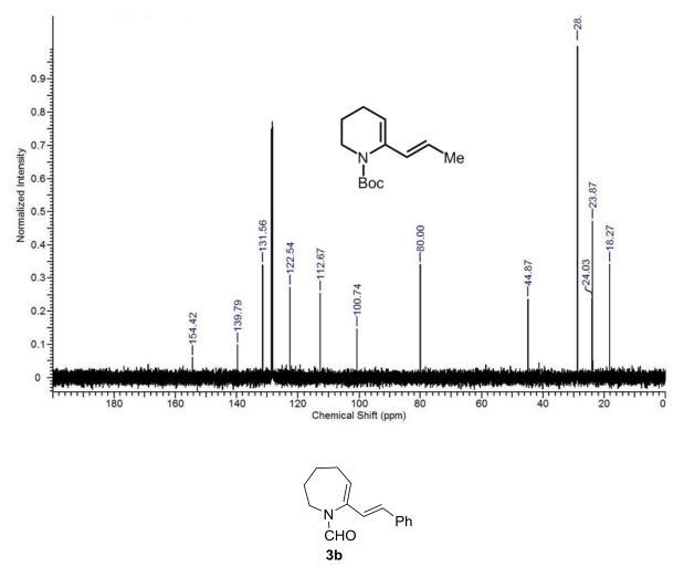
Prepared from **1f** (125 mg, 1 mmol) and β-styrenylboronic acid (2 equiv) using **Procedure A**. Time = 32 h. Purification: Flash chromatography on silica (pretreated with 1% Et<sub>3</sub>N) eluting with hexane/EtOAc (90:10). Yield = 136 mg, 60%. Data as previously reported by us.<sup>4</sup>
