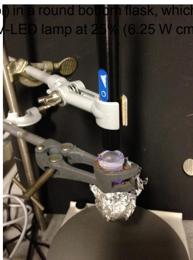
**Figure 1.** Setup for the photocyclisation of azides.
