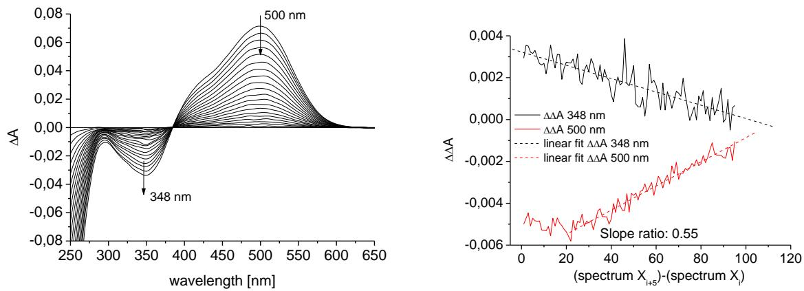
Fig. S10: Detergent effect on the stability of 13dm-assembled rhodopsin in the dark: left, 13dm-rhodopsin in DDM and LDAO (3%) without addition of hydroxylamine, immediate and after 90 min (strong loss of chromophore); right, stability of 13dm-rhodopsin against hydroxylamine in the dark over 3 h (no change).
