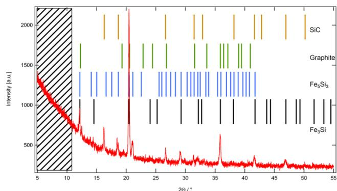
**Fig. 18** X-ray diffraction (XRD) pattern of ceramic material obtained by ceramization of VFc@PMSB1 under inert conditions showing a mixture of  $\text{Fe}_3\text{Si}_5$ ,  $\text{Fe}_3\text{Si}$ , SiC, and graphite.
