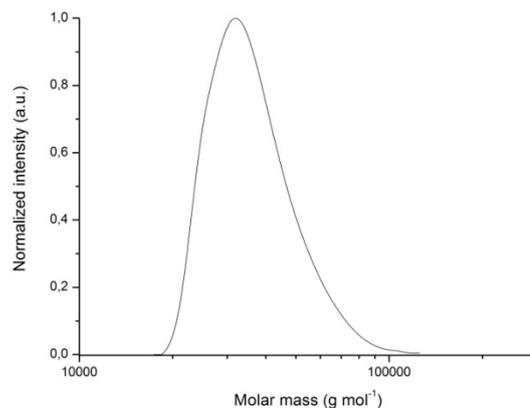
**Fig. S13** Molar mass distribution of VADN@PS-*b*-PMSB1 (THF, measurement vs. PS standards).
