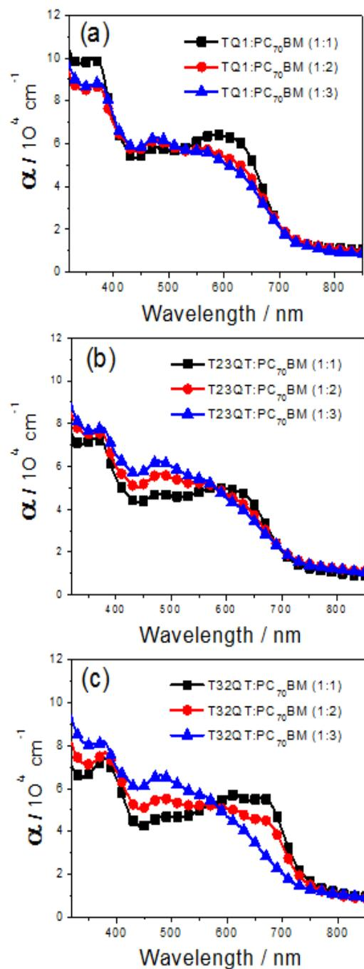
**Figure S4.** Thin film absorption spectra of (a) TQ1:PC<sub>70</sub>BM, (b) T23TQ:PC<sub>70</sub>BM and (c) T32TQ:PC<sub>70</sub>BM in three different composition ratio (1:1, 1:2 and 1:3).
