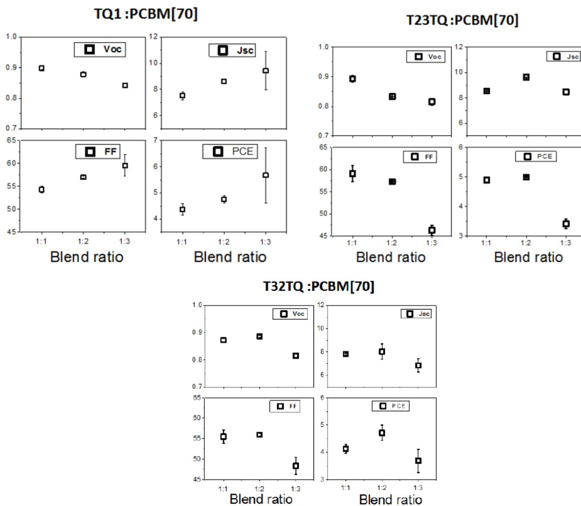
**Figure S8.** The basic figures of merit (V<sub>oc</sub>, J<sub>sc</sub>, FF and PCE) for the polymer:PC<sub>70</sub>BM OPV devices as a function of the polymer:PC<sub>70</sub>BM composition ratio (1:1, 1:2 and 1:3).
