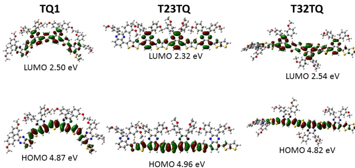
**Figure S6.** DFT [B3LYP/6-31G(d,p)] calculated frontier molecular orbitals of the HOMO (bottom) and LUMO (top) for the tetramers of TQ1, T23TQ and T32TQ.
