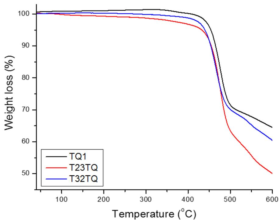
**Figure S2.** Thermogravimetric analysis graphs of the TQ1, T23TQ and T32TQ under a nitrogen atmosphere.
