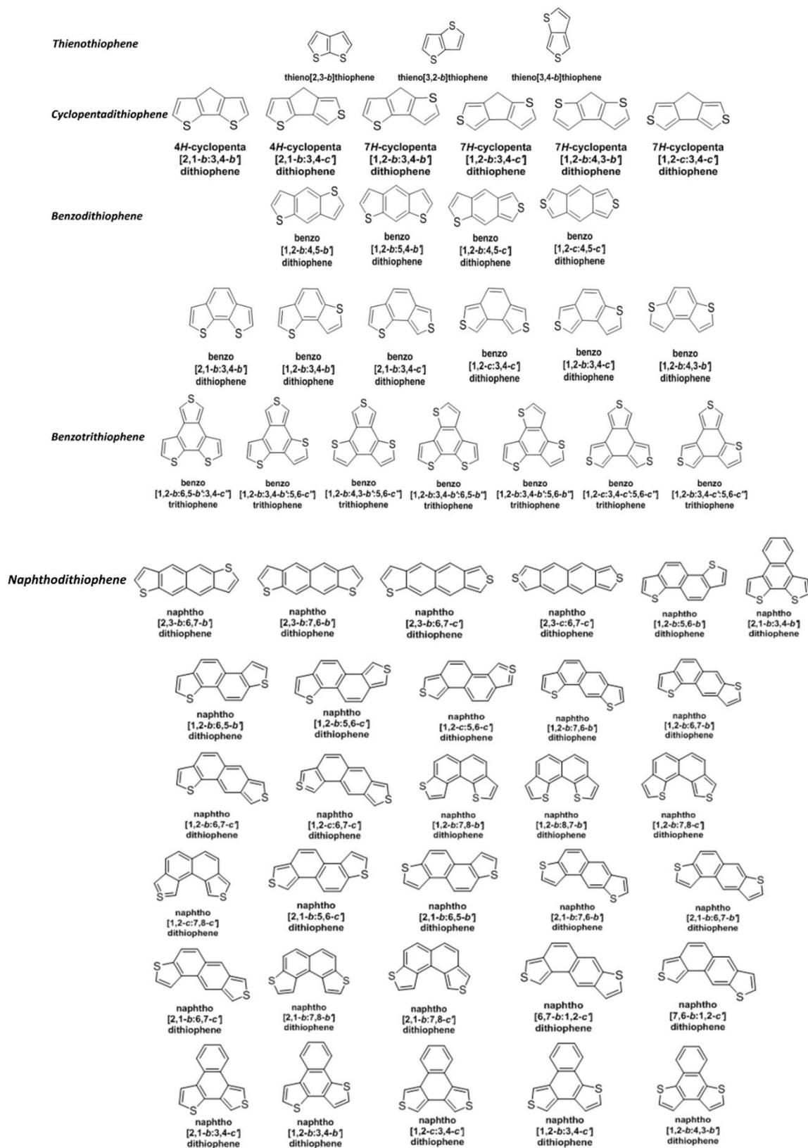
**Figure S1.** Isomeric structures of the most common electron rich building blocks for the synthesis of D-A conjugated polymers.
