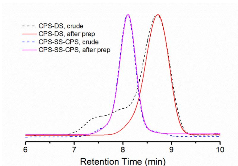
**Figure S4.** SEC RI traces of CPS-DS (crude, black dotted curve; purified by preparative SEC, red solid curve, yield: 75%), CPS-SS-CPS (crude, blue dotted curve; purified by preparative SEC, pink solid curve, yield: 95%). SEC analysis was based on the polystyrene calibration curve. All SEC traces were normalized to height.
