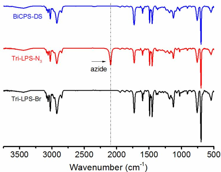
**Figure S6.** FT-IR spectra of Tri-LPS-Br (black curve), Tri-LPS-N<sub>3</sub> (red curve), BiCPS-DS (blue curve).
