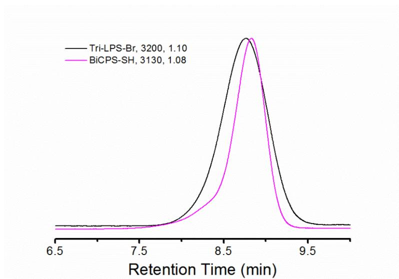
**Figure S5.** SEC RI traces of Tri-LPS-Br ( $M_p = 3310$ ), BiCPS-SH ( $M_p = 2980$ ). THF was used as the eluent, and PS standards were used for the calibration. All SEC traces were normalized to height.
