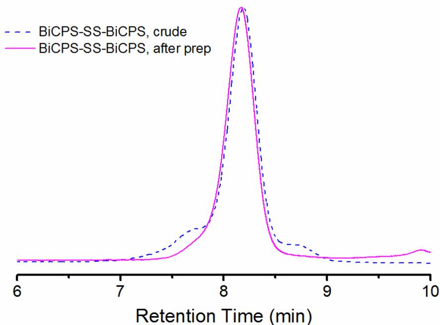
**Figure S8.** SEC RI traces of BiCPS-SS-BiCPS (crude, blue dotted curve; purified by preparative SEC, pink solid curve, yield: 90%). SEC analysis was based on the polystyrene calibration curve. All SEC traces were normalized to height.
