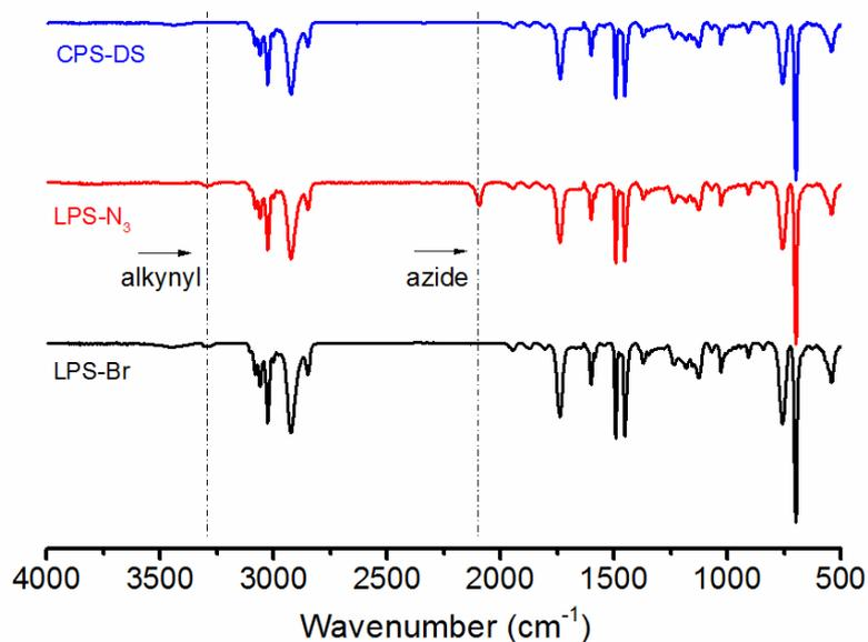
**Figure S3.** FT-IR spectra of LPS-Br (black curve), LPS-N<sub>3</sub> (red curve), CPS-DS (blue curve).
