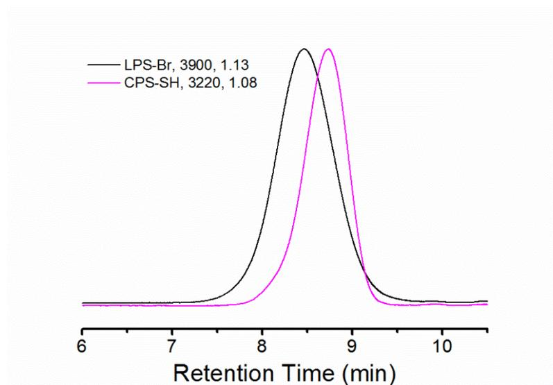
**Figure S2.** SEC RI traces of LPS-Br ( $M_p = 4290$ ), CPS-SH ( $M_p = 3190$ ). THF was used as the eluent, and PS standards were used for the calibration. All SEC traces were normalized to height.
